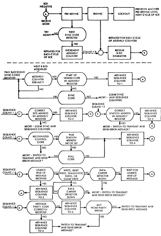
• ERROR MESSAGE SENT ONLY IF ERROR MESSAGE ENABLE/DISABLE SWITCH IS IN ENABLE POSITION. OTHERWISE, NO RESPONSE IS GIVEN.
