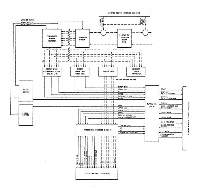
Typewriter Adapter Block Diagram
