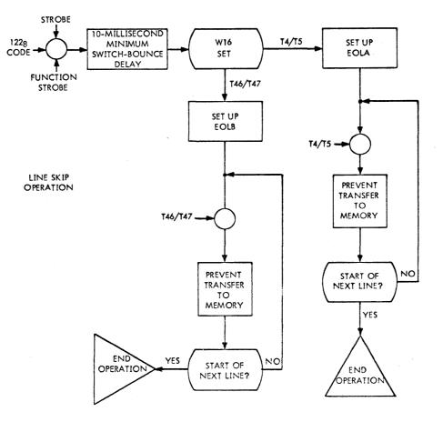
is display of the carriage return symbol () at the original entry marker position while remaining data in the line is erased. The marker subsequently references the first symbol position in the next line.
