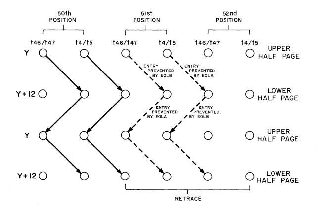
To briefly summarize, the end of line conditions for any half page and any page format prevent the possibility of data entry into memory when the entry position shifts into the retrace period at t4/t5.
