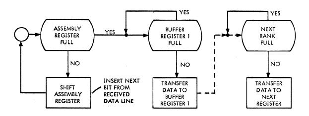
The contents of the assembly register are examined for parity errors and escape codes (these two codes require extra consideration). In addition, a BCD conversion is made. If the assembled word has a parity error and is part of the data subset, an octal code of 76 is entered in buffer register 1, and subsequently, display buffer memory. This results in display of the parity error symbol ( $\blacksquare$ ) for the particular code in error.
