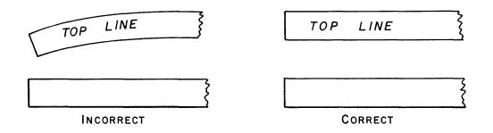
Squaring of the raster is accomplished by the horizontal ramp generator. To correctly adjust this circuit:
