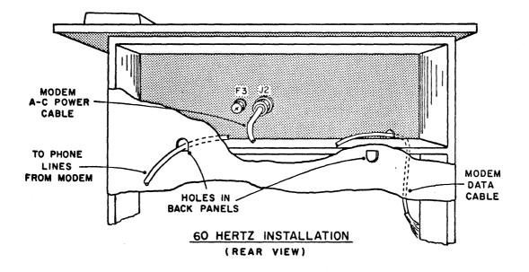
J2 is not used in 50-hertz installations. In this case, the modem power cable must be connected to terminal strip TB3 as shown in the next illustration. The terminal strip is on the front side of the panel so the cable must be routed through one of the holes.
