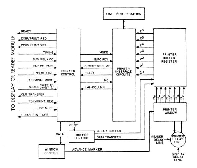
Line Printer Adapter Block Diagram
