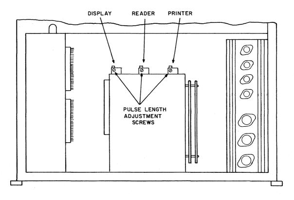
Figure 6-2. Delay Lines (Front Panel Removed)
