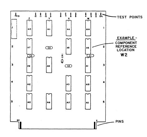
Figure 6-1. Typical Board Assembly
