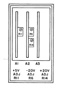
Figure 6-4. Power Supply Adjustments
