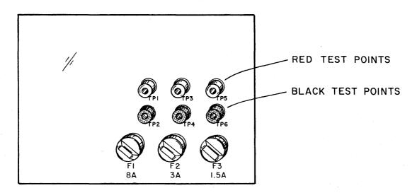
Figure 6-5. Power Supply Test Points
