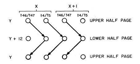
The delay-line skew and extra symbol count create the need for a pair of end of line conditions. A 50 by 20 format is again assumed in the following illustration to point out these conditions. The 51st symbol position marks the beginning of the retrace period during which display must be prevented. Data entry at t4/t5 of the 50th symbol position is possible in upper half page even though the delay-line Section IV 217 Theory of Operation Basic Configuration
