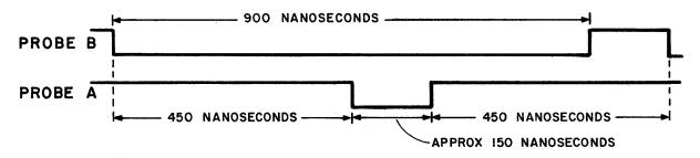
Figure 6-3. Delay-Line Adjustment Waveforms
