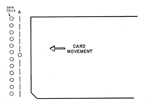
Since the card does not cover any of the data cells at this time, all cells should indicate a light condition. The controller samples the Data lines to provide this check. If a light condition does not exist in all cells, an error is evident. In any event, the adapter issues an Escapement Drive signal and card movement continues, with each column being read by the data cells.
