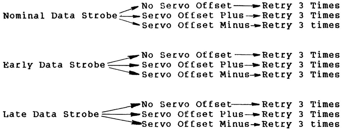
FIGURE 20. POSSIBLE DATA STROBE AND SERVO OFFSET COMBINATIONS USED BY THE SCSI WREN DURING READ RETRY
