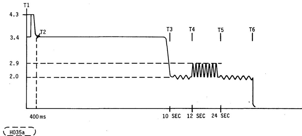
FIGURE 4. TYPICAL +12 V CURRENT PROFILE
