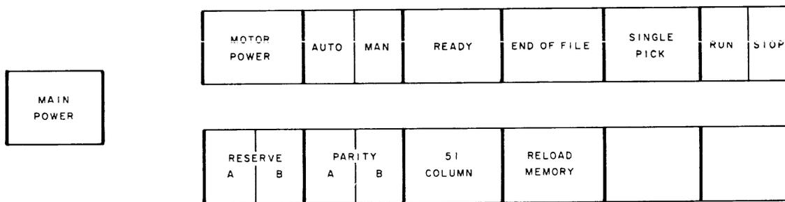
Figure 3. 3649 Card Reader Switches and Indicators
