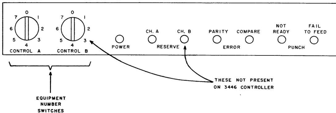
Figure 2. Controller Switches and Indicators
