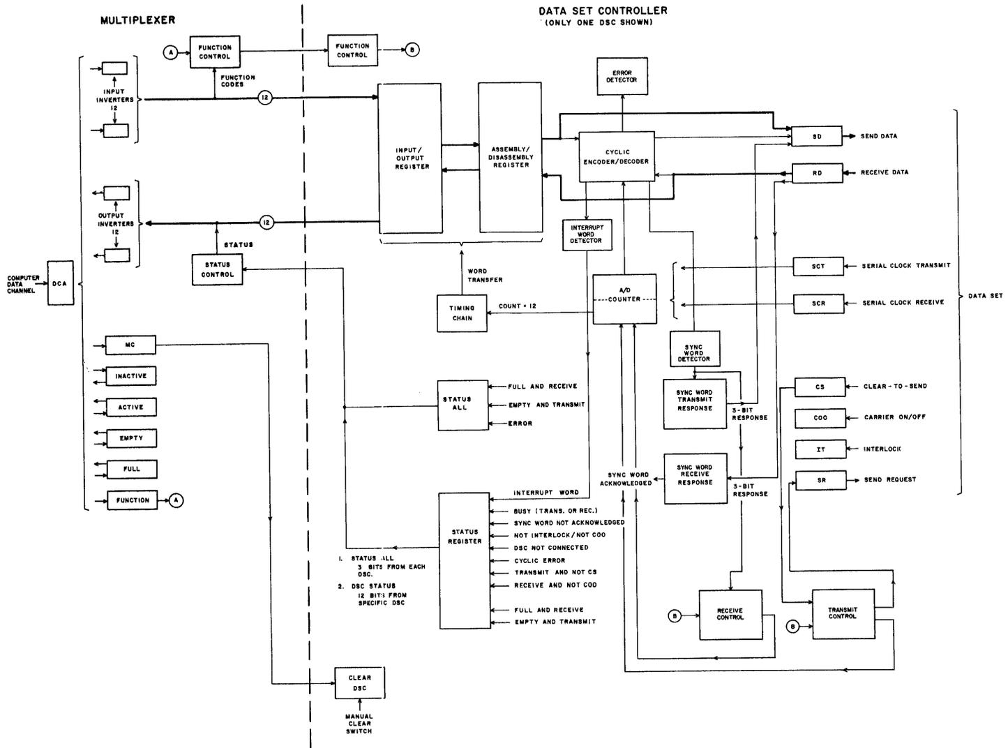
Figure 2. 6673/6674 Block Diagram
