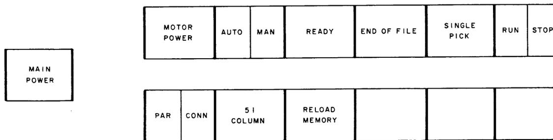
Figure 4. 3447 Card Reader Switches and Indicators
