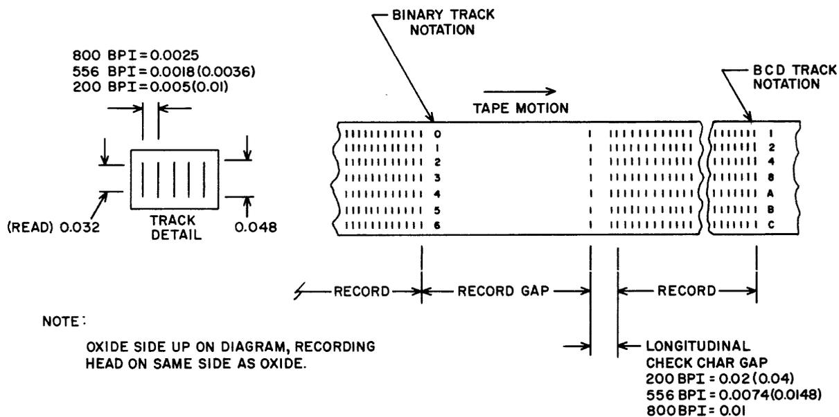
Figure 2. Bit Assignments on Tape
