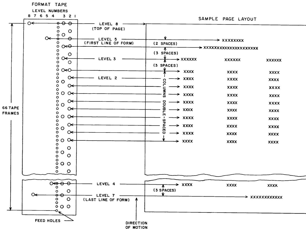
Figure 3. Spacing Example
