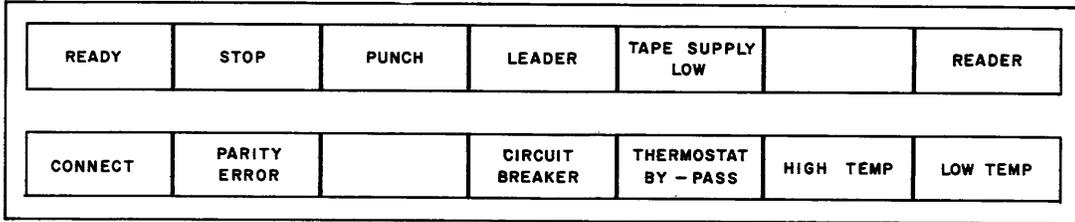
Figure 2. 3691-B Switch and Indicator Panel
