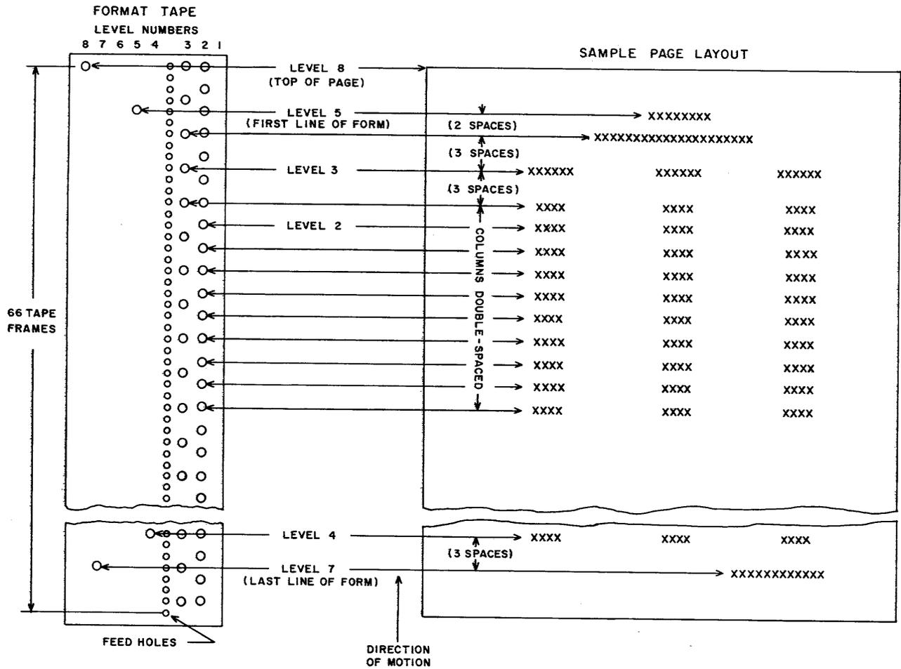
Figure 5. Spacing Example
