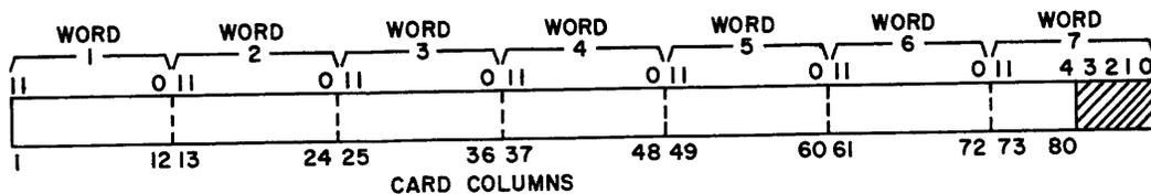
Figure 2. Punch Register in the 170 Controller
