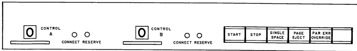
Figure 2. 3659 Controller Switch and Indicator Panel
