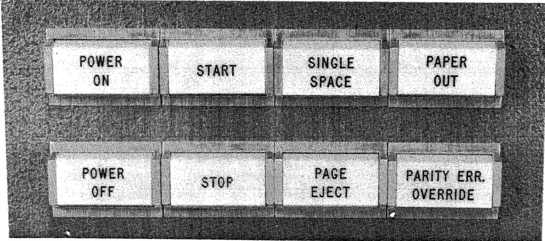
Figure 3. 501/505 Switch and Indicator Panel
