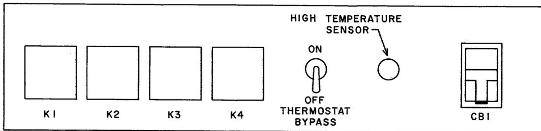
Figure 8. Operator Control Panel
