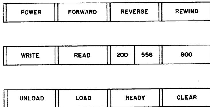
Figure 5. 604/607 Operator's Control Panel
