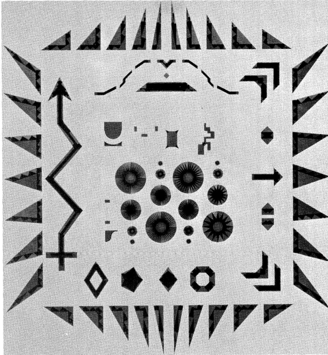
These complex shapes, shown in this enlargement of a test pattern plotted on an Electromask Pattern Generator, demonstrate the highly sophisticated nature of CALMA's pattern generator software. The reticle was underdeveloped to illustrate how each shape has been fractured into a set of rectangles acceptable to the pattern generator.
