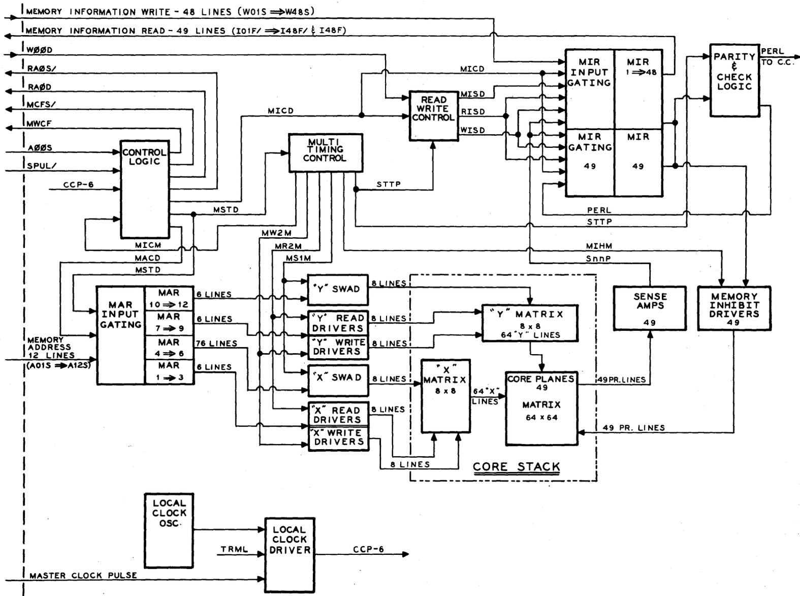
1. Control Logic - Controls all Memory functions which depend upon the System Clock. It also develops the Control levels that go to Central Control.
