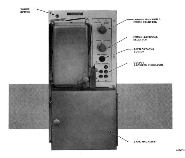
Figure 7. Tape Punch Assembly
