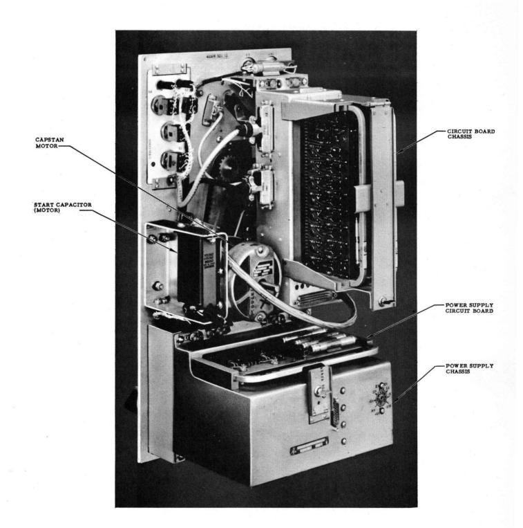
Figure 36. Photoelectric Tape Reader, Rear
