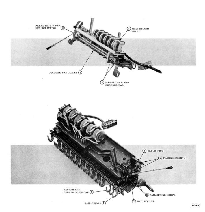
Figure 29. Decoder Lubrication Points
