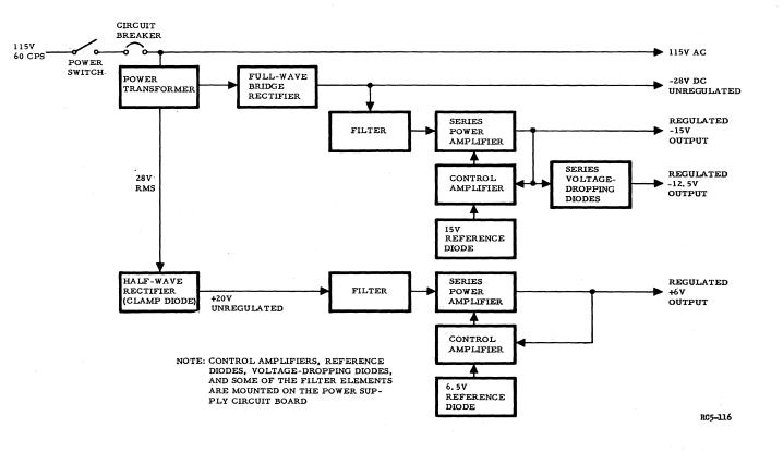
Figure 51. Tape Punch Power Supply (Block Diagram)
