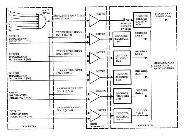
Figure 22. Typewriter-Decoding Block Diagram
