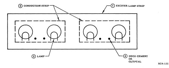
Figure 42. Photoreader Exciter Lamp Strip
