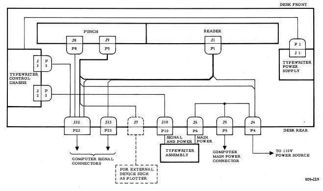
Figure 9. Desk Interconnection Block Diagram
