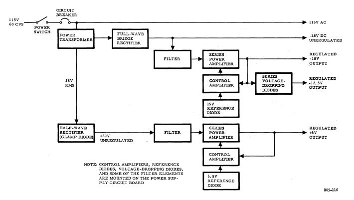
Figure 28. Typewriter Power Supply, Block Diagram
