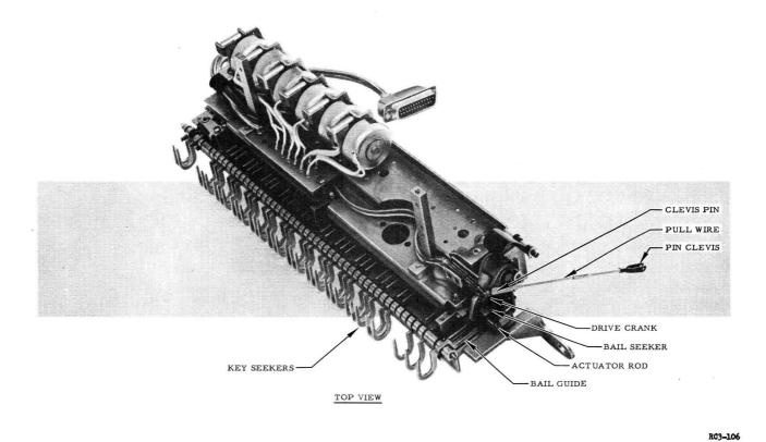
Figure 23. Decoder Assembly
