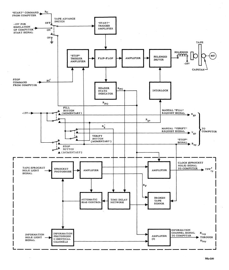
Figure 37. Photoelectric Tape Reader, Block Diagram
