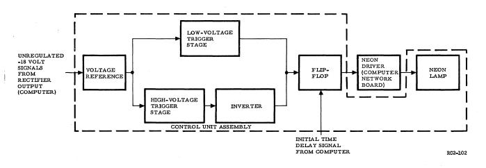
Figure 14. Voltage Transient Trigger Diagram
