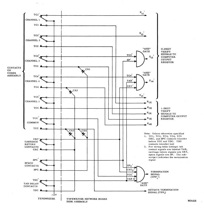
Figure 25. Typewriter Coding, Simplified Diagram
