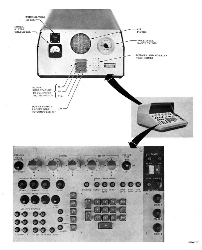
Figure 10. Control Console, Front and Rear Views
