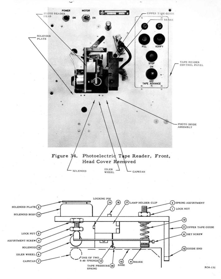
Figure 35. Photoelectric Tape Reader, Canister, Cover Removed photoreader front panel over two dowel pins. When the canister is mounted, a 90-degree manual turn of the locking handle locks the canister in place, releases the tape from magazine clips, and secures it in the reader head (see figure 6).
