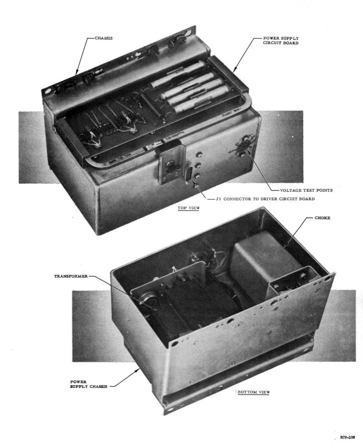
Figure 27. Typewriter Power Supply
