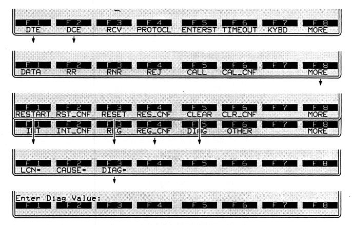
Figure 34-16 These four packet types (plus *Diagnostic*) allow you to enter a diagnostic-code value as a spreadsheet condition.
