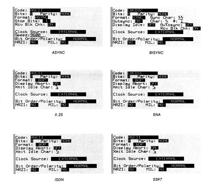
Figure 4-7 Sample Line Setup configurations for the following protocols: X.25, SNA, ASYNC, BISYNC, ISDN, and SS#7.
