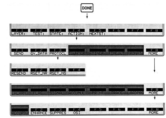
Figure 33-19 Action softkeys specific to X.25 Layer 2.
