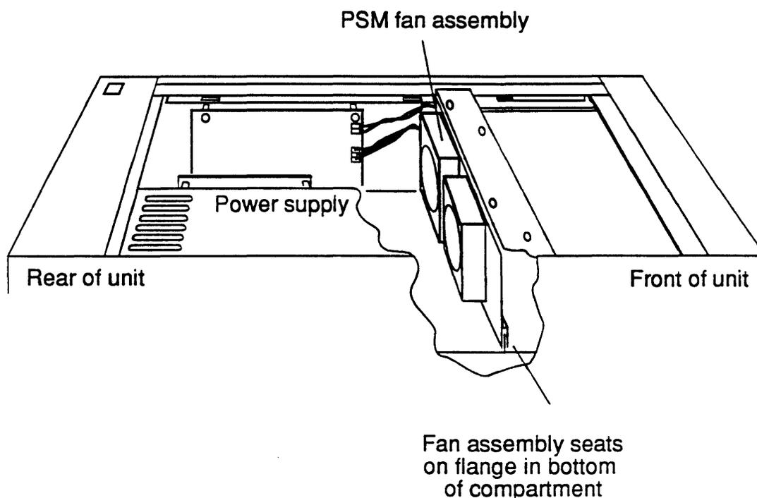
**Figure 6-8. PSM Fan Assembly Access**
