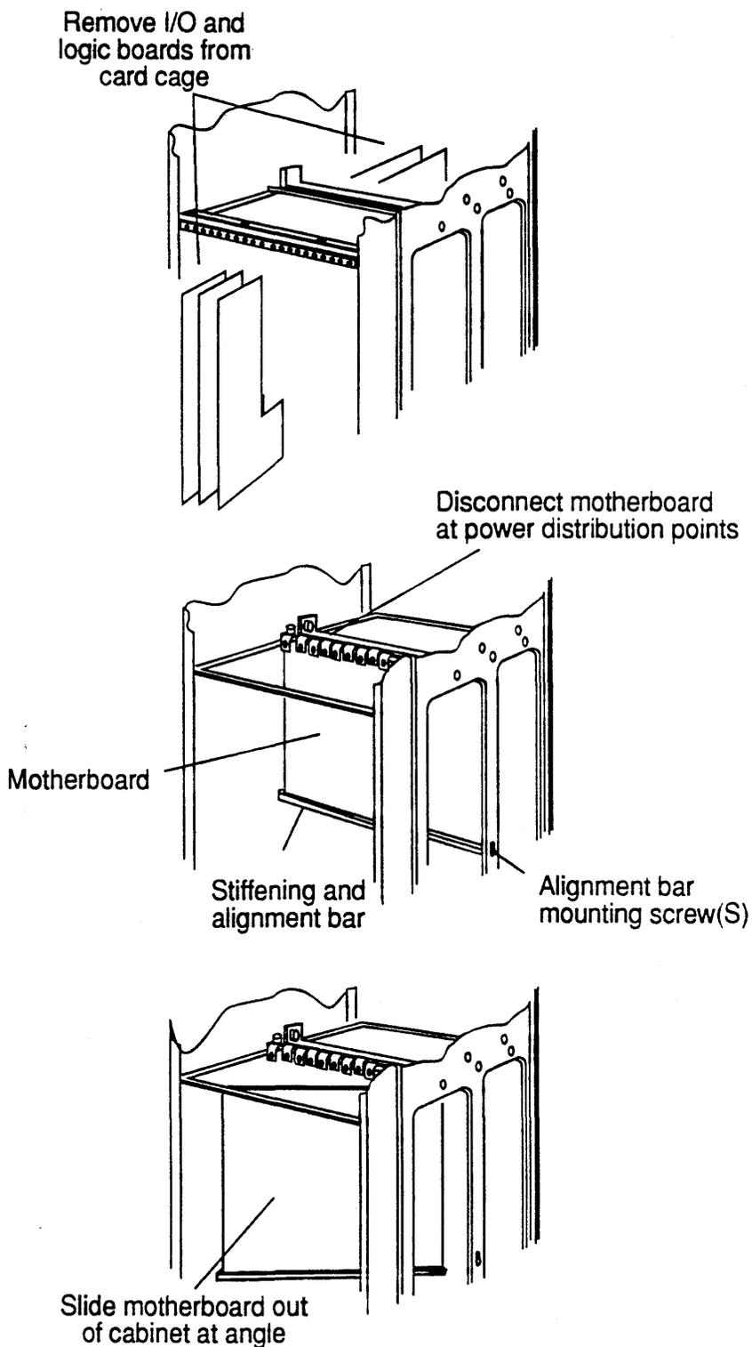
**Figure 3-24. Motherboard Access and Removal, Part 2**
