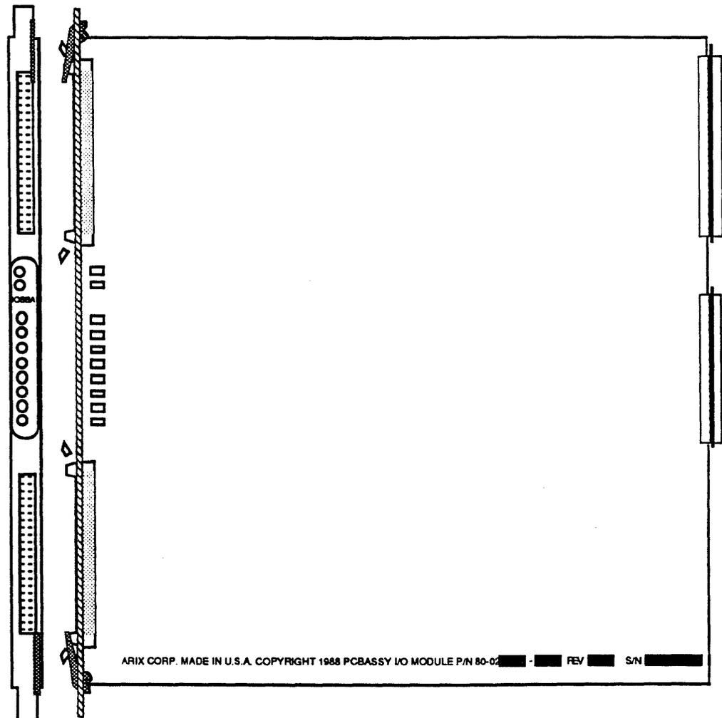
**Figure 3-10. I/O System Bus Adapter**
