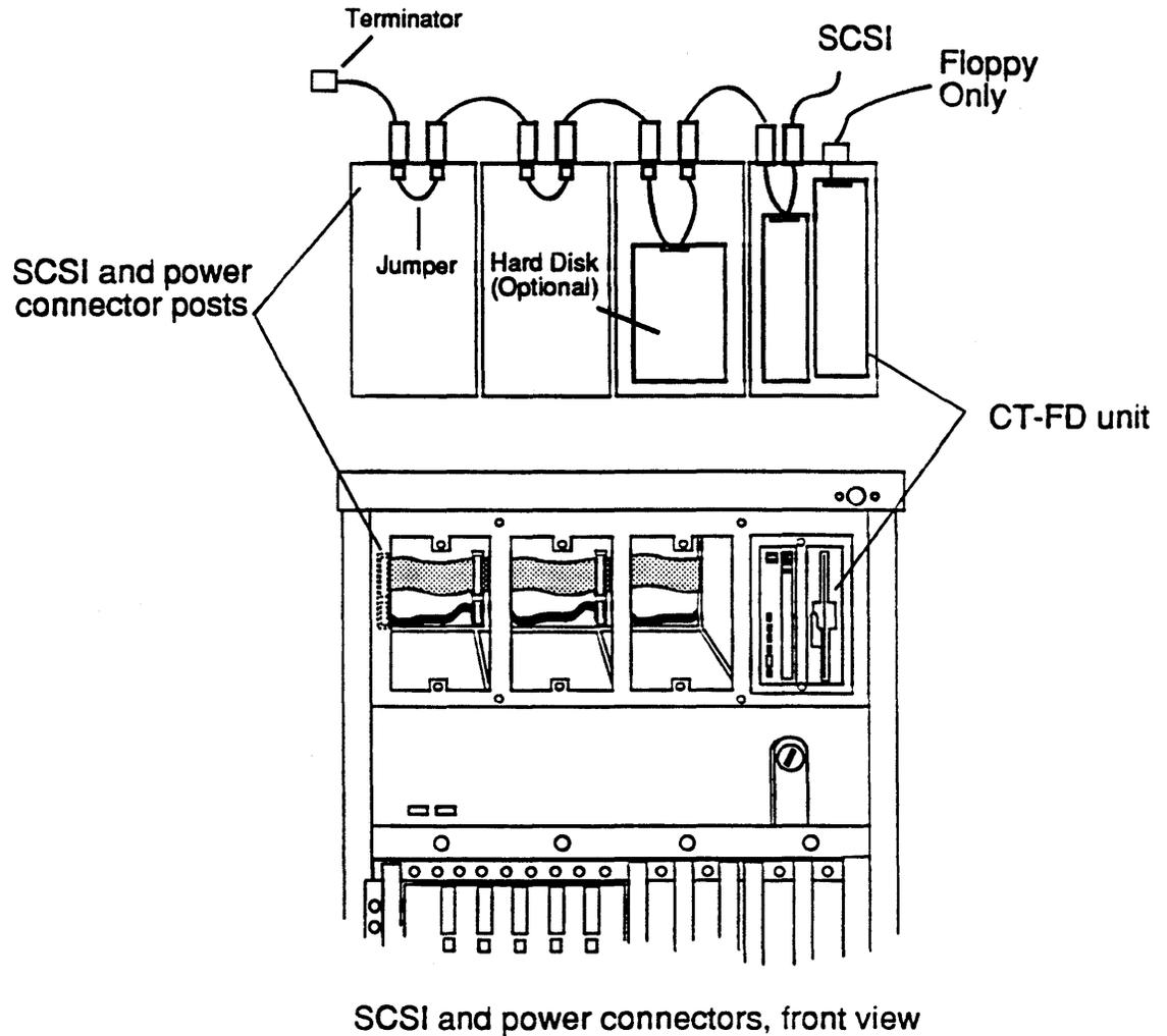
**Figure 5-2. SCSI Device Connectors, RMM Module**
