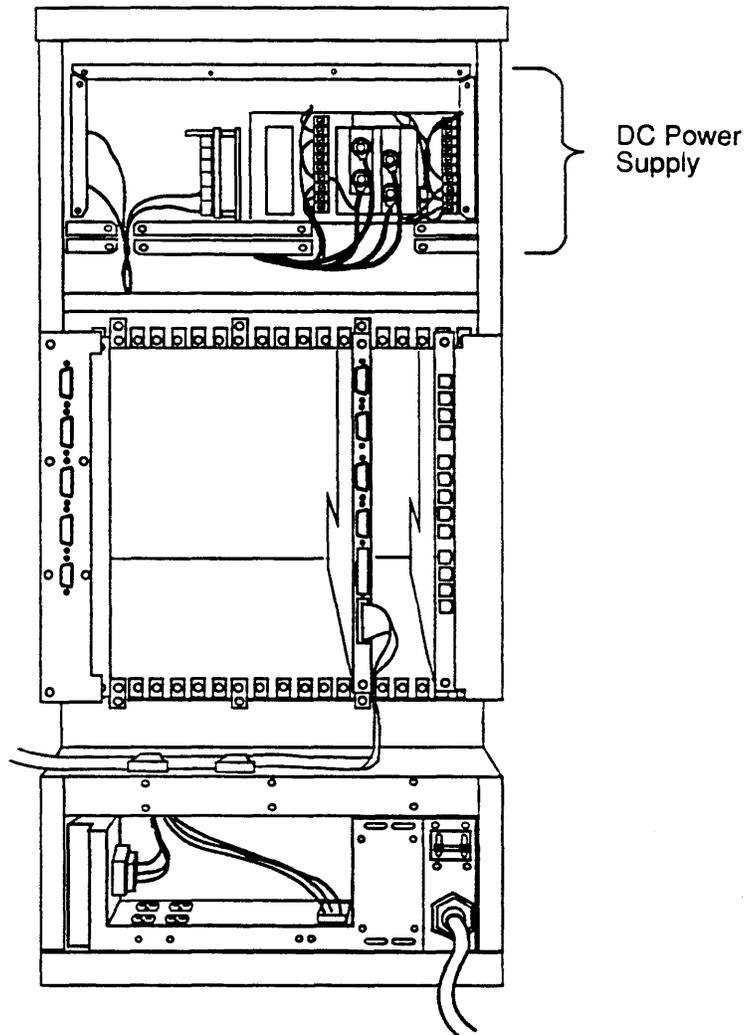
Figure 7-1. DC Power Supply Location in Cabinet
