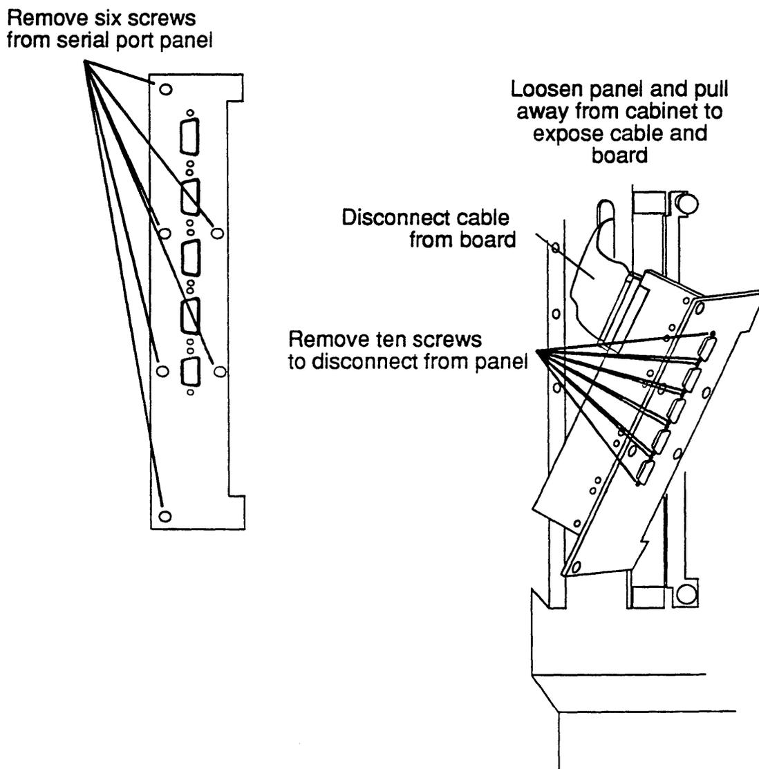
**Figure 3-19. System Console Board Access**
