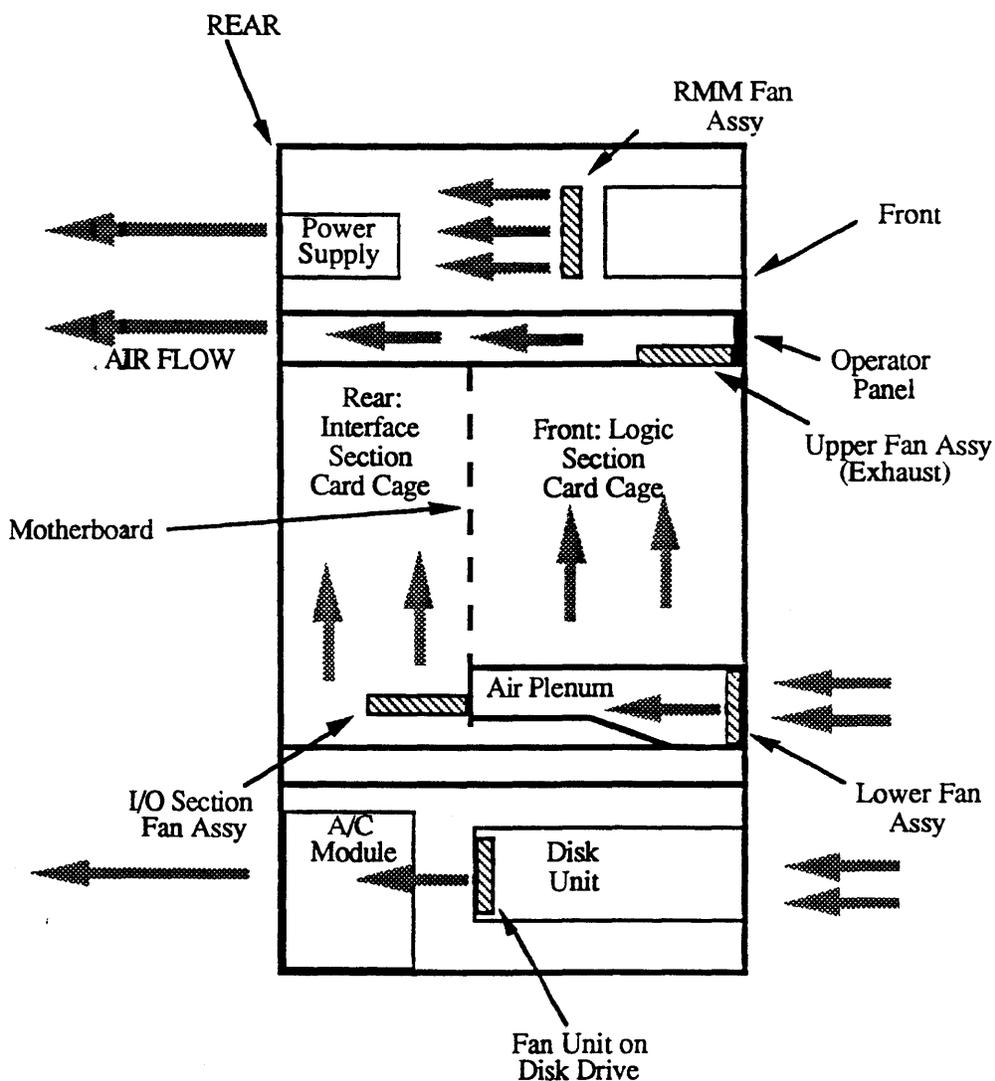
Figure 6-1. Primary Cabinet Cooling System, Air Flow
