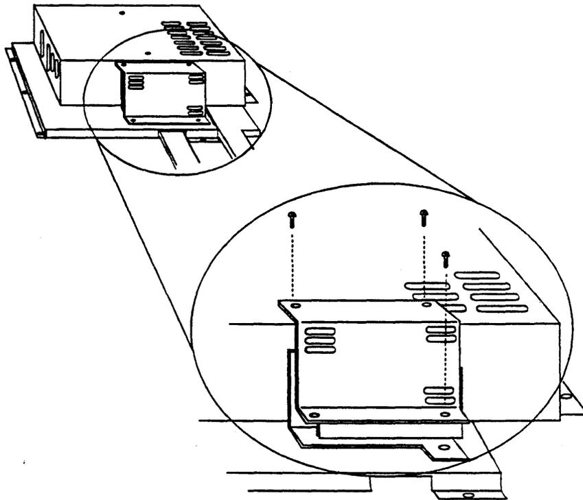
**Figure 4-4. Auxiliary Power Supply Board Access**
