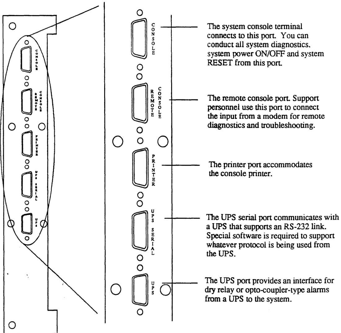
**Figure 1-6. System Serial Ports**
