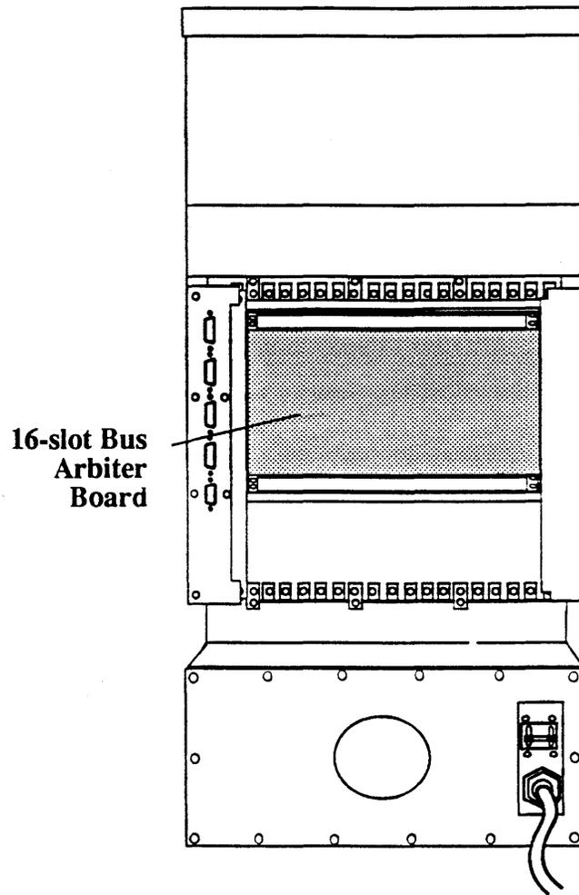
**Figure 3-21. Bus Arbiter Board Access**
