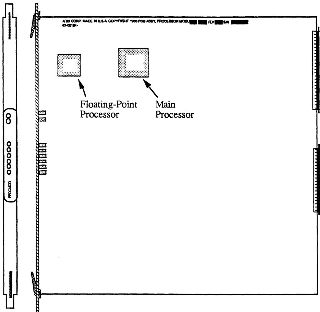
Figure 3-7. Processor Module
