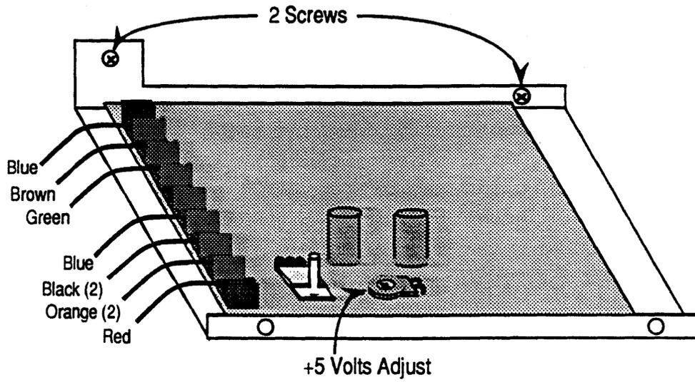
**Figure 4-3. Auxiliary Power Supply Board**
