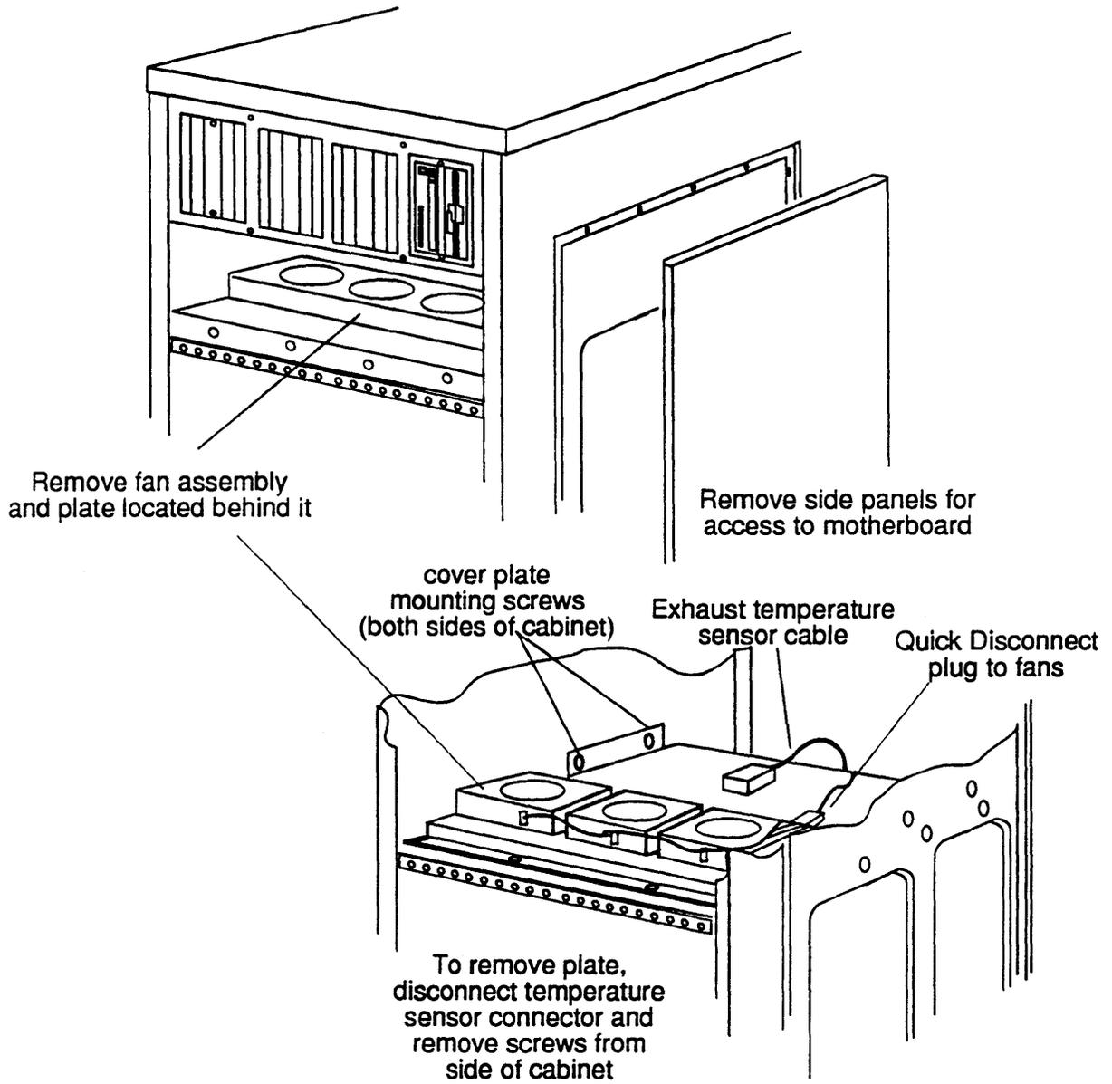
**Figure 3-23. Motherboard Access and Removal, Part 1**
