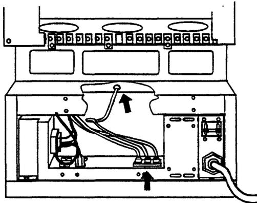
Disconnect temperature sensor cable from AC module and rear fan panel
