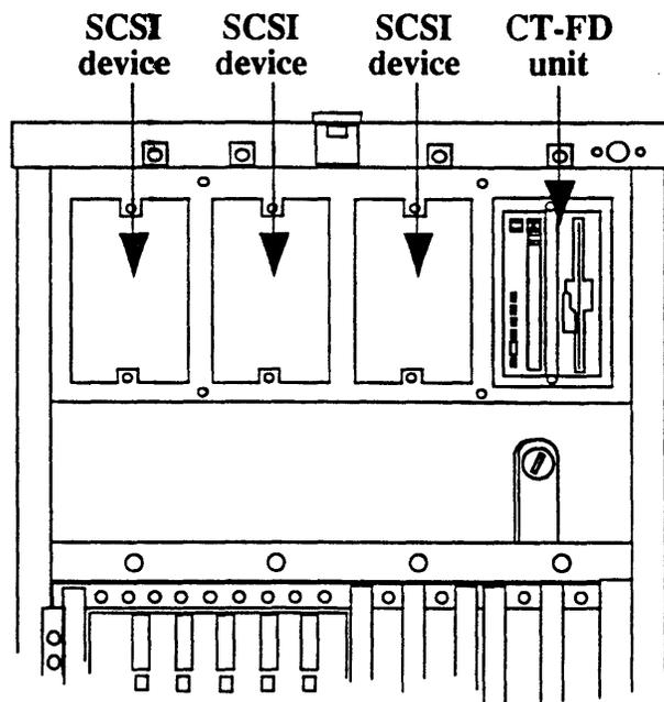
**Figure 5-1. RMM with Access Panels Removed**
