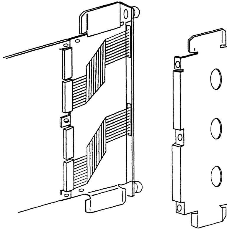
**Figure 3-3. DSDB Bracket and Plastic Shield.**
