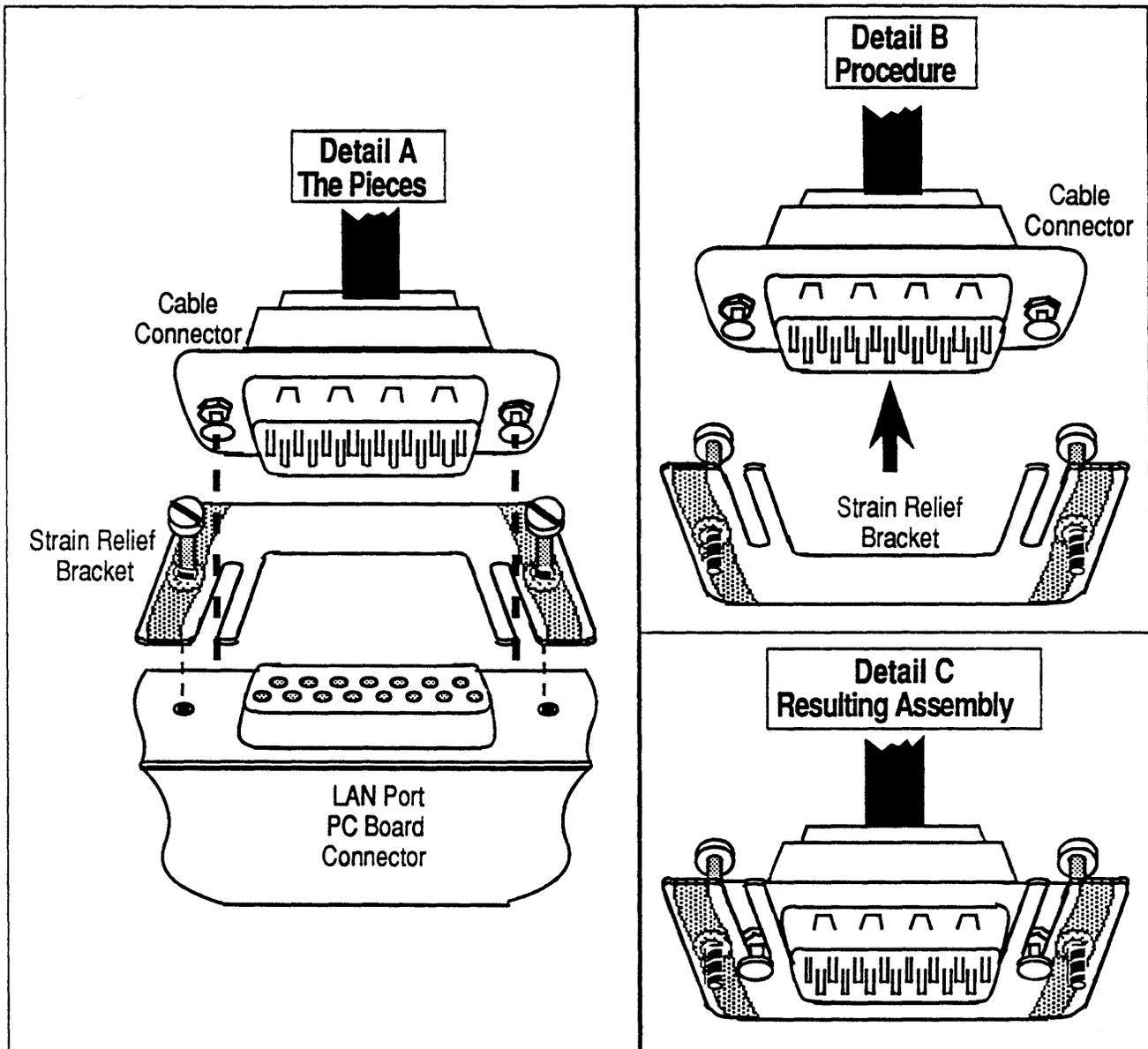
Figure 3-16. Connector Hardware and AUI Cable Configuration.
