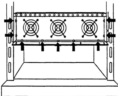
Remove nine mounting screws from front of unit
