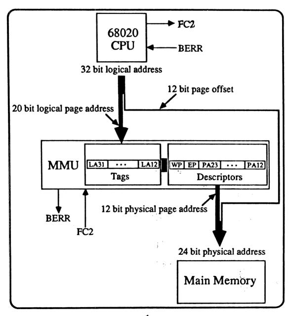
If the upper 20 bits of the logical address are contained in any of the 64 entries in the MMU, the upper 12 bits of the physical address are provided within 65ns. This permits the MMU to function without wait states. If the page is resident in the MMU, the access control bits associated with that page are also checked to see if write protection and or execute only protection is in effect.
