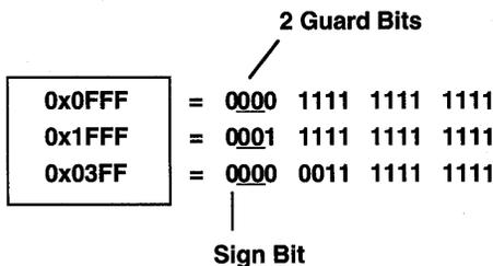
Figure C.5 Block Floating-Point Adjustment
