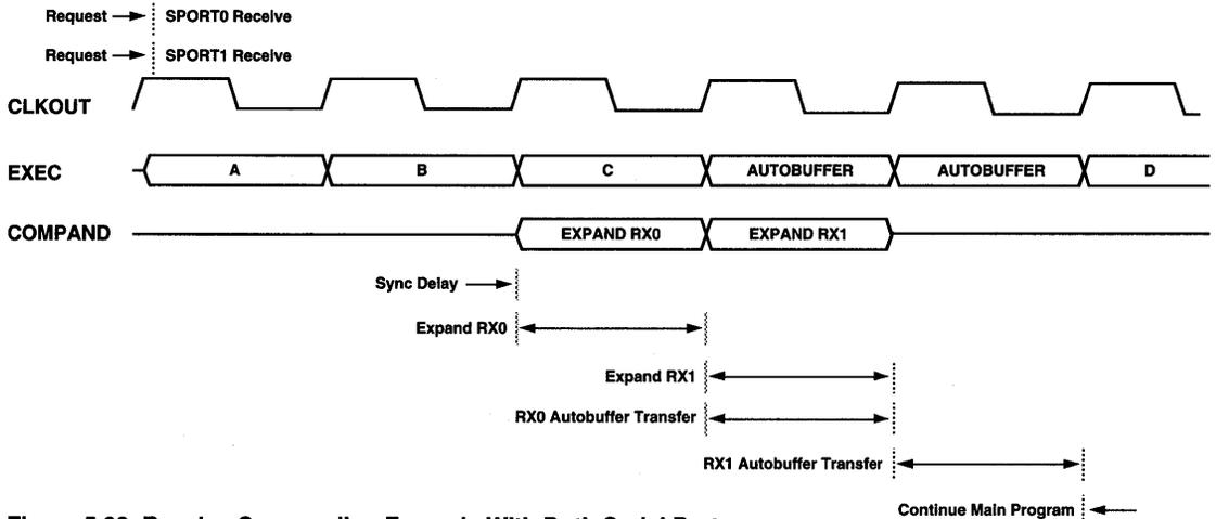
Figure 5.38 Receive Companding Example With Both Serial Ports
