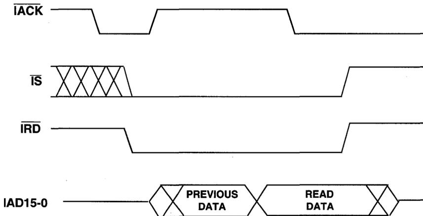
**Figure 11.10 IDMA Long Read Cycle Timing**
