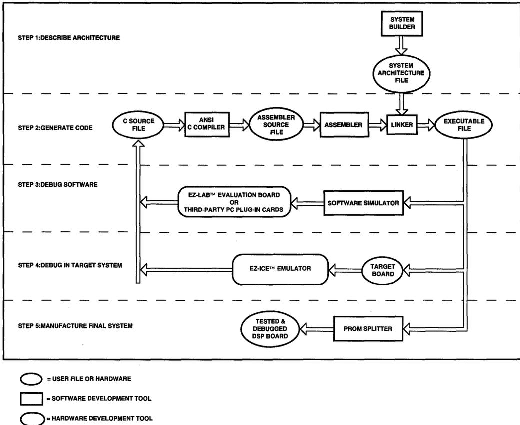
**Figure 14.1 ADSP-2100 Family System Development Process**
