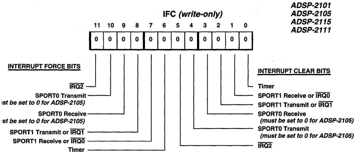
Default bit values at reset are shown; if no value is shown, the bit is undefined at reset.
