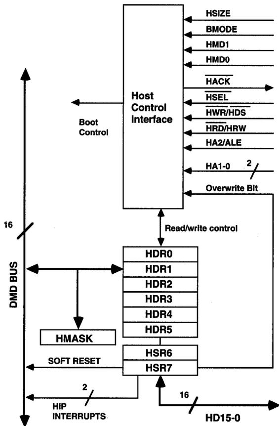
**Figure 7.1 HIP Block Diagram**
