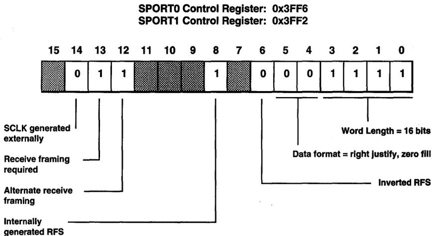
Figure 13.8 SPORT To AD7872 ADC Control Register Settings
