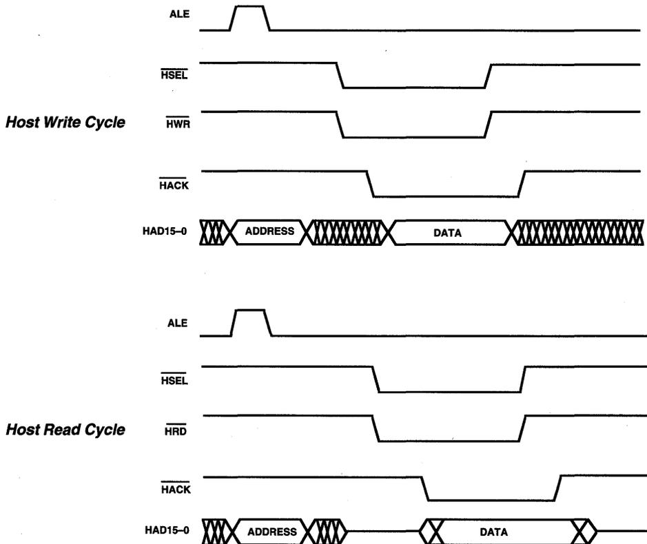
Figure 7.8 HIP Timing: Separate Strobes, Multiplexed Buses
