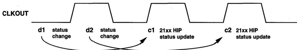
Figure 7.4 ADSP-21xx HIP Status Synchronization
