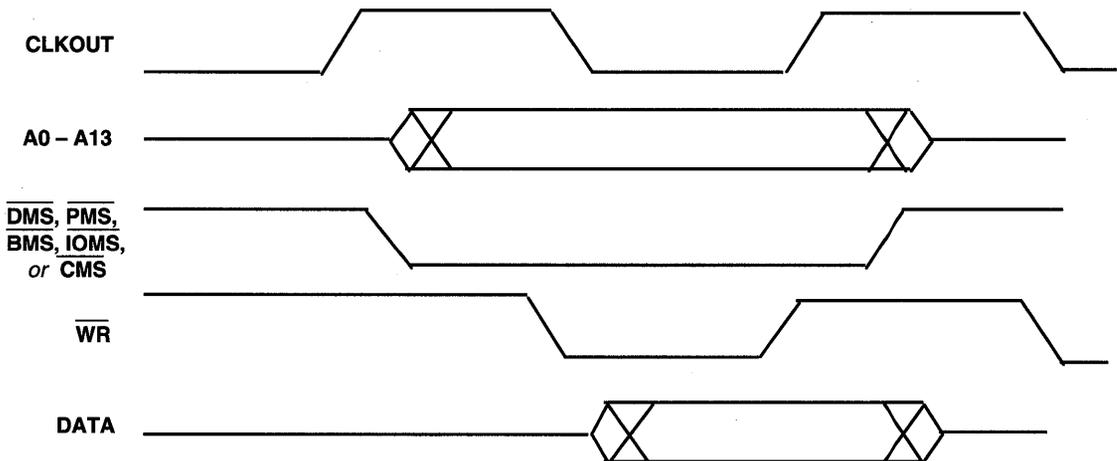
Figure 10.35 External Memory Write Timing
