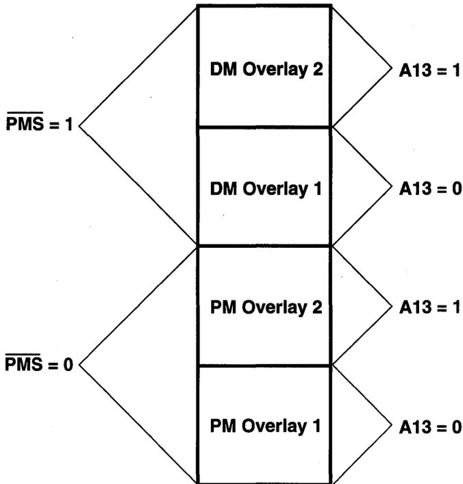
Figure 10.27 Memory Overlay Addressing For Example Design
