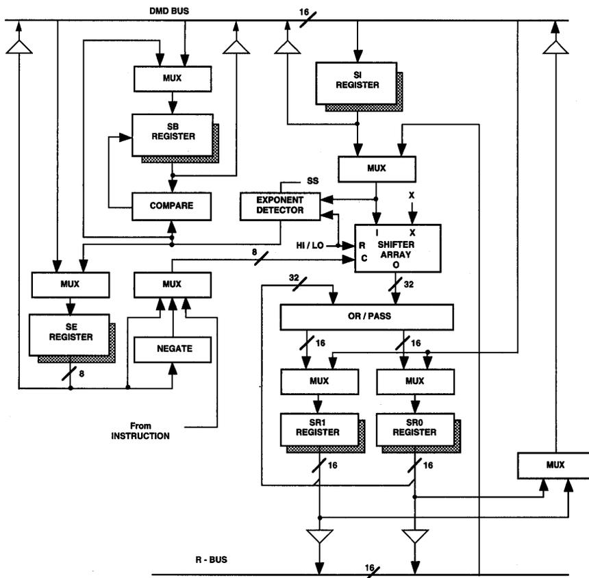
**Figure 2.9 Shifter Block Diagram**
