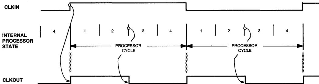
Figure 9.3 Clock Signals & Processor States (ADSP-2171, ADSP-2181, ADSP-21msp58/59)
