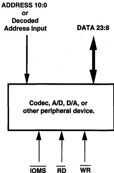
Figure 10.31 I/O Memory Space Peripheral Connection Example
