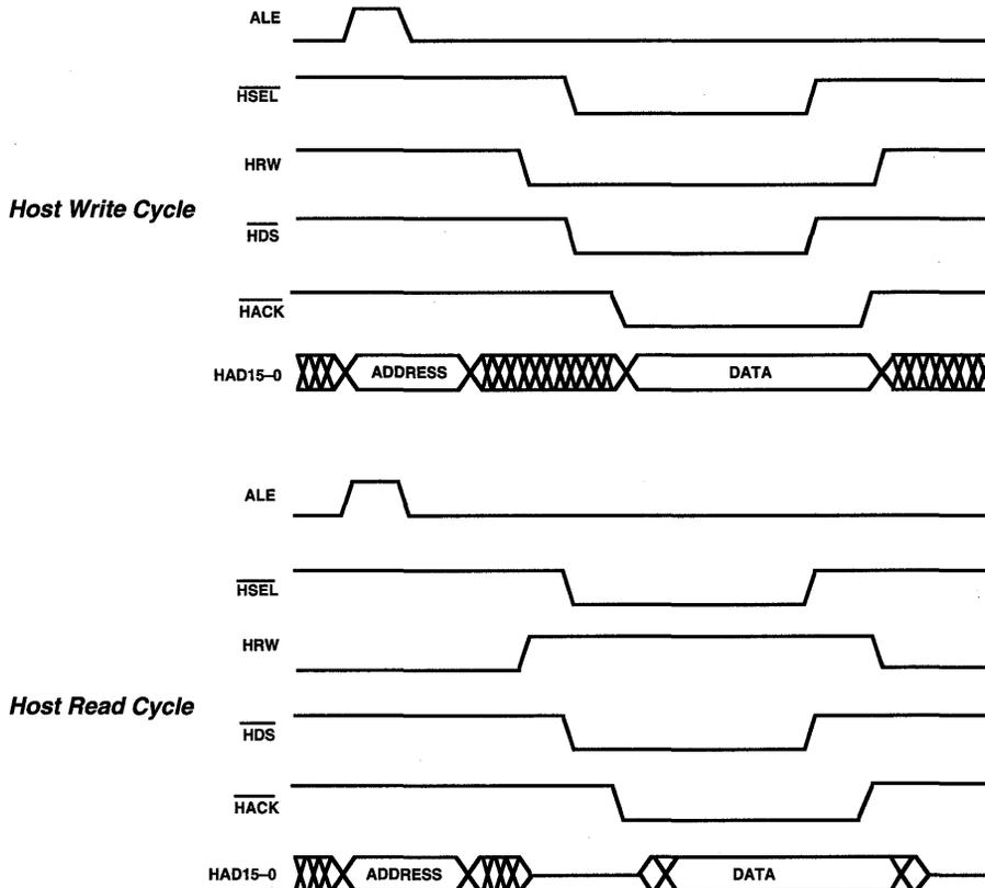
Figure 7.9 HIP Timing: Multiplexed R/W Strobe, Multiplexed Buses
