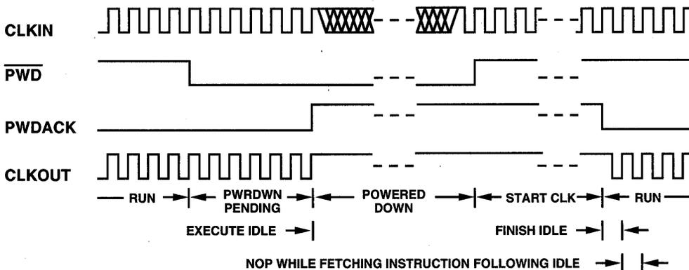
Figure 9.7 Powerdown Timing Example
