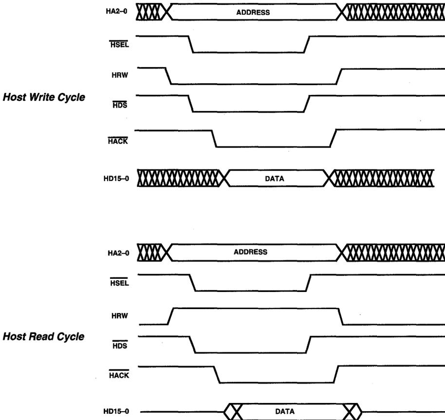
Figure 7.7 HIP Timing: Multiplexed R/W Strobe, Separate Buses
