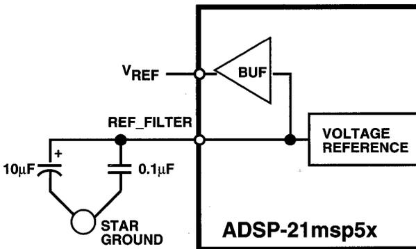
Figure 8.9 Voltage Reference Filter Capacitor
