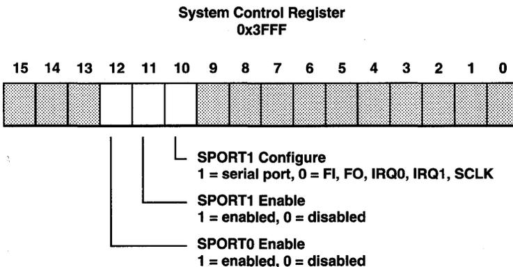
Figure 5.2 SPORT Enables In The System Control Register
