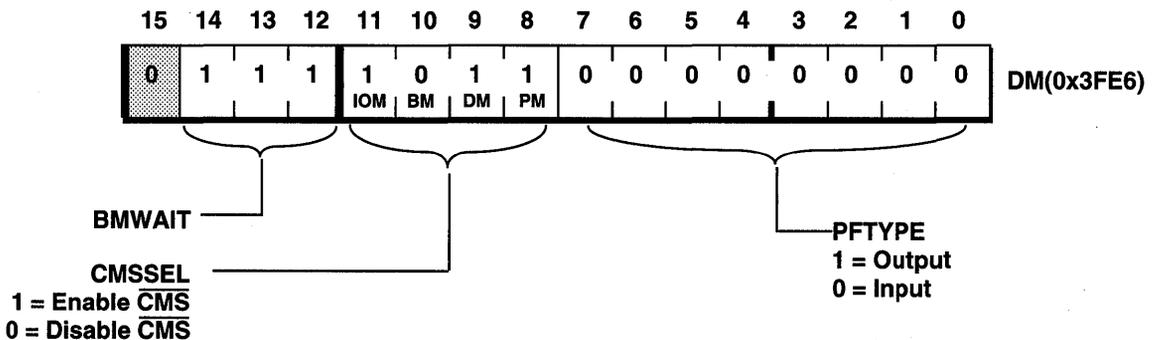
Figure 10.33 CMSSEL Selection for  $\overline{\text{CMS}}$  Signal
