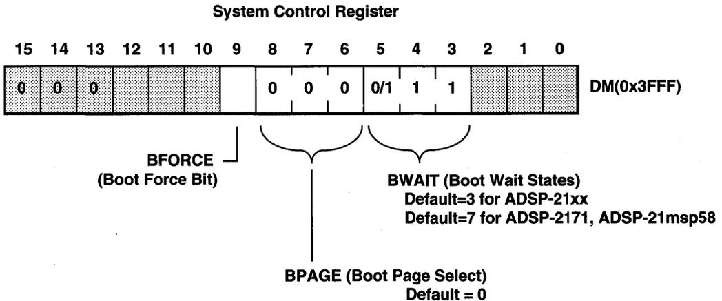
Figure 10.17 Boot Control Fields In System Control Register
