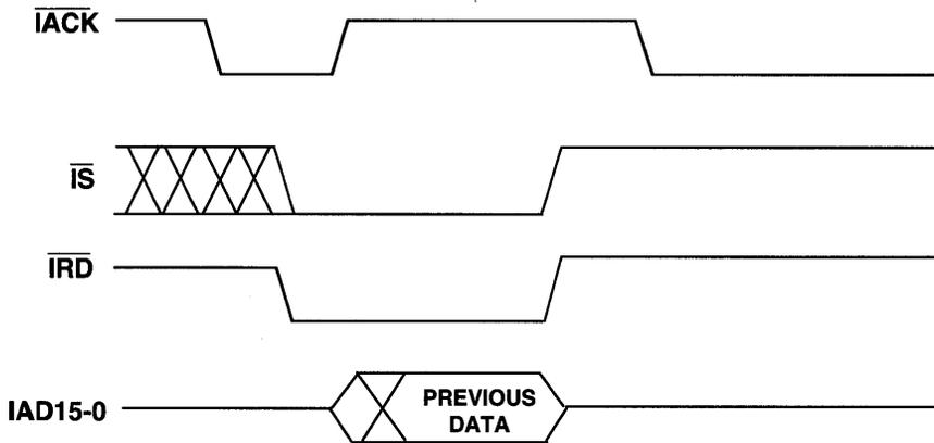
Figure 11.11 IDMA Short Read Cycle Timing
