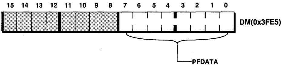
Default bit values at reset are shown; if no value is shown, the bit is undefined at reset. Reserved bits are shown on a gray field—these bits should always be written with zeros.
