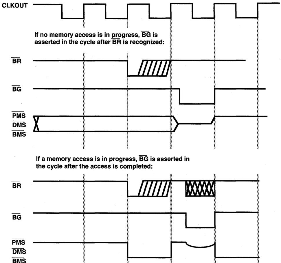
Figure 10.21 Bus Request (with and without external access)
