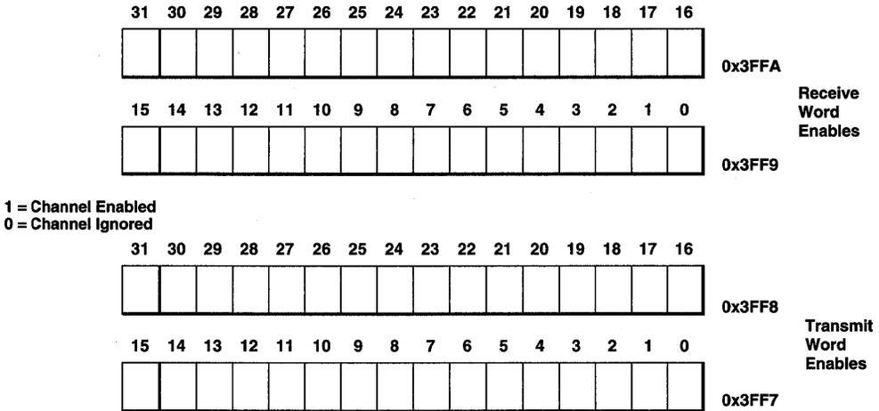
Figure 5.27 SPORT0 Multichannel Word Enable Registers
