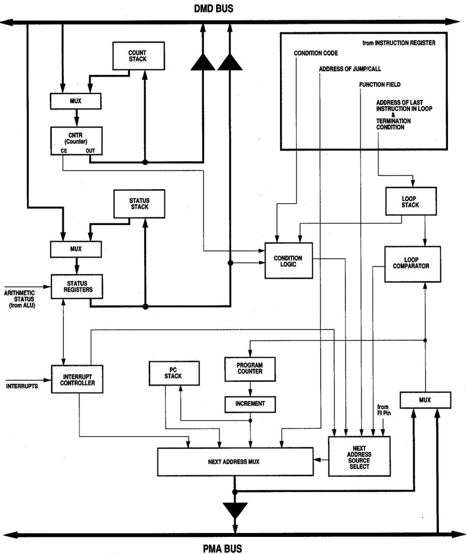
Figure 3.1 Program Sequencer Block Diagram
