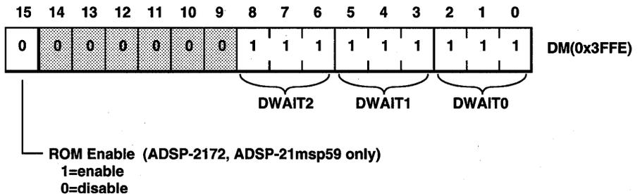
Figure 10.15 Data Memory Waitstate Control Register (ADSP-2171/72, ADSP-21msp58/59)
