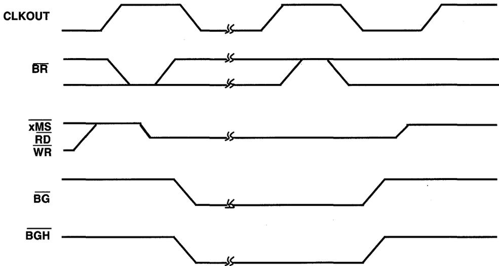
Figure 10.22 Bus Grant Hung (BGH) Timing (ADSP-2171, ADSP-2181 only)
