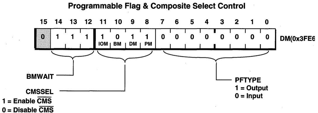
Figure 9.4 Programmable Flag & Composite Select Control Register (ADSP-2181)
