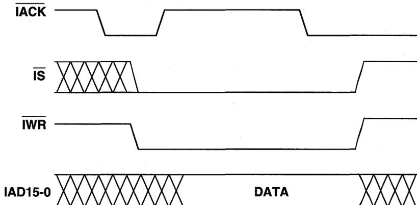
Figure 11.12 IDMA Long Write Cycle Timing
