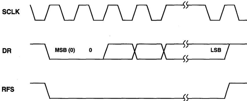
Figure 13.7 SPORT To AD7872 ADC Timing
