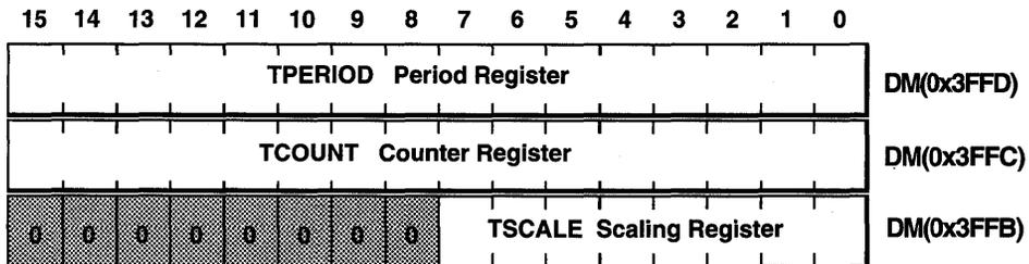
Default bit values at reset are shown; if no value is shown, the bit is undefined at reset.
