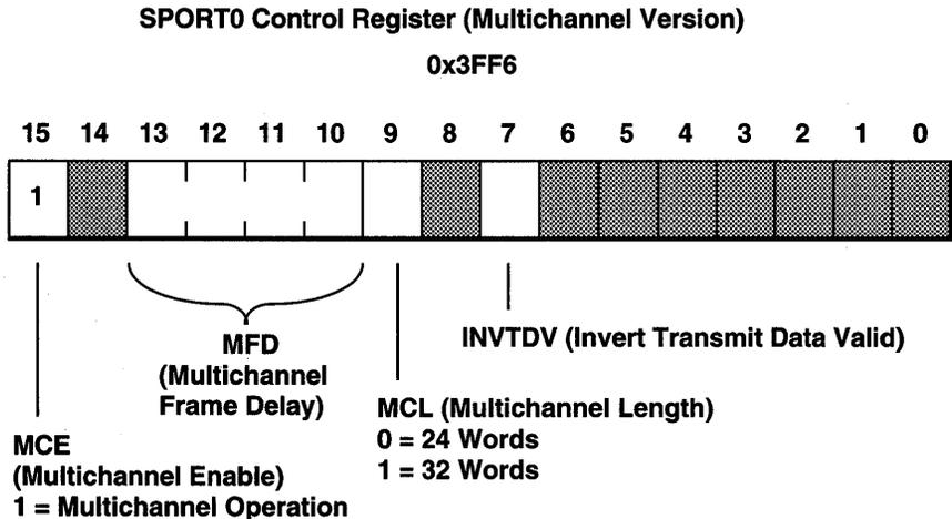
Figure 5.25 SPORT0 Control Register With Multichannel Mode Enabled
