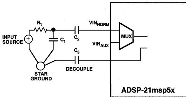
Figure 8.6 Recommended Analog Input Circuit
