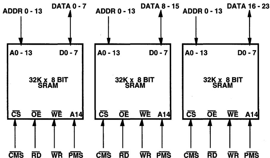
Figure 10.26 Example Program and Data Memory Overlay Design
