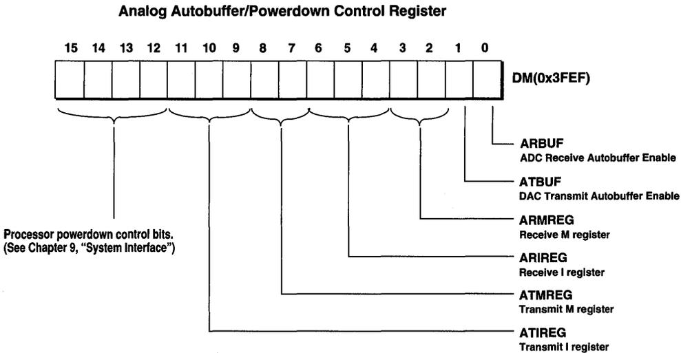
**Figure 8.5 Analog Autobuffer/Powerdown Control Register**
