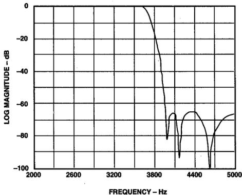
Figure 8.2 IIR Low Pass Filter Frequency Response
