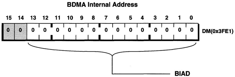
Figure 11.2 BDMA Internal Address Register
