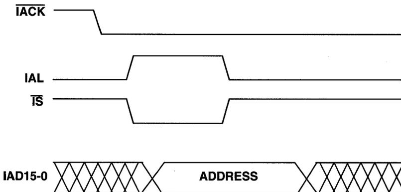
Figure 11.9 IDMA Address Latch Cycle Timing
