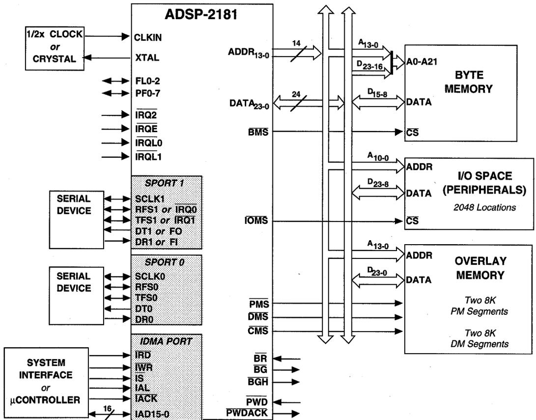
Figure 10.23 ADSP-2181 System Diagram
