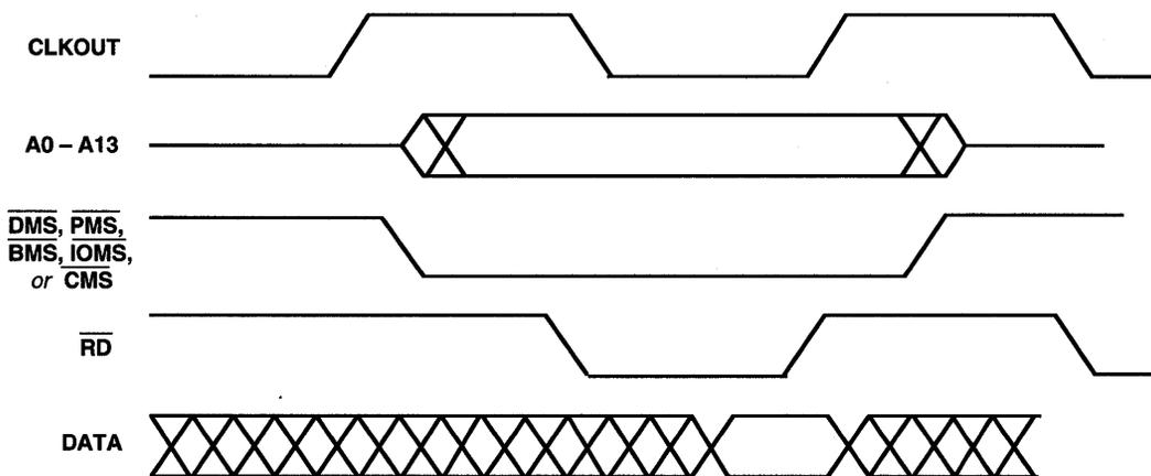
Figure 10.34 External Memory Read Timing
