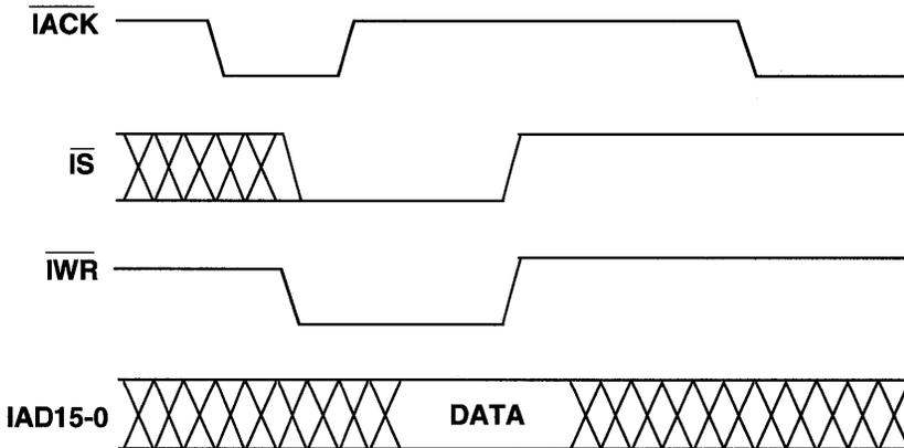
Figure 11.13 IDMA Short Write Cycle Timing
