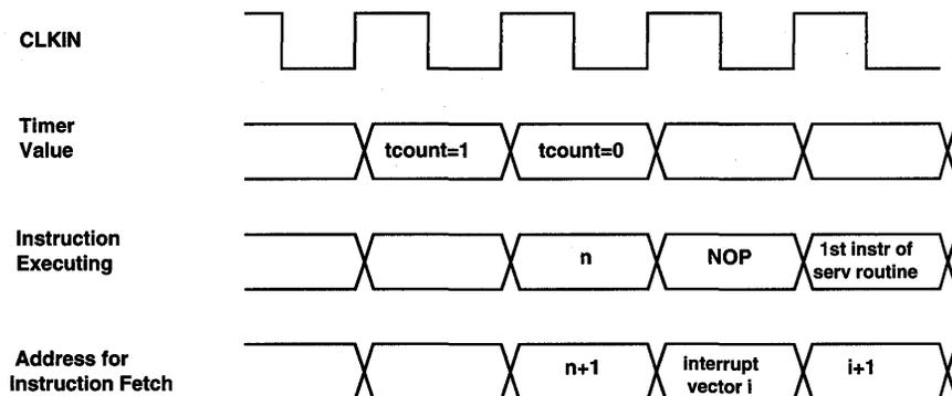
**Figure 3.3 Timer Interrupt Latency for ADSP-2101, ADSP-2105, ADSP-2115, ADSP-2111**
