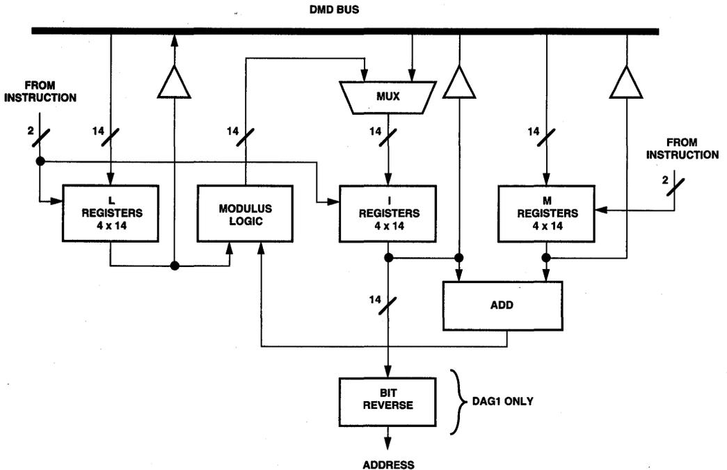
**Figure 4.1 Data Address Generator Block Diagram**
