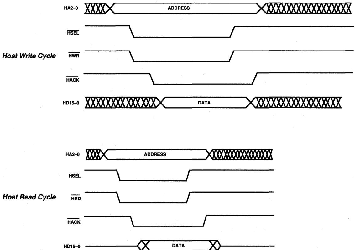
Figure 7.6 HIP Timing: Separate Strobes, Separate Buses
