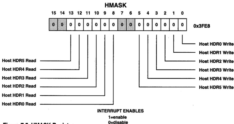
**Figure 7.5 HMASK Register**
