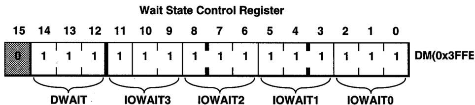
Figure 10.30 ADSP-2181 Waitstate Control Register
