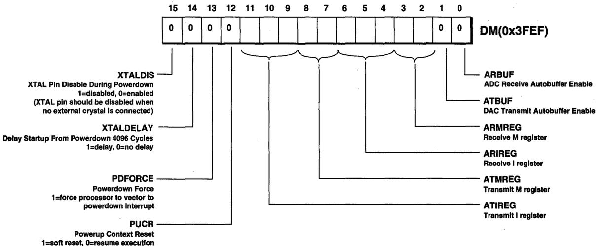
Default bit values at reset are shown; if no value is shown, the bit is undefined at reset.
