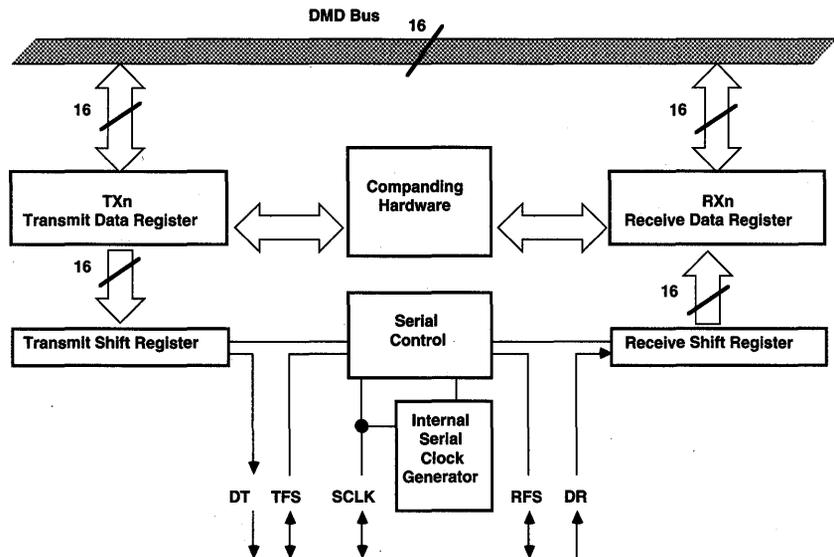
Figure 5.1 Serial Port Block Diagram
