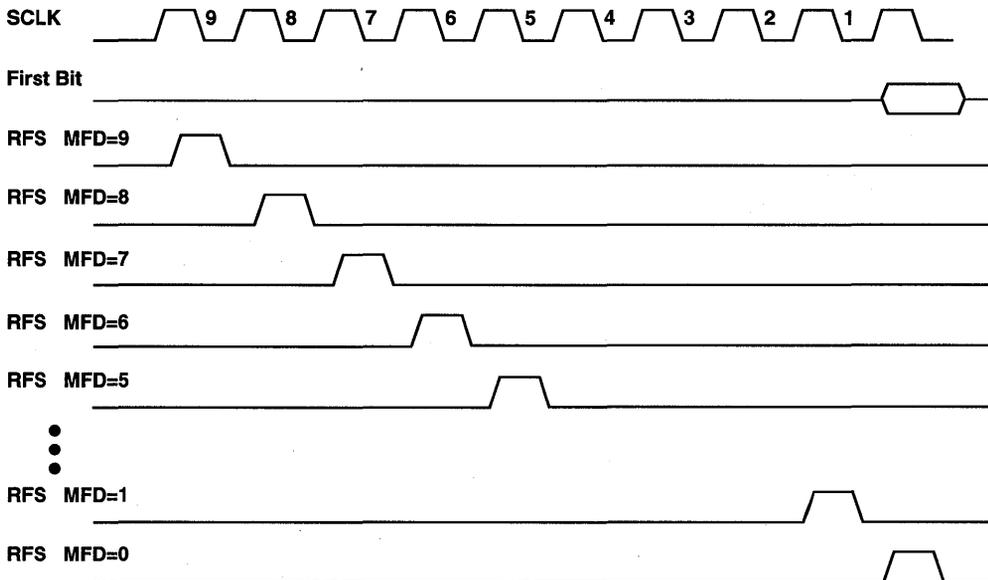
Figure 5.26 SPORT Multichannel Frame Delay Examples
