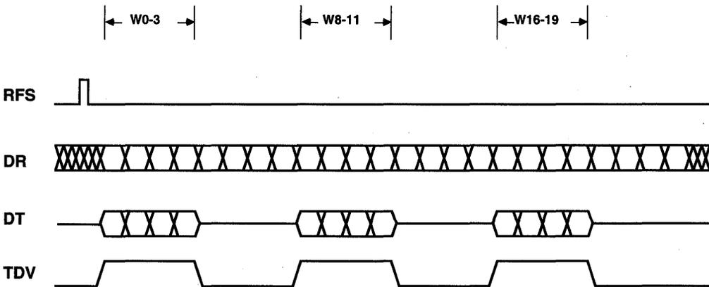
Figure 5.29 Complete Multichannel Example
