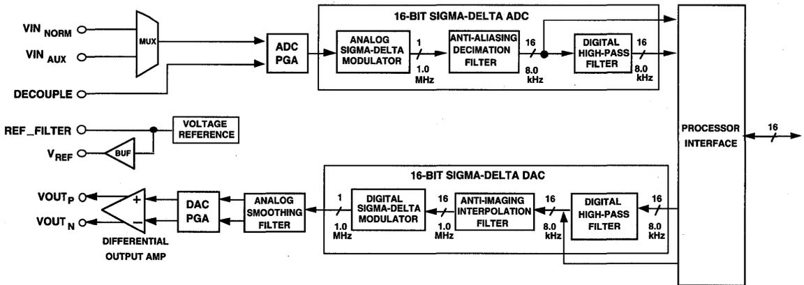
Figure 8.1 Analog Interface Block Diagram (ADSP-21msp58/59)
