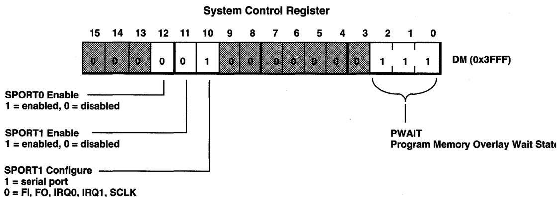
**Figure 10.24 PWAIT Field in System Control Register**
