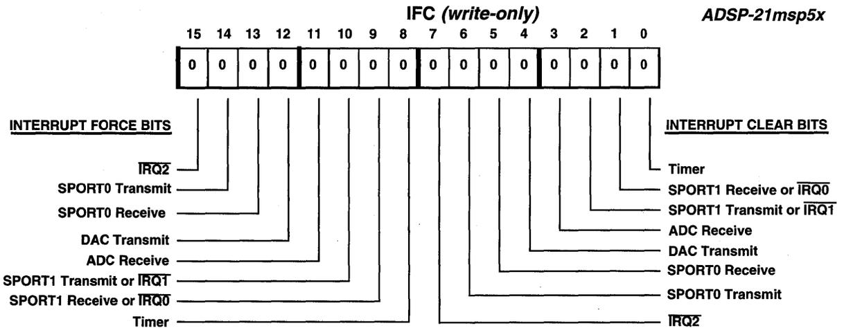
Default bit values at reset are shown; if no value is shown, the bit is undefined at reset.
