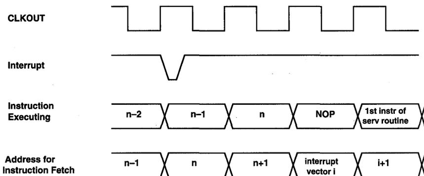
**Figure 3.2 Interrupt Latency (Timer,  $IRQ_x$ , SPORT, HIP, & Analog Interrupts)**
