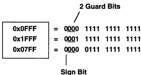
To detect bit growth into 2 guard bits, set SB=-2
