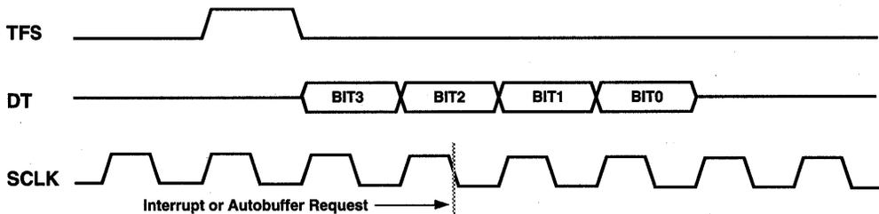
Figure 5.31 SPORT Interrupt or Autobuffer Timing, Transmit 4-Bit Words (No Companding)
