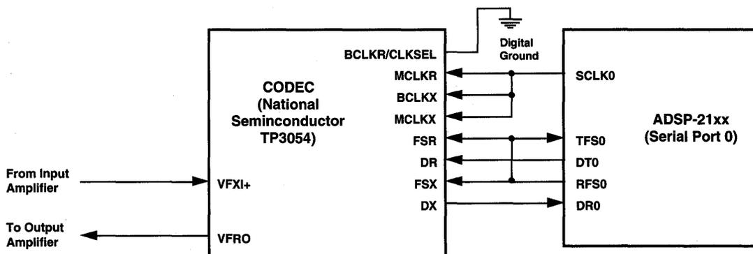
Figure 13.2 ADSP-21xx Serial Port (SPORT0) To CODEC
