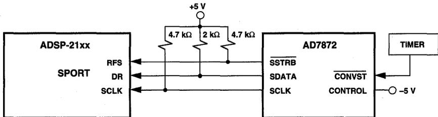
Figure 13.6 Serial Port Interface To AD7872 ADC
