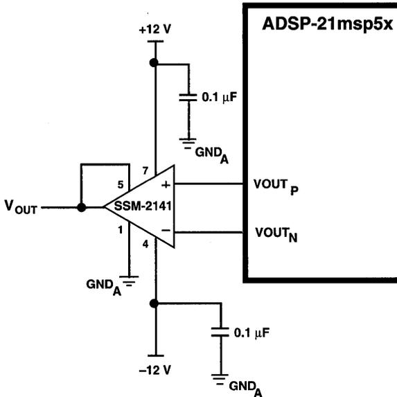
Figure 8.8 Example Circuit For Single-Ended Output
