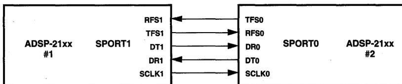
Figure 13.9 Serial Port Interface Between Two ADSP-21xx Processors
