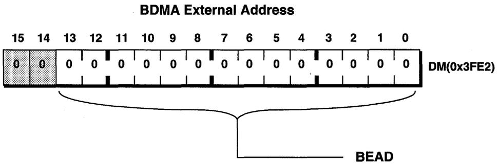
Figure 11.3 BDMA External Address Register
