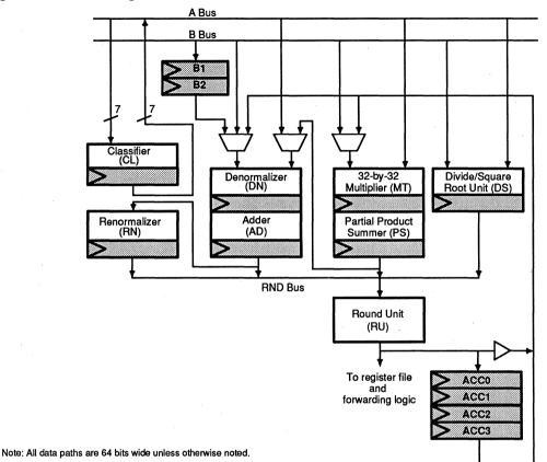
Denormalizer (DN)—Equalizes the exponent values of two floating-point operands by right-shifting the significand of the smaller operand.
