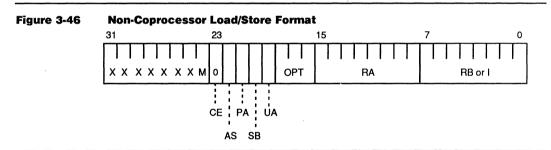
In load and store instructions, the RB or I field specifies the address for access. The address is either the content of a general-purpose register, with register number RB, or a constant with a value I (zero-extended to 32 bits). The M bit determines whether the register or the constant is used.
