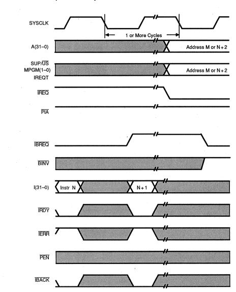
Figure A-10 Instruction Read—Burst-Mode Access Ended by Master (Preempted, Terminated, or Canceled)
