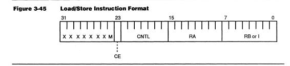
Addresses for accesses are given either by the content of a general-purpose register or by a constant value specified by the load or store instruction. The load and store instructions do not perform address computation directly. Any required address computations are performed explicitly by other instructions.
