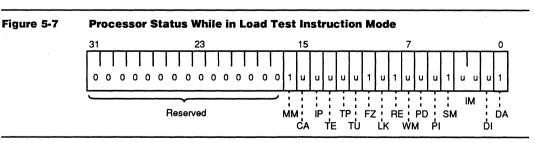
The visible processor state, including the Shadow Program Counter Registers, remains unchanged while the processor is in the Load Test Instruction Mode. The processor status shown in Figure 5-7 remains in effect until the next transition to the Normal Mode via the Halt Mode.
