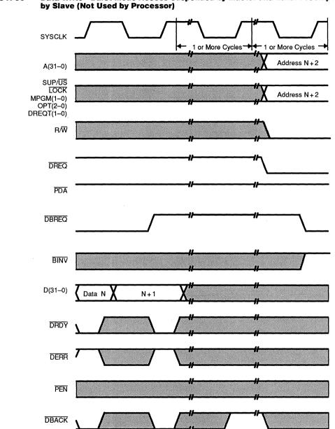
Figure A-33 Data Write—Burst-Mode Access Suspended by Master and Later Preempted by Slave (Not Used by Processor)
