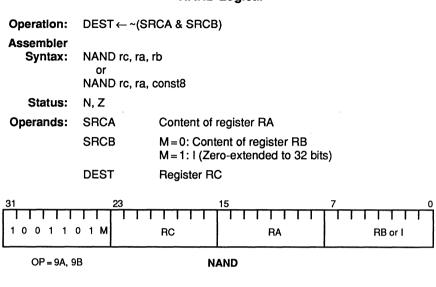
**Description:** The SRCA operand is logically ANDed, bit-by-bit, with the SRCB operand. The one's-complement of the result is placed into the DEST location.
