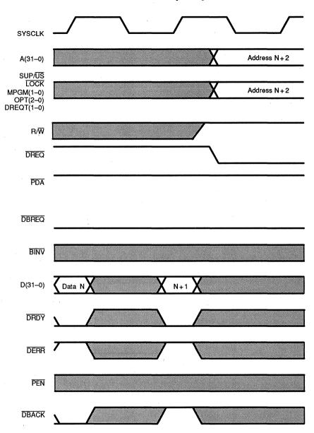
Figure A-31 Data Write—Burst-Mode Access Preempted by Slave
