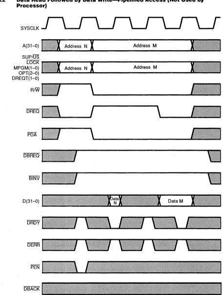
Data Read Followed by Data Write—Pipelined Access (Not Used by Figure A-22
