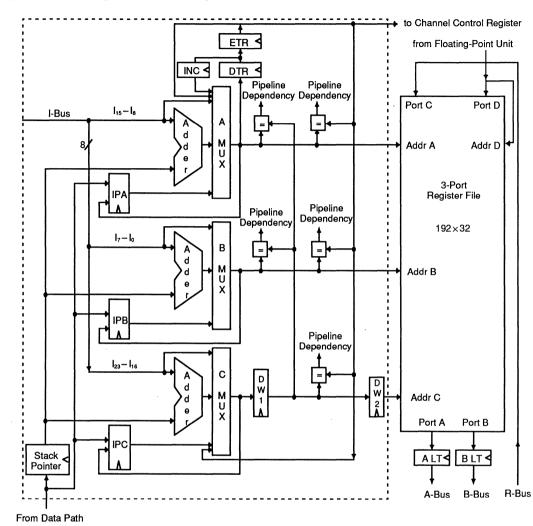
Figure 4-7 Register File and Register Address Generator
