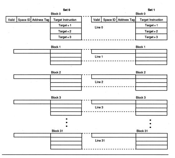
A 29-bit cache tag is associated with each block. Of the 29 bits, 26 are derived from the address (possibly virtual) of the instructions in the block and are called the Address Tag.
