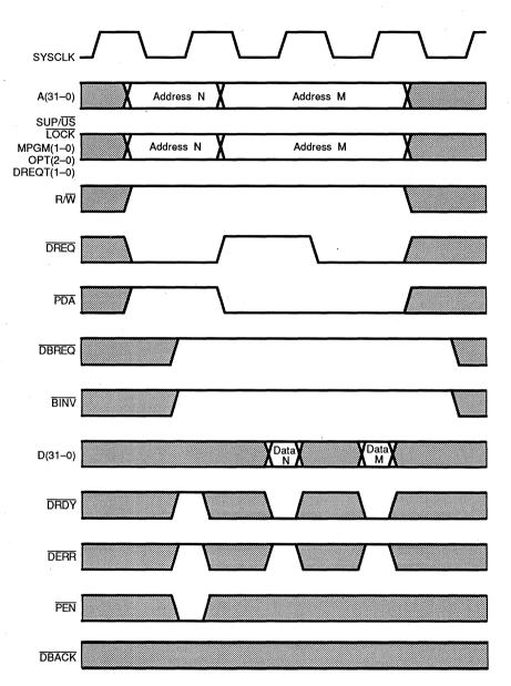
Figure A-21 Data Write—Pipelined Access
