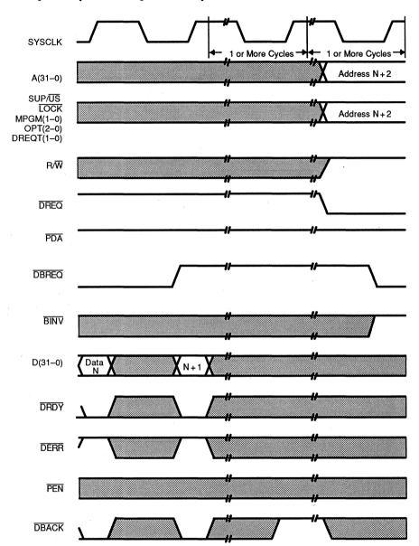
Figure A-32 Data Read—Burst-Mode Access Suspended by Master and Later Preempted by Slave (Not Used by Processor)
