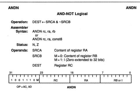
**Description:** The SRCA operand is logically ANDed, bit-by-bit, with the one's-complement of the SRCB operand, and the result is placed into the DEST location.
