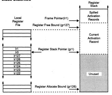
The processor performs no hardware management of the stack cache, and cannot detect a reference to a quantity that is not in the stack cache. Consequently, software must keep the size of an activation record less than or equal to the size of the local register file (128 words). Any additional storage requirements are satisfied by the Memory Stack.
