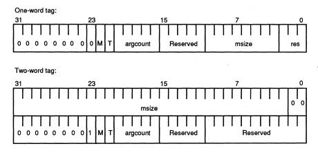
address within a procedure. The call sequence up to the current point in execution can be determined from the *rsize* and *msize* values in the trace-back tag. However, for procedures that perform dynamic stack allocation (e.g., using alloca()), the memorv frame pointer must be used.
