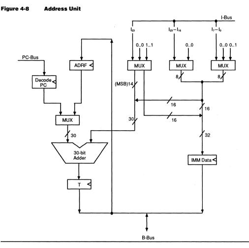
2. Absolute: a zero-extended, 16-bit field of the branch instruction is used directly as an instruction address.
