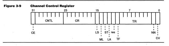
The Channel Control Register is updated on the execution of every load or store instruction, and on every load or store in a load-multiple or store-multiple sequence, except when the Freeze (FZ) bit in the Current Processor Status Register is 1.
