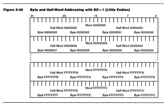
In the processor, the two least-significant bits of an external address can be reflected in the Byte Pointer (BP) field of the ALU Status Register when the DW bit of the Configuration Register is 0. Alternatively, the two least-significant bits of the address can be used to control byte and half-word accesses when the DW bit is 1. The BO bit affects only the interpretation of the BP field and the two least-significant address bits.
