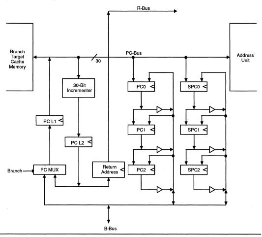
fetched in the Instruction Fetch Unit. The slave of the PC Register, PC L2, contains the next sequential address, which may be fetched by the Instruction Fetch Unit in the next cycle.
