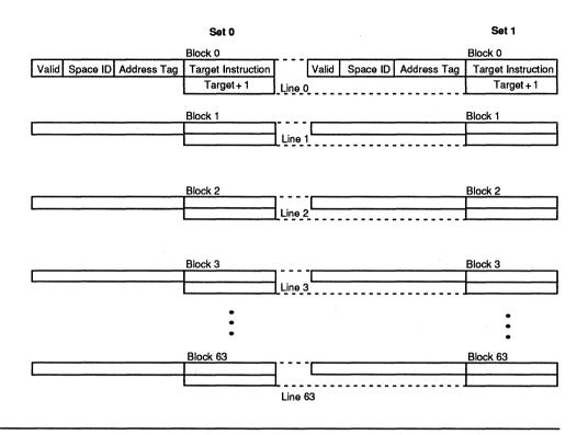
physical address space, and the program mode under which the instructions were fetched (Supervisor or User). When instructions are placed into the Branch Target Cache memory, the Space ID bits are written with the values of the following bits of the Current Processor Status Register: ROM Enable (RE), Physical Addressing/Instructions (PI), and Supervisor Mode (SM).
