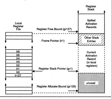
The register allocate bound (*rab*, gr126) pointer defines the lowest-addressed stack location that can be cached within the local registers. This defines the limit to which local registers can be allocated in the Register Stack.
