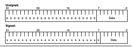
If the Data Width Enable (DW) bit of the Configuration Register is 1, the Am29050 microprocessor is enabled to load and store byte data. On a load, an external packed byte is converted to one of the character formats shown in Figure 3-41. On a store, the low-order byte of a word is packed into every byte of an external word. Section 3.4.6 describes external byte accesses in more detail.
