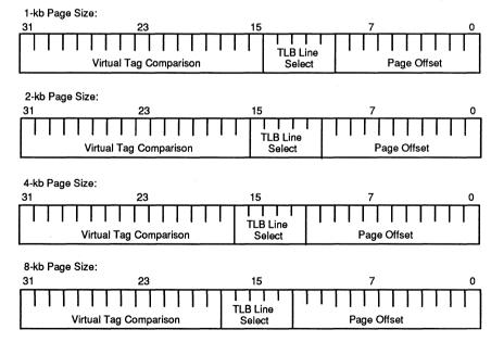
The TLB address-translation process is diagrammed in Figure 3-54. Address translation is performed by the following fields in the TLB entry: the Virtual Tag (VTAG), the Task Identifier (TID), the Valid Entry (VE) bit, the Real Page Number (RPN) field, and the Input/Output (IO) bit. To perform an address translation, the processor accesses the TLB line whose number is given by certain bits in the virtual address. The bits used depend on the page size as follows:
