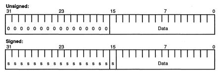
The Extract Half-Word (EXHW) instruction replaces the low-order half-word of a destination word with either the low-order or high-order half-word of a source word. For the EXHW instruction, the destination word can be a zero word, which effectively zeroextends the half-word from the source operand.
