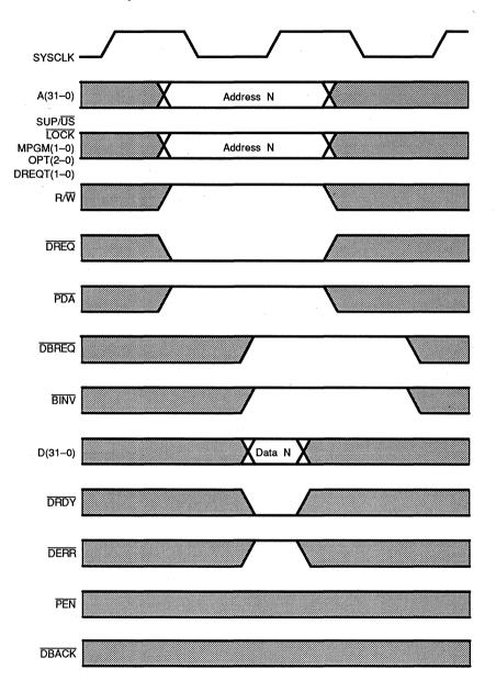
Figure A-15 Data Write—Simple Access
