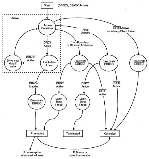
Note: The Am29050 microprocessor does not suspend burst-mode data accesses.
