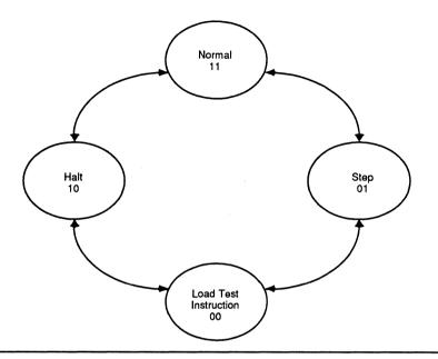
The Halt mode can be invoked by applying a value of 10 to the CNTL(1-0) inputs. The processor enters the Halt mode within two or three cycles after the CNTL(1-0) inputs are changed (depending on synchronization time), except that it first completes any external data access in progress.
