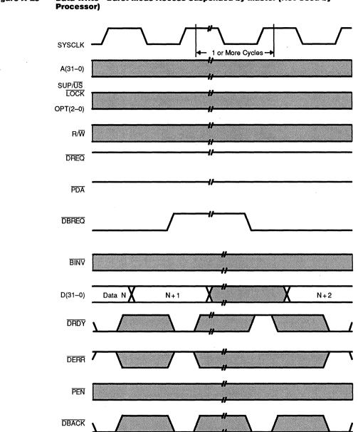
Figure A-29 Data Write—Burst-Mode Access Suspended by Master (Not Used by
