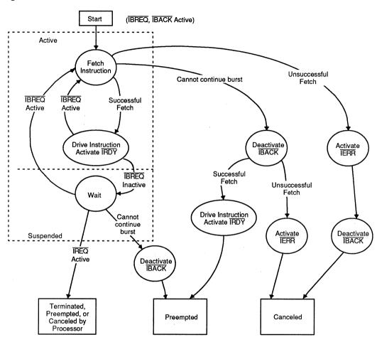
Figure 5-3 Slave Burst-Mode Instruction Accesses: Control Flow
