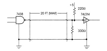
Figure 5-2. ST506 Control Signal Driver/Receiver Circuit
