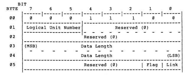
Figure 6-32. RECEIVE DIAGNOSTIC Command
