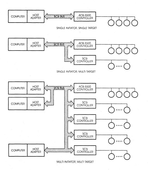
Figure 2-3. Typical SCSI Configurations
