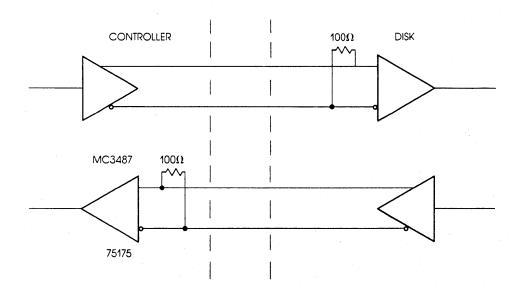
Figure 5-3. MFM Data Driver/Receiver Circuit
