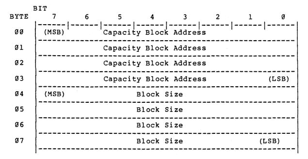
Figure 6-38 shows the format of the capacity data returned.
