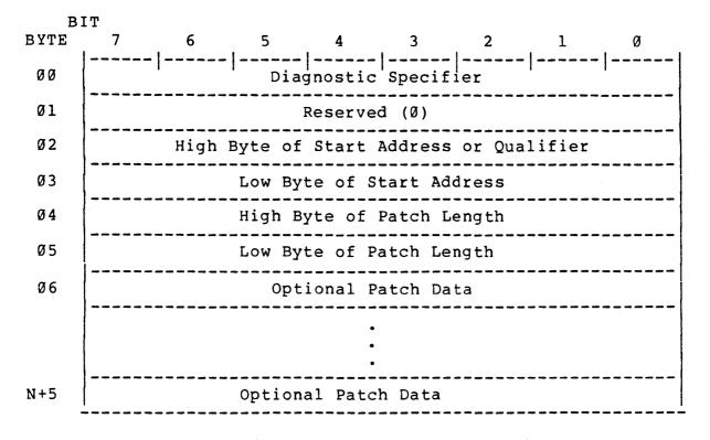
Figure 6-35. SEND DIAGNOSTIC Parameter Format
