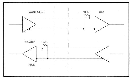
Figure 3-6. ACB-4000 Data Receiver/Driver Pairs
