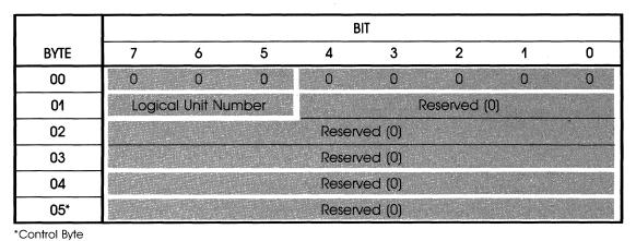
Figure 6-3. TEST UNIT READY Command
