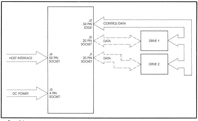
Figure 3-4. System Interconnect Diagram
