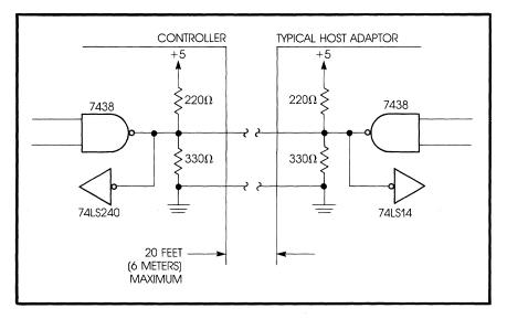
Figure 3-3. Host Adapter Bus Termination
