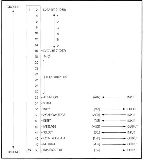
Figure 3-1. SCSI Bus Pin Assignments
