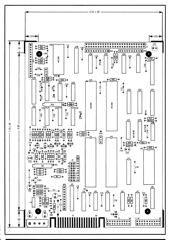
Figure 3-2. ACB-4000 Board Layout and Connectors
