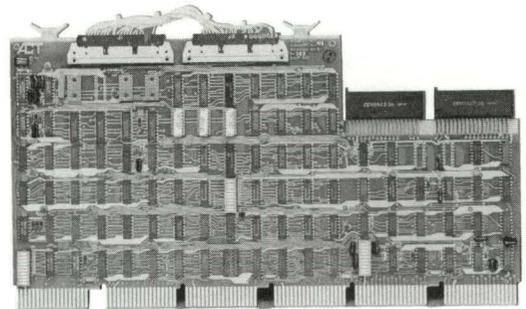
The INTERLINK/UNI is a hex width board, INTERLINK/LSI is a quad width board, and BUSLINKS are combinations of two INTERLINK boards.
