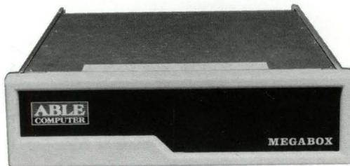
The system also is available as a self-contained unit called MEGABOX, consisting of an ENABLE control board, backplane, a one megabyte memory board, bus terminator board and power supply, with room for the optional cache.
