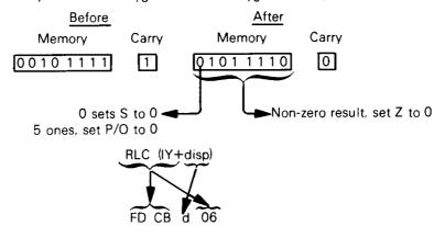
This instruction is identical to RLC (IX+disp), but uses the IY register instead of the IX register.
