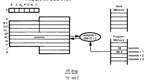
Add the contents of the JR instruction object code second byte, the contents of the Program Counter, and 2. Load the sum into the Program Counter. The jump is measured from the address of the instruction operation code, and has a range of -126 to  $\pm$ 129 bytes. The Assembler automatically adjusts for the twice-incremented PC.
