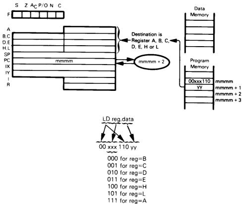
Load the contents of the second object code byte into one of the registers.
