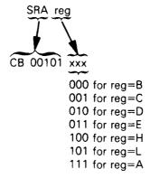
Shift specified register right one bit. Most significant bit is unchanged. Suppose Register H contains 59<sub>16</sub>, and Carry=0. After the instruction SRA H
