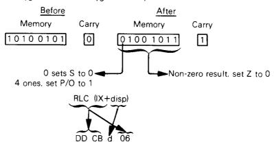
Rotate memory location (specified by the sum of the contents of Index register IX and displacement integer d) left one bit, copying bit 7 into Carry.
