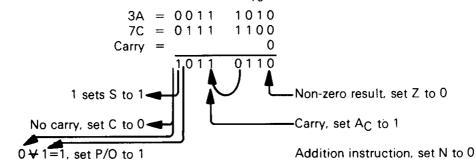
The ADC instruction is frequently used in multibyte addition for the second and subsequent bytes.
