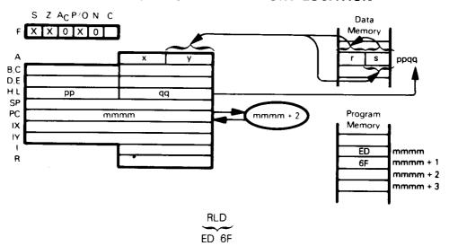
The four low-order bits of a memory location (specified by the contents of register pair HL) are copied into the four high-order bits of the same memory location. The previous contents of the four high-order bits of that memory location are copied into the four low-order bits of the Accumulator. The previous four low-order bits of the Accumulator are copied into the four low-order bits of the specified memory location.
