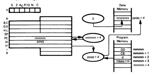
The illustration shows execution of SET b, (IX+disp). Bit 0 is execution of SET b, (IX+disp). Bit 0 is the least significant bit.
