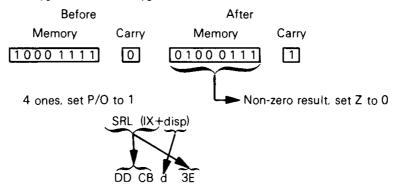
Shift contents of memory location (specified by the sum of the contents of the IX register and the displacement value d) right one bit. Most significant bit is reset to 0.
