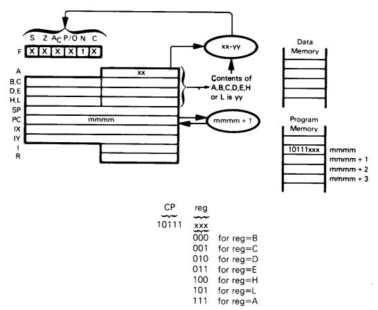
Subtract the contents of Register A, B, C, D, E, H or L from the contents of the Accumulator, treating both numbers as simple binary data. Discard the result; i.e., leave the Accumulator alone, but modify status flags to reflect the result of the subtraction.
