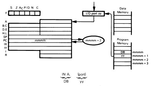
Load a byte of data into the Accumulator from the I/O port (identified by the second IN instruction object code byte).
