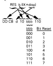
Reset indicated bit within memory location indicated by the sum of Index Register IX and d.
