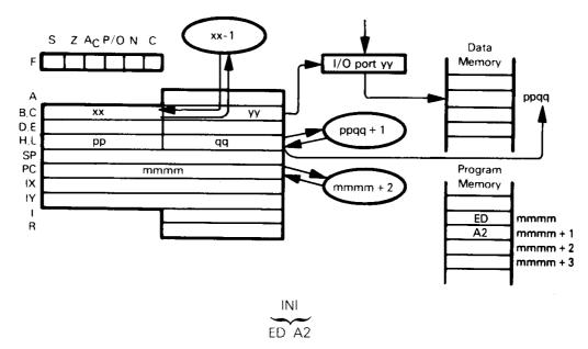
Input from I/O port (addressed by Register C) to memory location (specified by HL). Decrement Register B: increment register pair HL.
