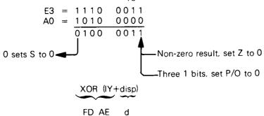
This instruction is identical to XOR (IX+disp), except that it uses the IY register instead of the IX register.
