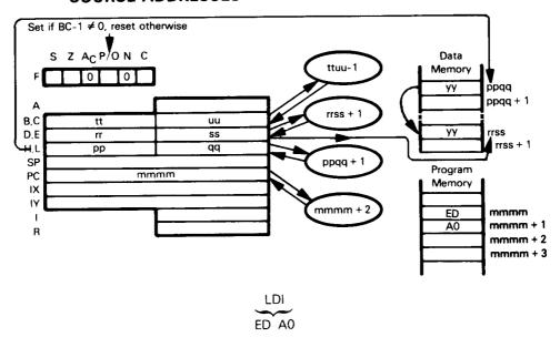
Transfer a byte of data from memory location addressed by the HL register pair to memory location addressed by the DE register pair. Increment contents of register pairs HL and DE. Decrement contents of the BC register pair.
