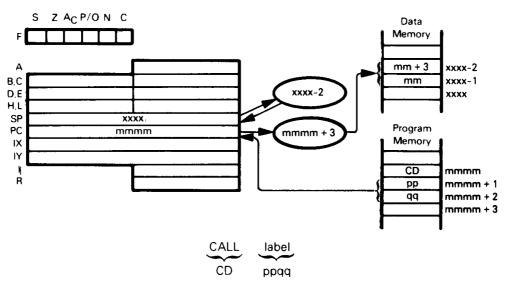
Store the address of the instruction following the CALL on the top of the stack: the top of the stack is a data memory byte addressed by the Stack Pointer. Then subtract 2 from the Stack Pointer in order to address the new top of stack. Move the 16-bit address contained in the second and third CALL instruction object program bytes to the Program Counter. The second byte of the CALL instruction is the low-order half of the address, and the third byte is the high-order byte.
