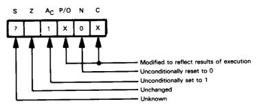
An X identifies a status that is set or reset. A 0 identifies a status that is always cleared. A 1 identifies a status that is always set. A blank means the status does not change. A question mark (?) means the status is not known.
