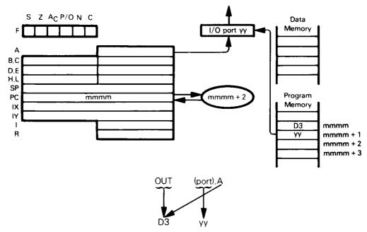
Output the contents of the Accumulator to the I/O port identified by the second OUT instruction object code byte.
