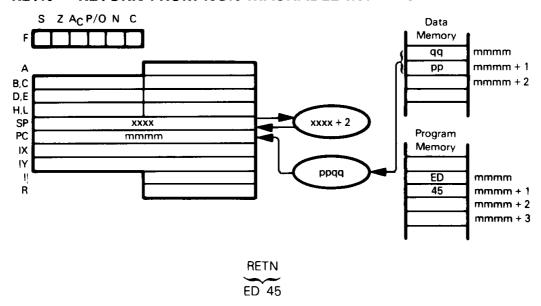
Move the contents of the top two stack bytes to the Program Counter; these two bytes provide the address of the next instruction to be executed. Previous Program Counter contents are lost. Increment the Stack Pointer by 2 to address the new top of stack. Restore the interrupt enable logic to the state it had prior to the occurrence of the non-maskable interrupt.
