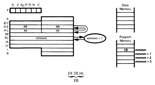
The D and E registers' contents are swapped with the H and L registers' contents. Suppose pp=03<sub>16</sub>, qq=2A<sub>16</sub>, xx=41<sub>16</sub> and yy=FC<sub>16</sub>. After the instruction
