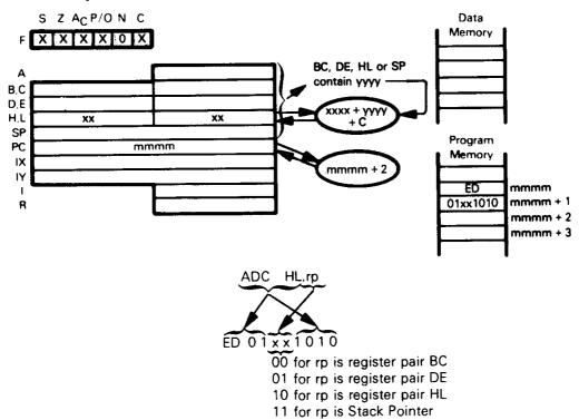
Add the 16-bit value from either the BC, DE, HL register pair or the Stack Pointer, and the Carry status, to the HL register pair.
