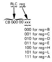
Rotate contents of specified register left one bit, copying bit 7 into Carry.
