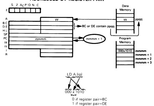
Load the contents of the memory byte (addressed by the BC or DE register pair) into the Accumulator.
