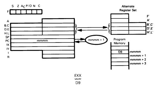
The contents of register pairs BC, DE and HL are swapped with the contents of register pairs B'C', D'E', and H'L'.
