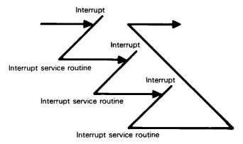
By inhibiting interrupts for one more instruction following execution of El, the Z80 CPU ensures that the RET instruction gets executed in the sequence:
