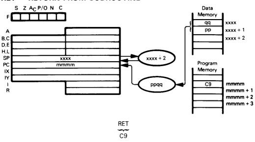
Move the contents of the top two stack bytes to the Program Counter; these two bytes provide the address of the next instruction to be executed. Previous Program Counter contents are lost. Increment the Stack Pointer by 2, to address the new top of stack.
