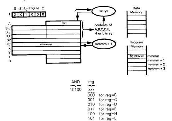
AND the Accumulator with the contents of Register A, B, C, D, E, H or L. Save the result  $\rightarrow$  in the Accumulator.
