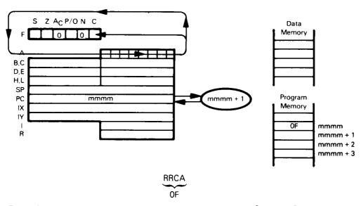
Rotate Accumulator contents right one bit circularly, copying bit 0 into the Carry status. Suppose the Accumulator contains  $7A_{16}$  and the Carry status is set to 1. After the instruction
