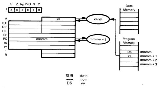
Subtract the contents of the second object code byte from the Accumulator.
