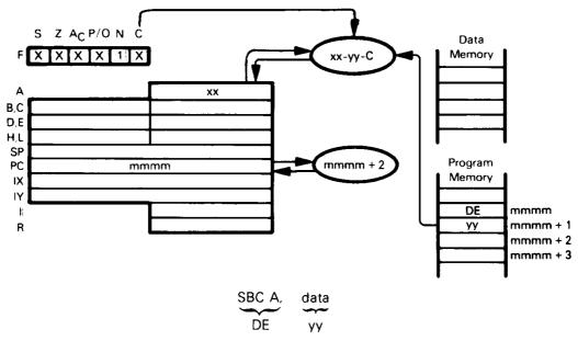
Subtract the contents of the second object code byte and the Carry status from the Accumulator.
