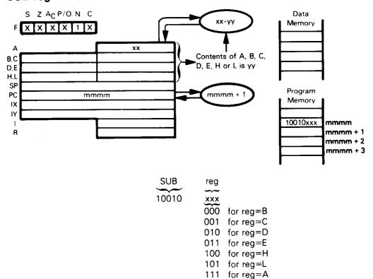
Subtract the contents of the specified register from the Accumulator.
