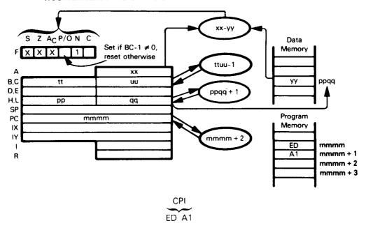
Compare the contents of the Accumulator with the contents of memory location (specified by the HL register pair). If A is equal to memory, set the Z flag. Increment the HL register pair and decrement the BC register pair (BC is used as Byte Counter).
