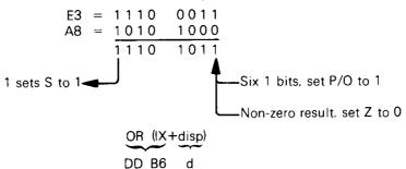
OR contents of memory location (specified by the sum of the contents of the IX register and the displacement value d) with the Accumulator.
