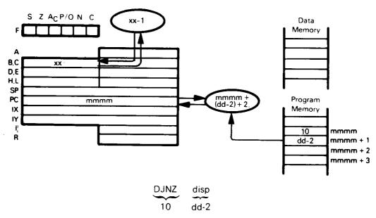
Decrement Register B. If remaining contents are not zero, add the contents of the DJNZ instruction object code second byte and 2 to the Program Counter. The jump is measured from the address of the instruction operation code, and has a range of -126 to +129 bytes. The Assembler automatically adjusts for the twice-incremented PC.
