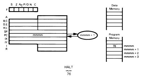
When the HALT instruction is executed, program execution ceases. The CPU requires an interrupt or a reset to restart execution. No registers or statuses are affected; however, memory refresh logic continues to operate.
