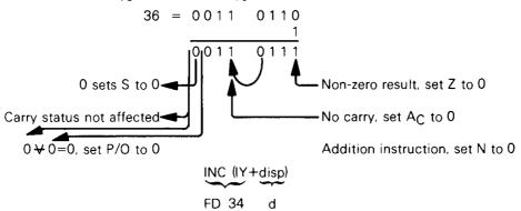
This instruction is identical to INC (IX+disp), except that it uses the IY register instead of the IX register.
