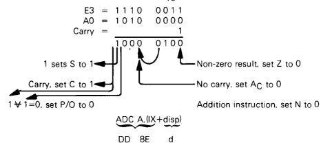
Add the contents of memory location (specified by the sum of the contents of the IX register and the displacement digit d) and the Carry to the Accumulator.
