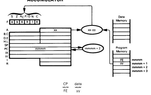
Subtract the contents of the second object code byte from the contents of the Accumulator, treating both numbers as simple binary data. Discard the result; i.e., leave the Accumulator alone, but modify the status flags to reflect the result of the subtraction.
