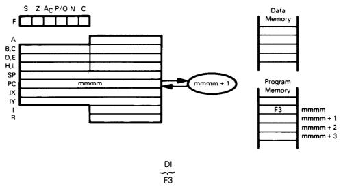
When this instruction is executed, the maskable interrupt request is disabled and the  $\overline{\text{INT}}$  input to the CPU will be ignored. Remember that when an interrupt is acknowledged, the maskable interrupt is automatically disabled.
