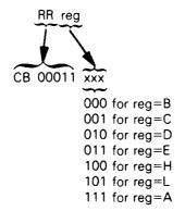
Rotate contents of specified register right one bit through Carry.
