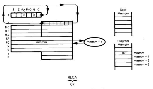
Rotate Accumulator contents left one bit, copying bit 7 into Carry.
