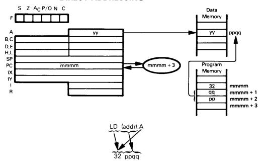
Store the Accumulator contents in the memory byte addressed directly by the second and third bytes of the LD (addr), A instruction object code.
