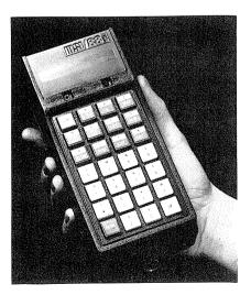
FIGURE 5-7. The MSI Data Corporation MSI 88f is a programmable portable terminal able to provide a handful of sophisticated operations. (Photo courtesy of MSI Data Corporation.)
