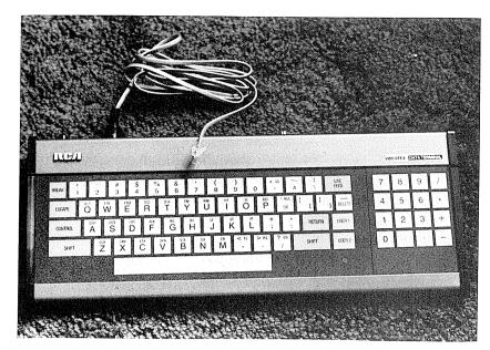
FIGURE 5-8. The RCA VP-3501 portable terminal includes an integrated modem and video modulator to allow direct connection to any television set.
