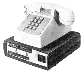
FIGURE 6-5. The Lynx modem connects directly to the data bus of TRS-80 Model I and III computers. Versions are available which provide complete auto-answer and auto-dial capabilities.
