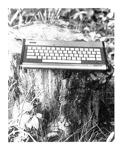
FIGURE 5-2. The RCA VP 3303 Data Terminal is a unique device in many ways. It is designed for use with information utilities and Videotext systems. It features a full keyboard, which is rugged and water resistant. It can use a home television set or monitor to display color and graphic screens of information and data. The system includes sound effects and many other operating features.
