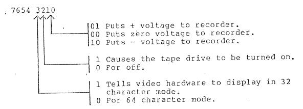
Creating square wave music on the tape output line is a matter of outputting the correct number to port 255 at the correct time. An example of OUT instructions and timing loops is given in Example 9. This routine processes data pointed to by the IX register. First, DE is loaded with the number of square wave cycles to be in the note. Plus (+) and minus (-) voltages are sustained by the timing logic at 0060H, (0060H uses the A and BC registers only). The duration of timing delay is:
