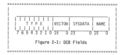
The DCB follows a strict format that defines the utilization of all four fields. The programmer need be concerned only with the TYPE and VECTOR fields. The system requires sole use of the SYSDATA field. It also maintains the NAME field thus usually necessitating no programmer intervention. The DCB format must be followed in all Device Control Blocks established by the user. The following information provides specifications for each field of the DCB.
