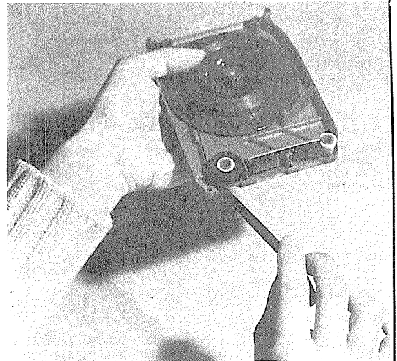
Excess tape is pulled gently from outside of the hub, letting hub and platter rotate freely. Note that end near center of hub has been cut fairly short to eliminate the possibility of tangling with the tape being removed.
