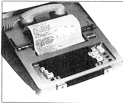
Figure 1. The PT-210 Portable Data Terminal weighs 15 pounds, prints quietly, and communicates with almost any modem-equipped computer.
