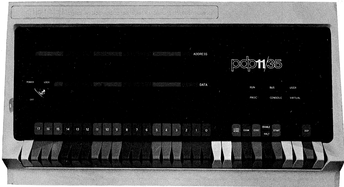
Figure 3-1b PDP-11/35 Programmer's Console
