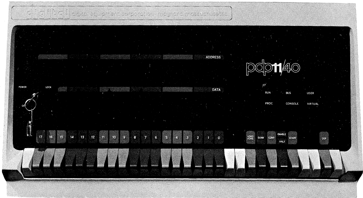
Figure 3-1a PDP-11/40 Programmer's Console
