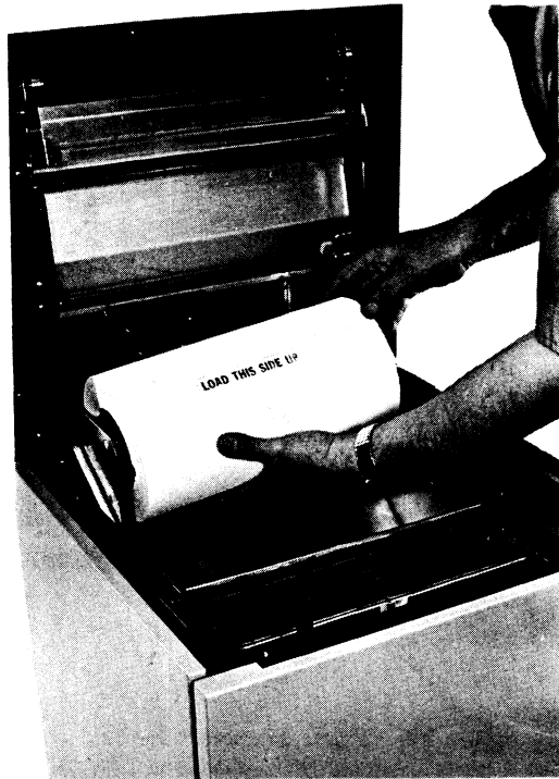
Figure 3-3 Inserting Roll Paper
