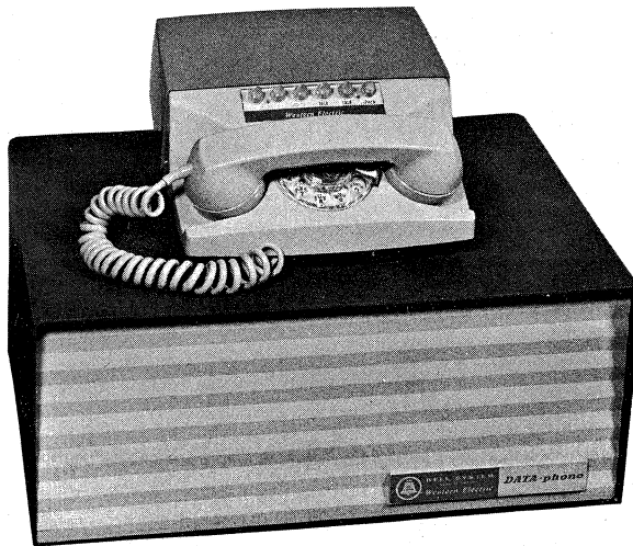
Figure I-1. Bell System 201A Modem with 804A Auxiliary Set
