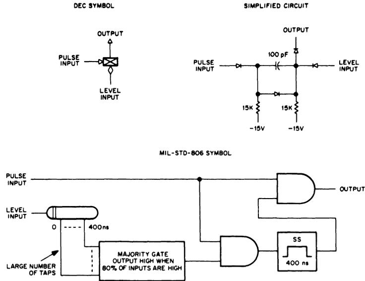
Figure 3-5 DCD Gate
