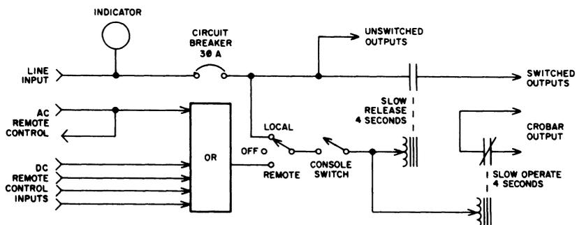
Figure 4-9 844 Power Control Block Diagram
