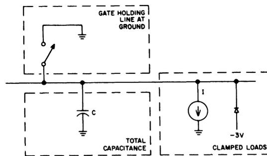
Figure 4-1 Circuit to Estimate Fall Time
