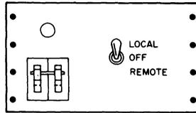
The 844 Power Control provides remote and local on-off control, noise filtering, and power-on, power-off logic transient control.
