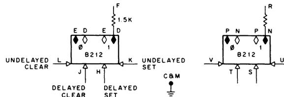
The B212 standard size FLIP CHIP module contains two clear-set flip-flops with buffered outputs and individual delayed and undelayed set and clear inputs.
