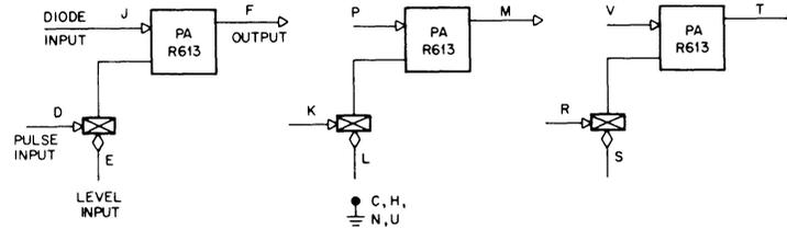
The R613 is pin compatible with and functionally similar to the R603.
