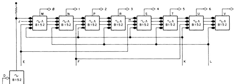
Figure 4-4 Internal Gating Structure, B152 Module
