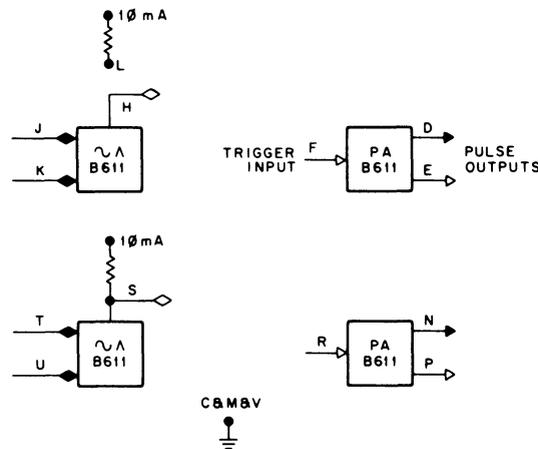
The B611 contains two independent 10 MHz 35 ns pulse amplifiers for power gain and pulse standardization. Two 2-input diode gates increase the logic flexibility.
