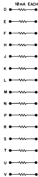
The W010 is pin compatible with the W002 and W005 clamped loads. It contains fifteen 10 mA clamped loads.
