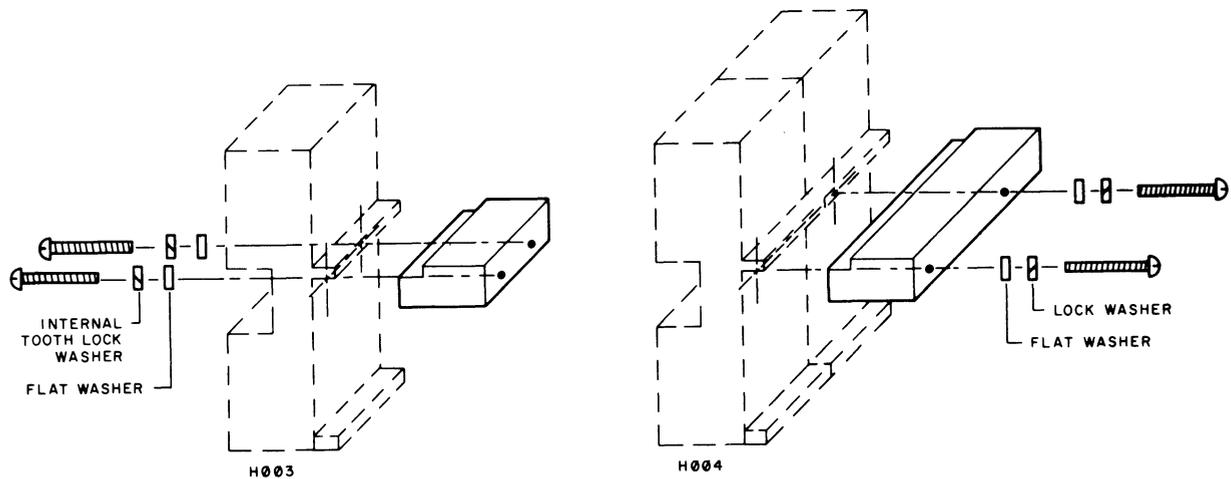
The H003 and H004 Connector Retaining Block kits are hardware kits which provide a connector retaining block to hold H350 series cable connectors and BC09A, BC10A and other compatible cable assemblies to H800 connector block (shown in phantom) such as are used in the H900 and 1943 mounting panels.
