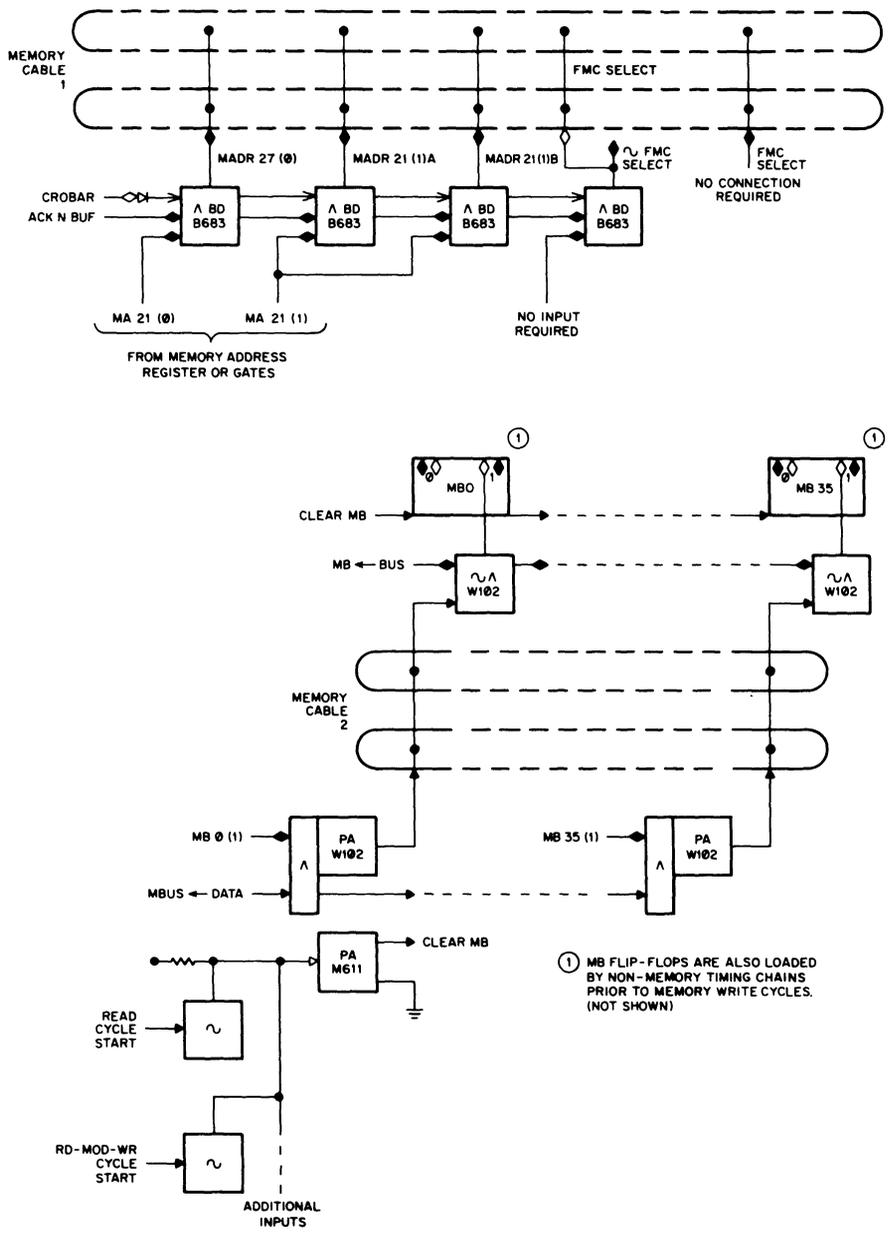
Figure 7-12 Memory Bus Address and Data Interface
