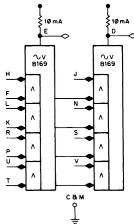
The B169 is a 2 mA diode gate used for performing AND/OR functions such as register input gating. The B169 will operate from standard DEC 35 ns or 40 ns negative pulses, provided that adequate fall times are maintained. It will also operate with standard DEC levels of ground and  $-3$  V. (Pulses 70 ns or wider are considered levels.) Repetition rate may be limited to less than 10 MHz by slow fall times.
