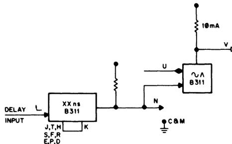
The B311 consists of a tapped delay line with suitable buffering and a connected 2 mA diode gate. Delay time is selected by connecting pin K to a delay line tap. (See delay control below.) This module has the same pin connections and can be used in the same slot as the B312 variable delay line module.
