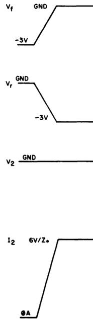
Figure A-3 Waveforms During Reflection
