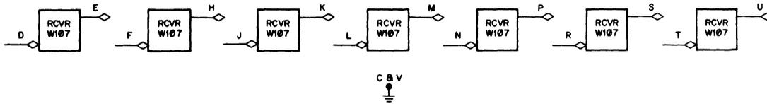
The W107 contains seven identical non-inverting receiver circuits with high-impedance input for buffering signals from the PDP-10 I/O Bus. The W107 is pin compatible with the W500 emitter follower.
