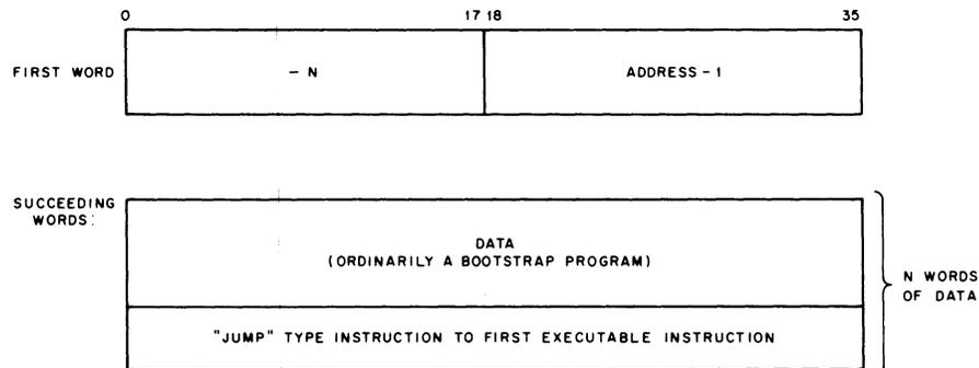
Figure 2-2 Read-In Mode Data Format
