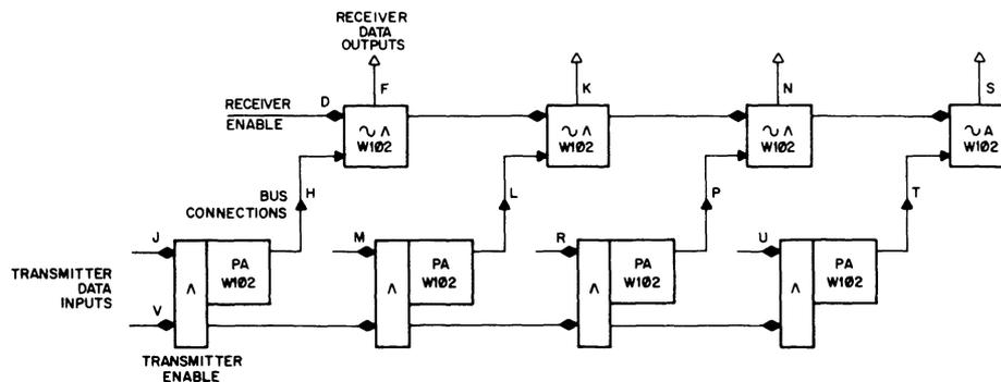
The W102 module is a pulsed bus transceiver capable of communicating with the PDP-1-D, PDP-6 and the PDP-10 memory bus system.
