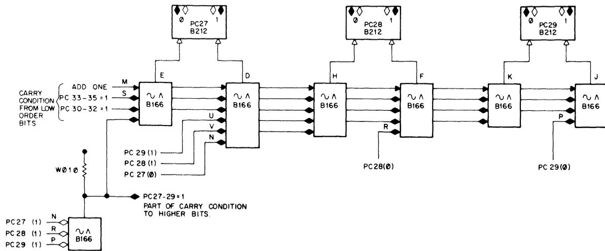
Figure 4-5 Up Counter Arrangement of B166 Module
