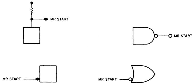
Figure 3-2 Sources and Loads Shown Without Connections
