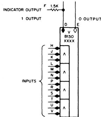
This special module has two levels of high speed logic and complementary outputs. It is designed to compute the parity (odd or even) of the contents of a flip-flop register with a minimum of delay, but it can be used wherever there is a need for four 3-input negative diode AND gates feeding a 4-input OR gate.
