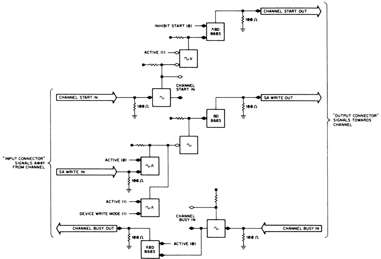
Figure 8-4 Channel Bus Synchronizing Logic
