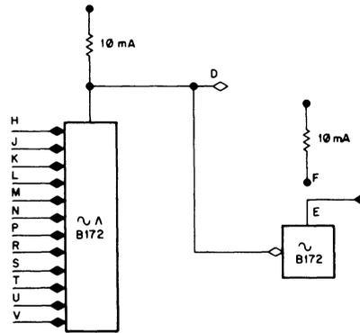
The B172 provides a 12-input 2 mA diode gate with 2 mA diode inverter permanently connected to the output of the first gate. It is often used for memory module selection on the PDP-10 memory bus.
