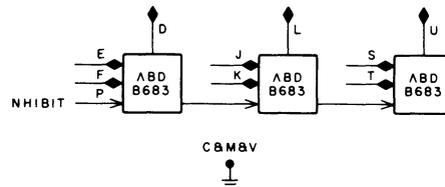
The B683 is the level counterpart of the W102 pulsed bus transceiver. It is designed to drive two 100  $\Omega$  transmission lines terminated to ground in their characteristic impedance. A single, terminated 50  $\Omega$  transmission can be driven instead. The output impedance of the B683 is zero when the output is low (-3 V) and infinite when high (ground) or when the power is off. Thus, two or more of these drivers may be attached to the same line in a "wired OR" fashion.
