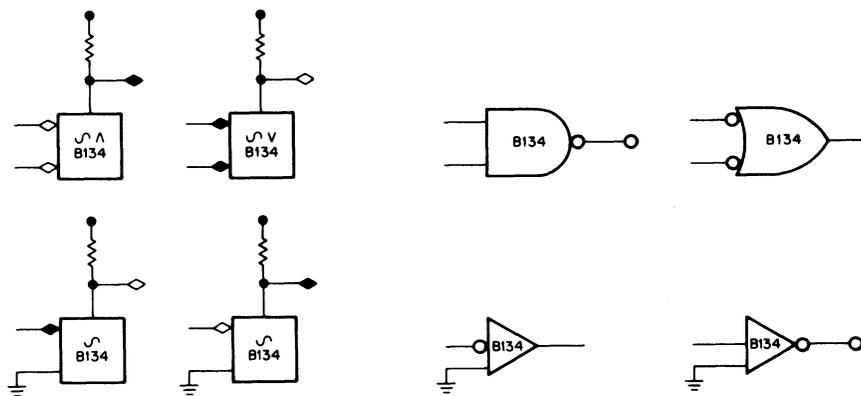
Figure 3-7 Different Uses of a Particular Module
