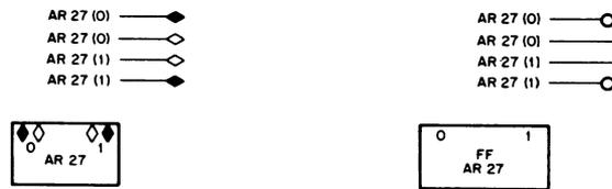
Figure 3-4 Flip-Flop Representation
