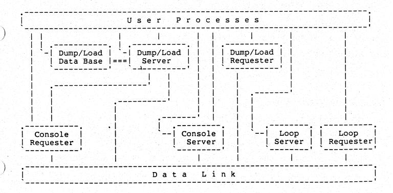
Requesters are the processes responsible for initiation of maintenance operations. This can be done either at higher level user request, or because of information obtained from a lower level. Requesters are the active side of a maintenance operation.
