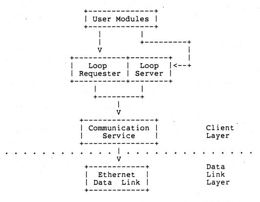
The active end of the loop testing communication link is the Loop Requester module. It contains features which establish and control the loop communications. Every Ethernet station must implement the Loop Server module. This module contains procedures which respond to Loop Requester inquiries and performs general communications service for remote Loop Requester modules for system tests and diagnostics.
