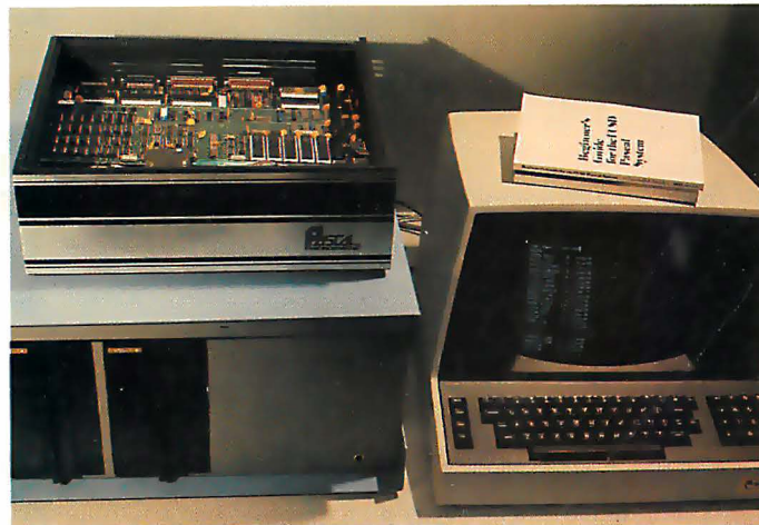
FIGURE 1: The Pascal Microengine is shown here in a system which includes two Shugart 8-inch disk drives in an Integrand cabinet and a Boroc IQ120 terminal. The computer uses a 16-bit processor chip and it executes p-code directly through the use of three integrated circuits on which the processor microinstructions are stored. The Microengine also includes 64 K bytes of memory, a 24-bit parallel port, and two RS-232C serial interfaces. The software provided is the UCSD extended Pascal system.
