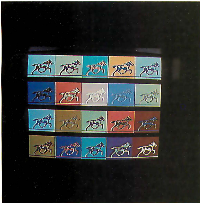
Photo 2: An example of the Apple III's high-resolution color graphics (290 by 192 lines of resolution with sixteen colors) displayed on an RGB (red, green, blue) color monitor. This particular demonstration is an animation program: the horses gallop on the screen.
