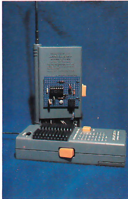
Photo 3: Two walkie-talkies can be used in a simple remote-control scheme. One walkie-talkie, used as the receiver, is modified by connection to the circuit illustrated in figure 10a. The new circuit is attached to the rear of the walkie-talkie's case, as shown. These walkie-talkies are sold by Radio Shack as catalog number 60-4001; they incorporate a Morse-code tone oscillator necessary to the control scheme. Transmission is on a frequency of 49.86 MHz.
