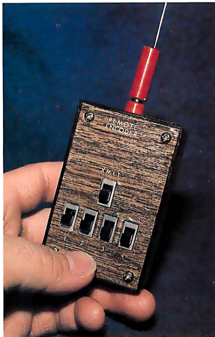
Photo 1: The handheld biphasic FSK remote-control transmitter, which uses the circuit shown in figure 3. The transmit (XMIT) switch is a momentary power switch; the other four switches are used to set a 4-bit control-channel code.
