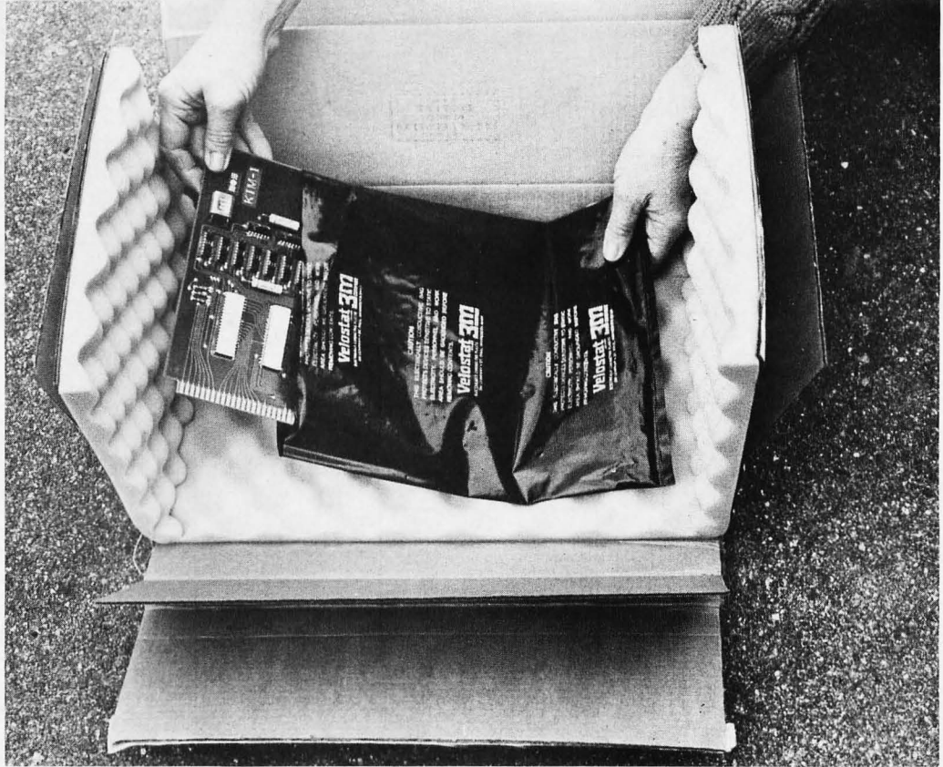
Photo 2: The KIM-1 processor as it is removed from its box. The MOS Technology product comes in a neat package which has one foam padded and static protected KIM-1 board as its bottom layer.
