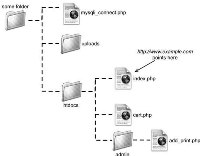
**Figure 17.8** The site structure for this Web application. The MySQL connection script and the `uploads` directory (where images will be stored) are not within the Web directory (they aren't available via `http://`).
