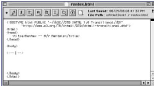
Figure 153-2: Comment tags inserted using the Utilities submenu
