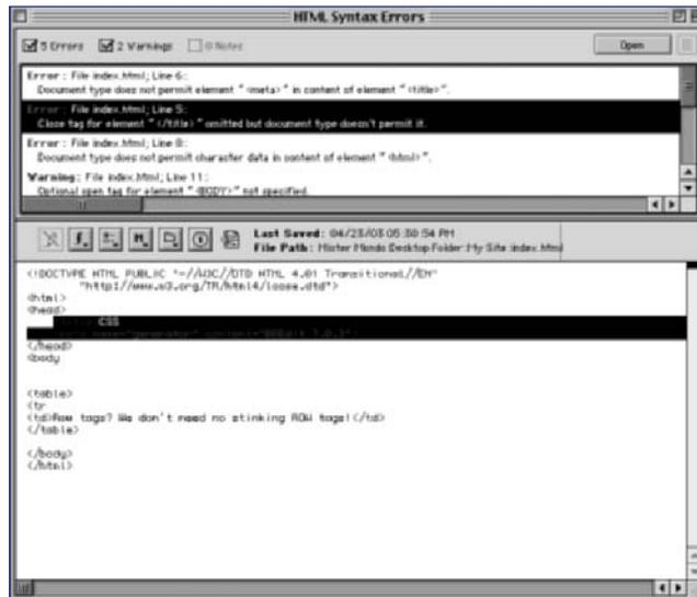
**Figure 152-1:** When BBEdit encounters errors, it displays the HTML Syntax Errors panel in the code window.
