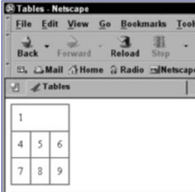
Figure 45-2: Cell 1 spanned across three columns
