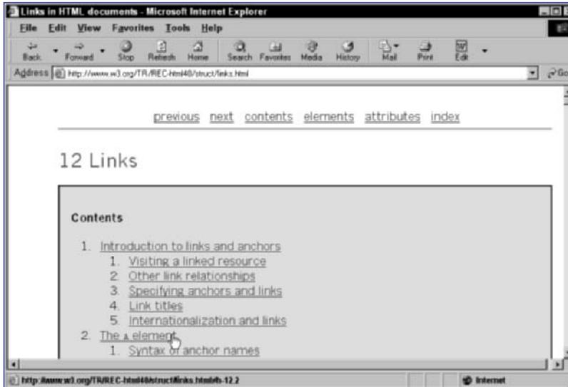
**Figure 42-1:** The Contents links at `www.w3.org/TR/REC-html40/struct/links.html` pointing to corresponding paragraphs further down the page (`links.html#h-12.2` in this case)
