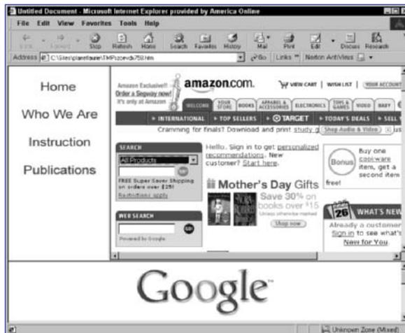
Figure 210-4: A frameset filled with original content (left) and links to other sites (right and bottom) that the browser fills within the frame borders
