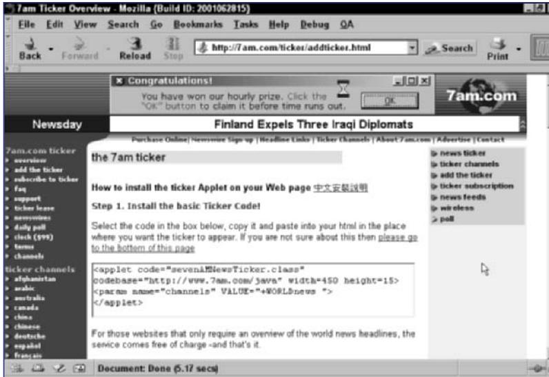
**Figure 111-2:** Getting the code for the 7 a.m. news ticker: the first field contains the applet code; the rest of the page describes the available parameters for the applet
