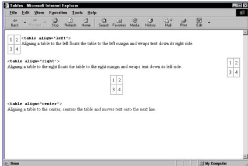
**Figure 46-1:** Three tables aligned around text: left, right, and center (from top to bottom)
