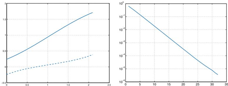
**Fig. 9.1.** At left: the two curves represent the two possible configurations of rods system in terms of the angle  $\alpha$  versus  $\beta \in [0, 2\pi/3]$  (Solution 2.9). At right: error versus iteration number of the Newton method for the computation of the zero of the function  $f(x) = x^3 - 3x^22^{-x} + 3x4^{-x} - 8^{-x}$  (Solution 2.11)
