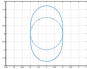
**Fig. 9.9.** Boundaries of the regions of absolute stability for the Heun method (*solid line*) and the forward Euler method (*dashed line*). The corresponding regions lie at the interior of the boundaries
