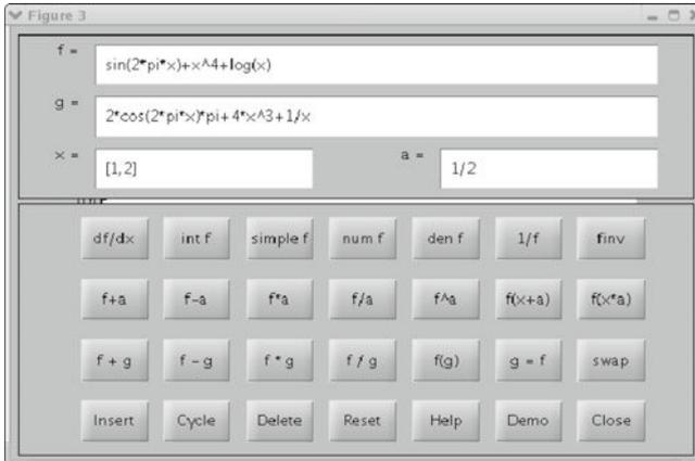
**Fig. 1.5.** Graphical interface of the command `funtool`
