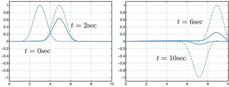
**Fig. 8.17.** Propagation of a pulse of voltage using the wave equation (*dashed line*) and the telegrapher's equation (*solid line*). At left, the thin solid line represents the initial condition  $u_0(x)$
