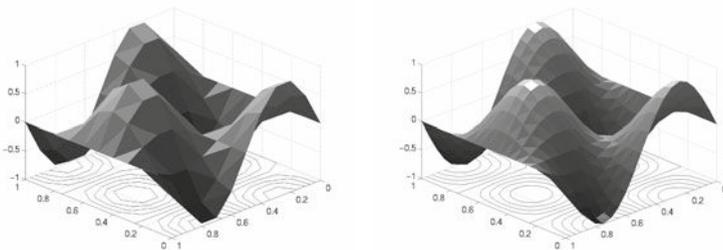
**Fig. 8.8.** Transverse displacement of an elastic membrane computed on two uniform grids, coarser at left and finer at right. On the horizontal plane we report the isolines of the numerical solution. The triangular partition of  $\Omega$  only serves the purpose of the visualization of the results
