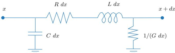
**Fig. 8.1.** An element of cable of length  $dx$
