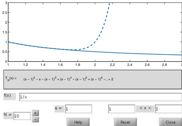
**Fig. 3.3.** Comparison between the function  $f(x) = 1/x$  (solid line) and its Taylor polynomial of degree 10 related to the point  $x_0 = 1$  (dashed line). The explicit form of the Taylor polynomial is also reported
