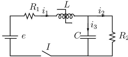
**Fig. 7.2.** The electrical circuit of Problem 7.4
