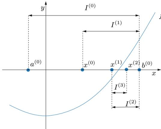
**Fig. 2.2.** A few iterations of the bisection method
