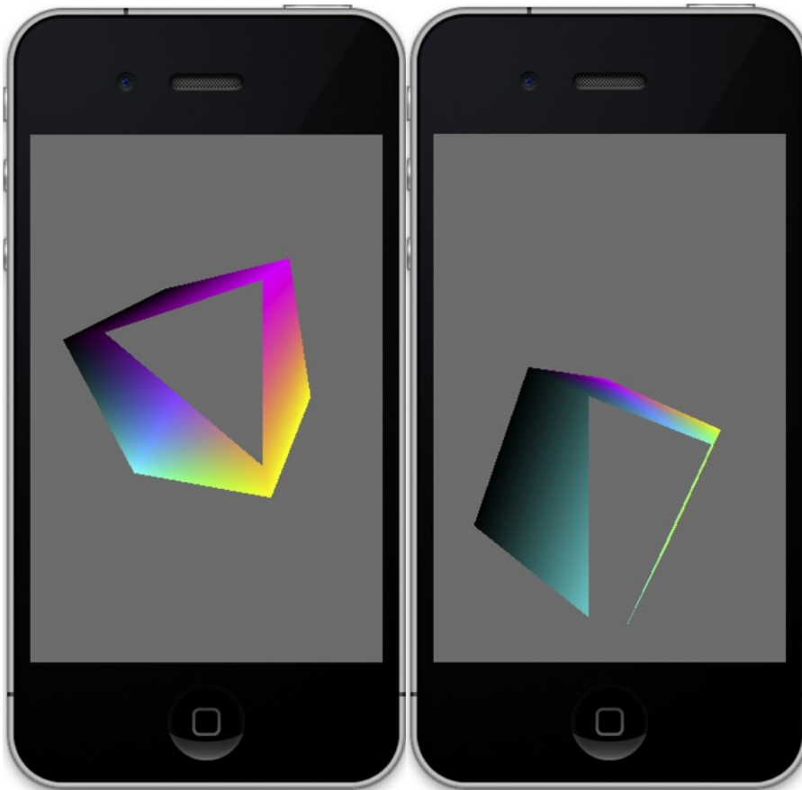
Figure 3-13. The zFar plane is reset, while the zNear plane is moved back to clip any part of the cube that is too close.
