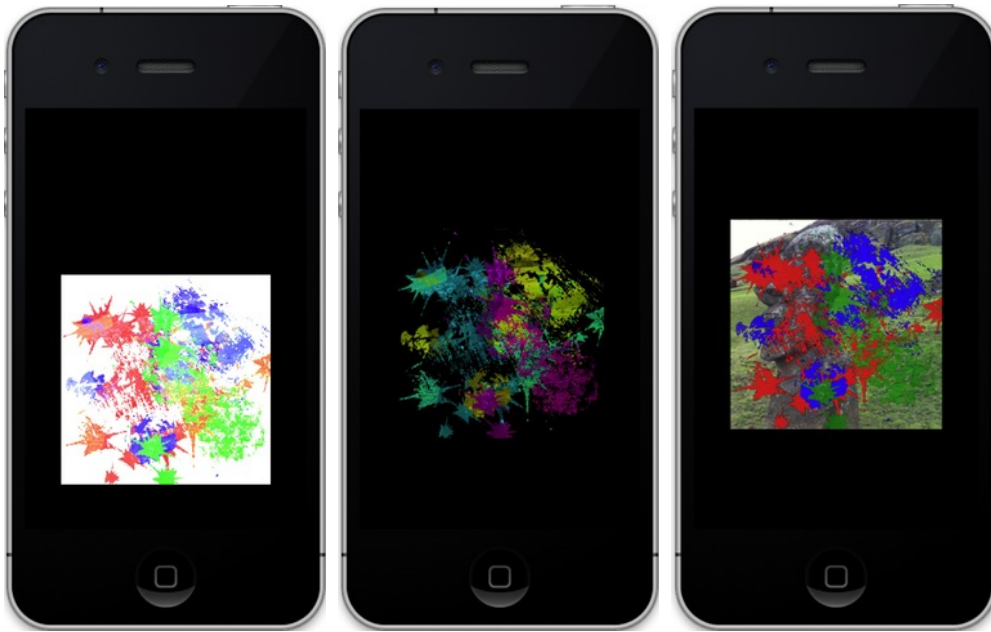
Figure 6-12. On the left, GL_ADD was used, GL_BLEND was added for the center, and GL_DECAL was added on the right.
