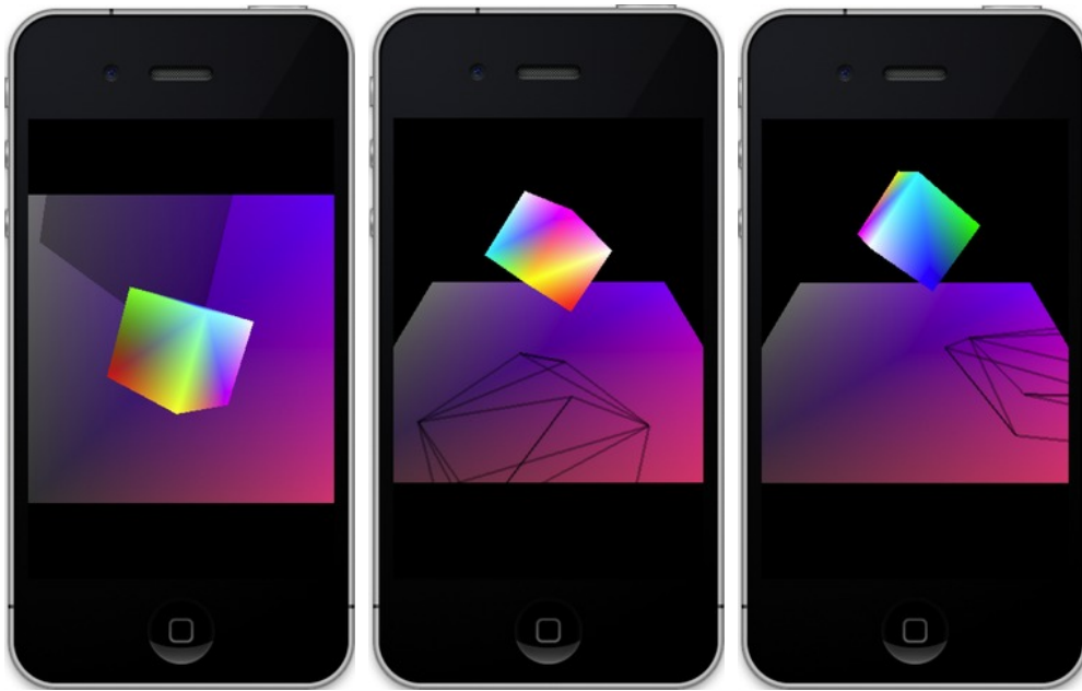
Figure 7-14. Showing the shadow in wireframe mode. The cube has been removed in the rightmost image to show the wireframe more clearly.
