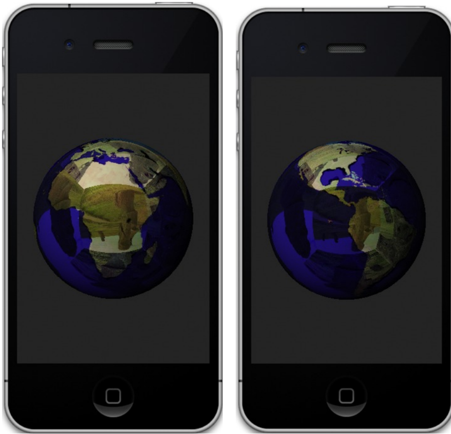
Figure 10-9. Reflection mapping the earth
