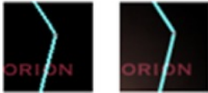
Figure 8-9. Multisample anti-aliasing, before (left) and after (right)
