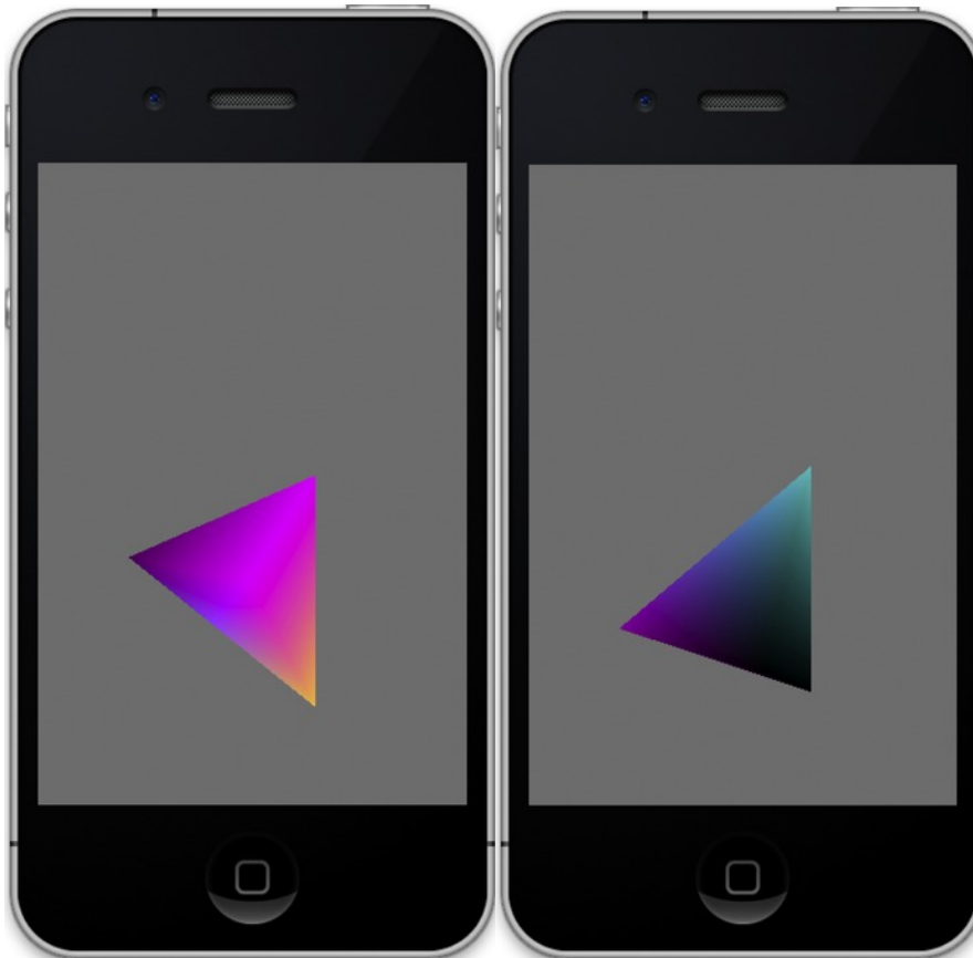
Figure 3-12. Peek-a-boo! The cube is clipped when any part of it is farther away than zFar.
