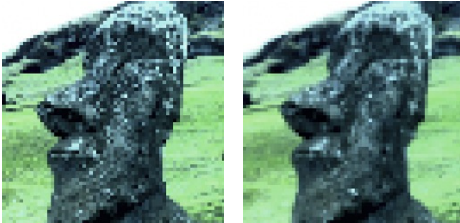
Figure 5-20. All filtering turned off (left), bilinear filtering turned on (right)
