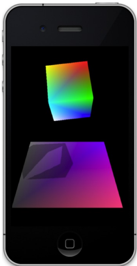
Figure 7-12. Z-fighting between the platform and the shadow
