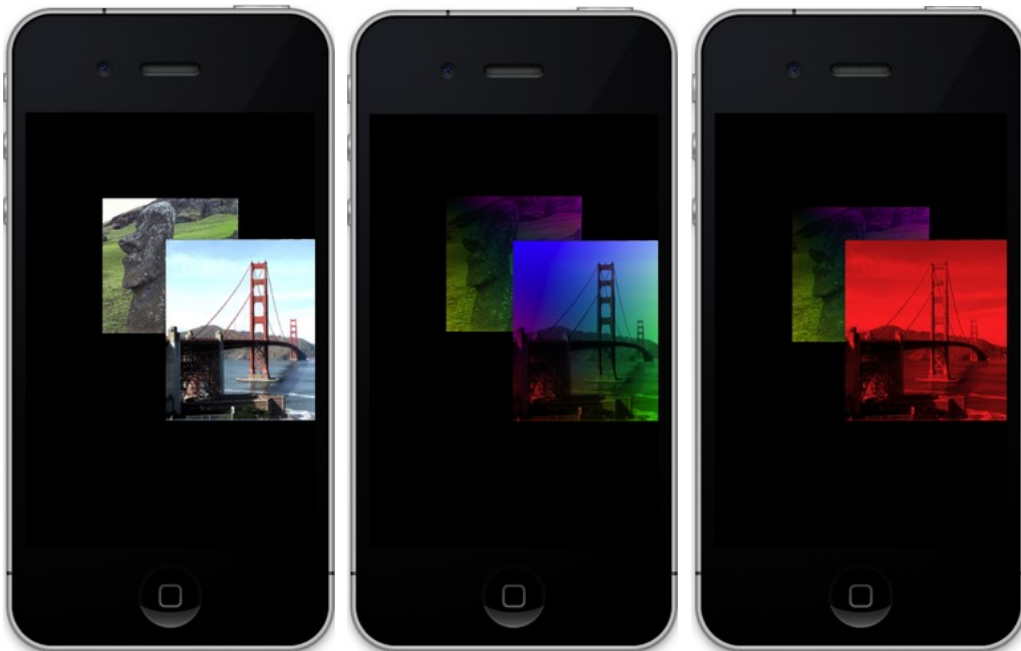
Figure 6-8. On the left, only the textures are displayed. In the center, they're blended with color, and for the one on the right they're solid red.
