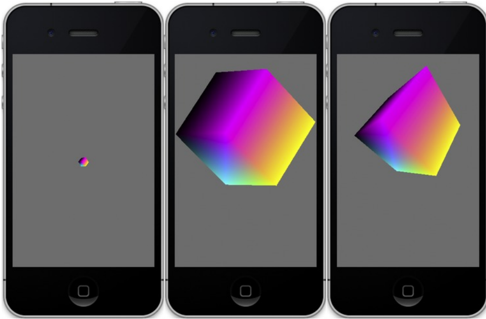
Figure 3-14a,b,c. Moving the object away (left) and then zooming in on it (center). The rightmost image has the default FOV value set to 60 degrees with the cube at only 2 units away.
