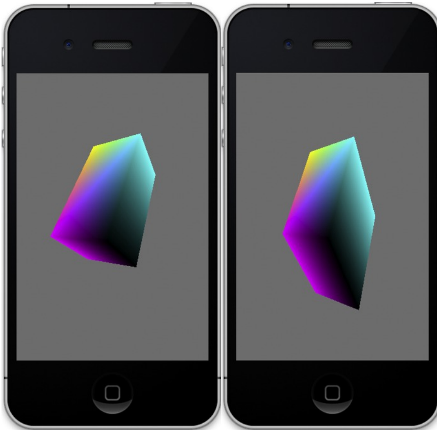
Figure 3-11. Scaling before the rotations have been executed (left) and scaling after the rotations (right)
