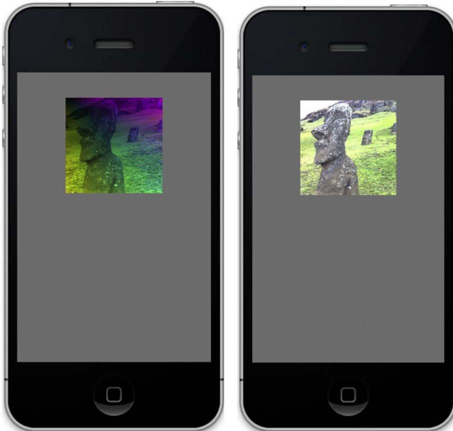
Figure 5-13. Applying texture to the bouncy square. Using vertex colors (left) and not (right).
