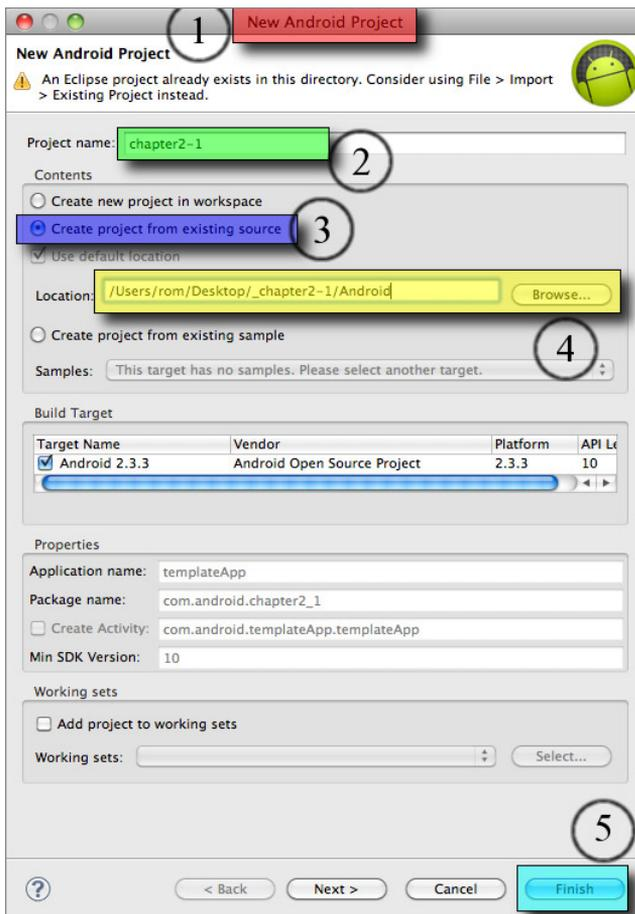
**FIGURE 1-4:** Importing an Android project into Eclipse
