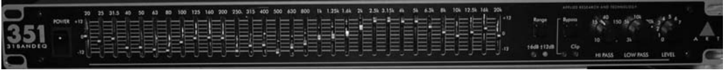
Figure 11.2: Photograph of an Applied Research and Technology, Inc. 31-band, 1/3 octave, ISO spaced, monaural graphic equalizer.
