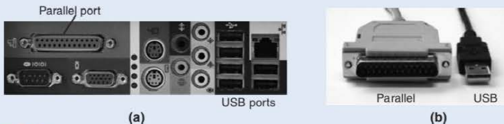
Figure 4.20 Parallel versus serial communication in desktop computers: (a) a PC having a parallel port and six serial USB ports, (b) parallel and USB plugs/cables.
