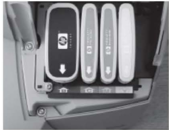
Figure 4.48 A color printer mixes cyan, magenta, and yellow inks to create any color. The picture shows inside a color printer having those three colors' cartridges on the right, labeled C, M, and Y. Such printers may use black ink directly (the big cartridge on the left), rather than mixing the three colors, to make grays and blacks, in order to create a better-looking black and to conserve the more expensive color inks.
