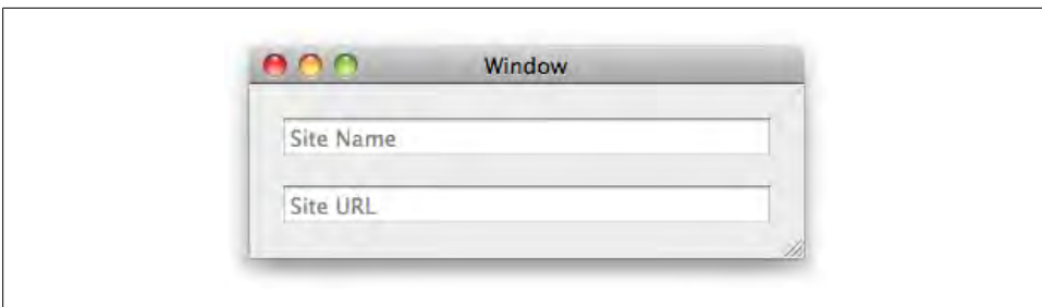
Figure 8-28. Placeholder text indicates the purpose of a text field to the user
