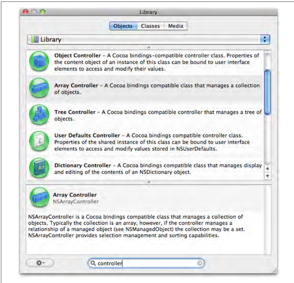
Figure 8-44. The classes that inherit from NSController
