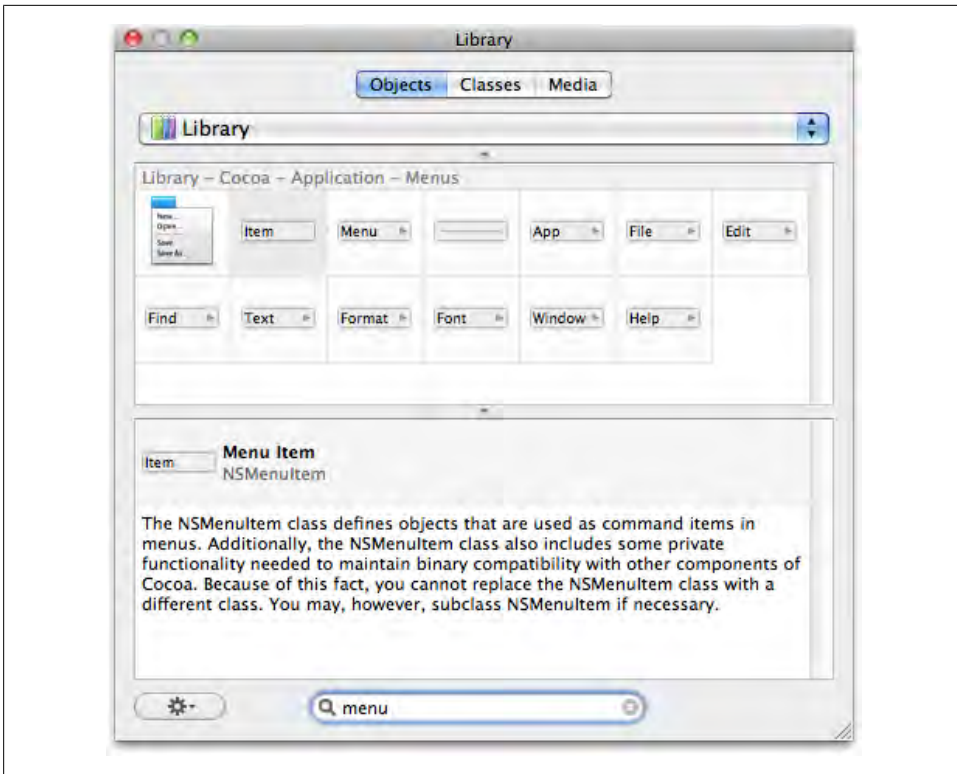
Figure 8-16. You can drag menus and menu items from the Library window into the menu bar
