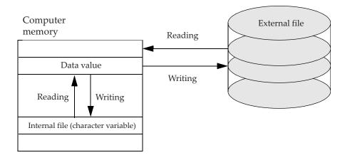
**Figure 9-5** External and internal files
