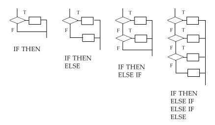
**Figure 8-1** Execution flow for IF constructs.
