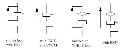
**Figure 8-4** Execution flow for DO constructs
