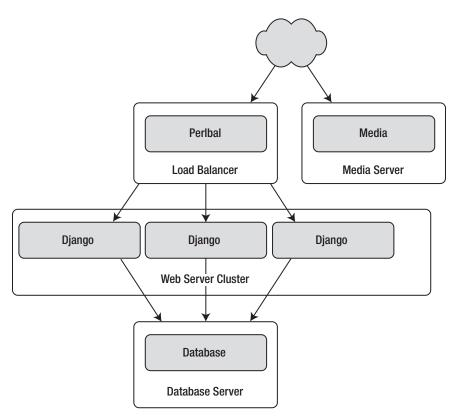
Figure 12-4. A load-balanced, redundant server setup
