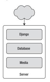
Figure 12-1. A single-server Django setup
