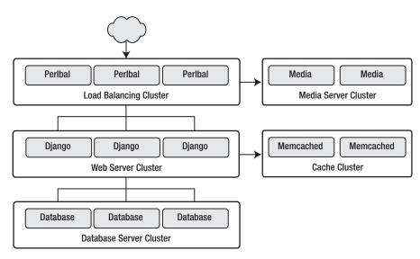
Figure 12-5. An example large-scale Django setup
