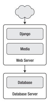
Figure 12-2. Moving the database onto a dedicated server
