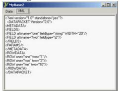
Figure 13.2: The XML display of a CDS file in the MyBase2 example. The table structure is defined by the program, which creates a file for the dataset on its first execution.
