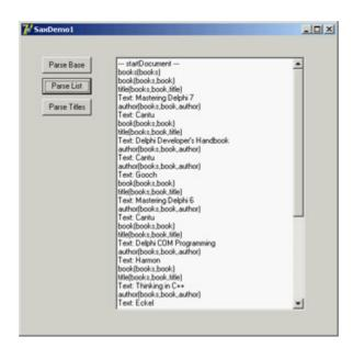
Figure 22.6: The log produced by reading an XML document with the SAX in the Sax-Demo1 example
