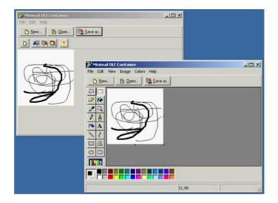
Figure 12.6: The second toolbar of the OleCont example (above) is replaced by the server's toolbar (below). Tip
