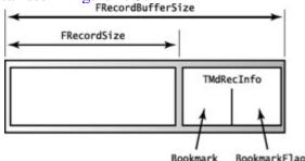
Figure 17.5: The structure of each buffer of the custom dataset, along with the various local fields referring to its subportions
