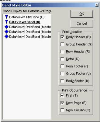
This editor provides a simple method to select the features you want for a Band by using the check boxes. Note that a Band can have several different features active at a time. This means it is possible for a Band to be both a Body Header and Body Footer simultaneously.
