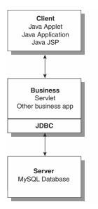
Figure 2.2 A three-tier deployment model.
