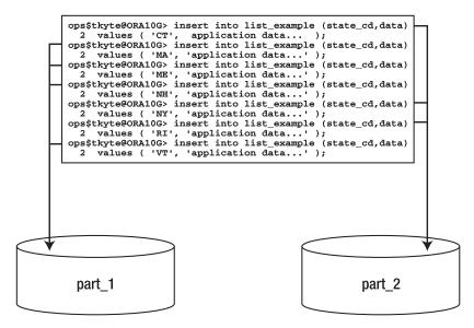
Figure 13-3. List partition insert example
