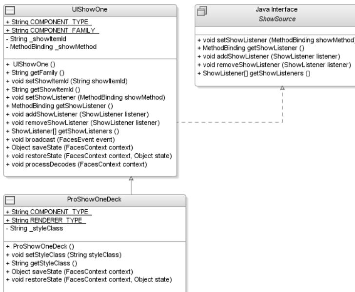
Figure 3-8. Class diagram showing the `UIShowOne` implementation
