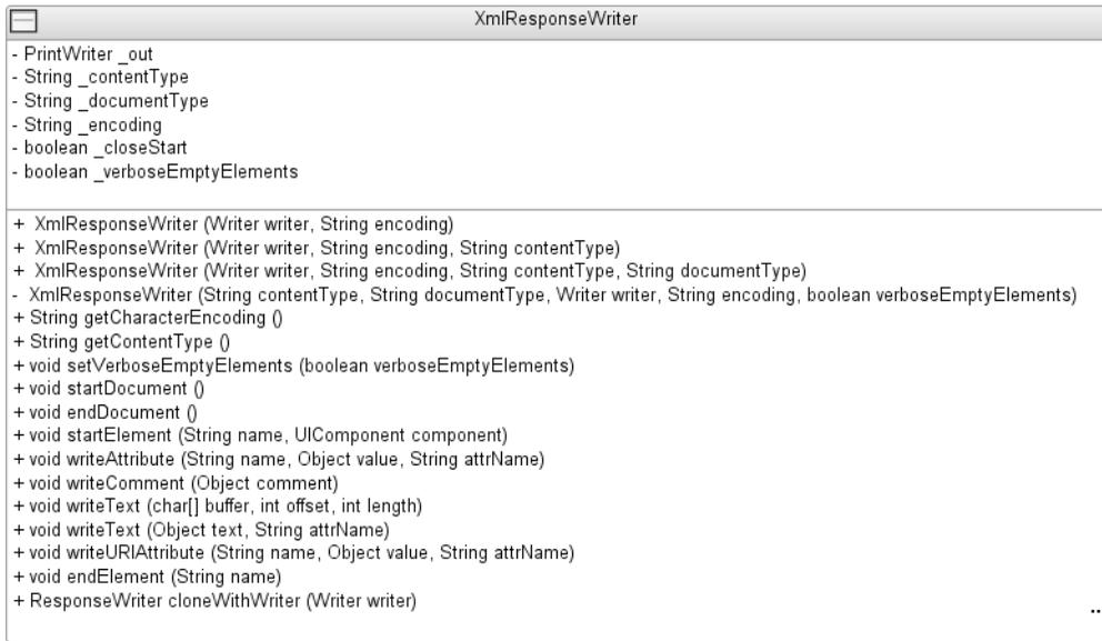
**Figure 8-15.** Class diagram showing the XMLResponseWriter class
