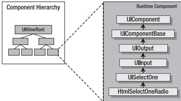
**Figure 1-7.** `UIComponent` inheritance
