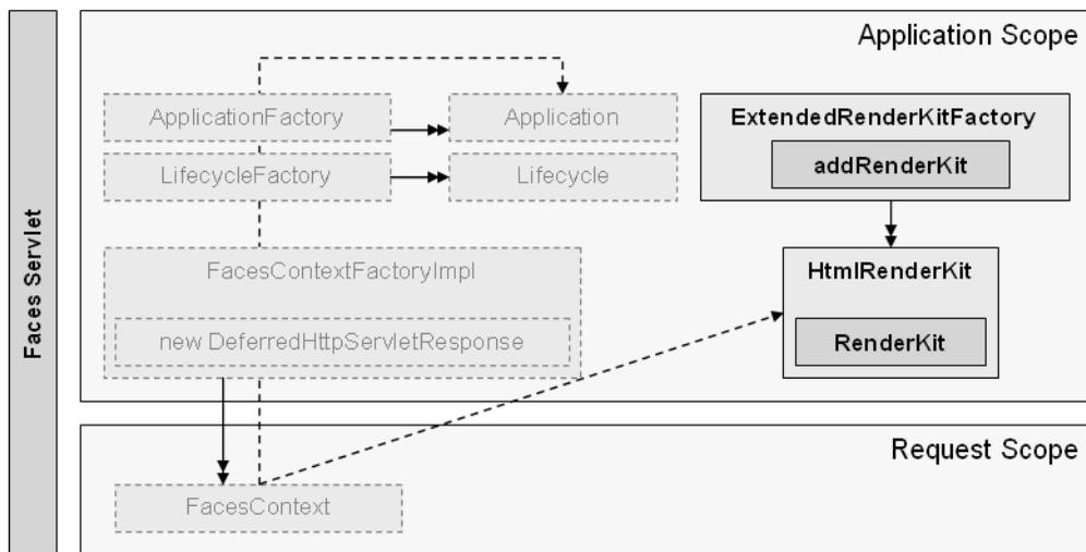
**Figure 6-6.** *Extending the RenderKitFactory and wrapping the standard HTML RenderKit*
