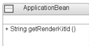
**Figure 10-2.** *Class diagram showing the `ApplicationBean` class*
