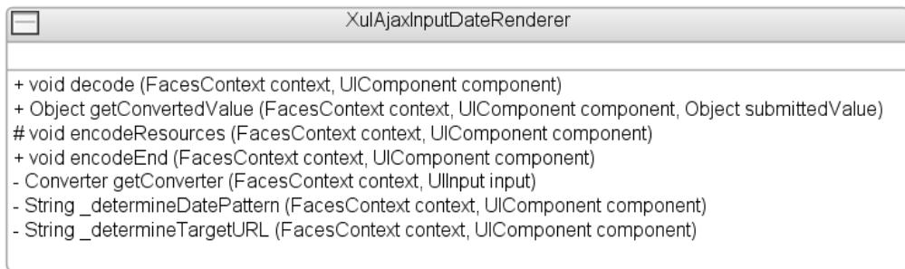
**Figure 8-9.** Class diagram showing the `XulAjaxInputDateRenderer` class
