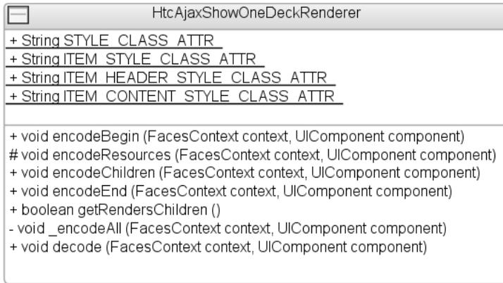
**Figure 9-10.** Class diagram showing the `HtcAjaxShowOneDeckRenderer` class
