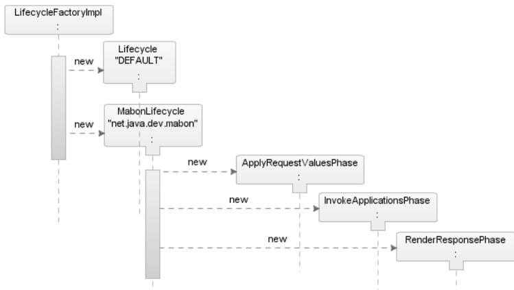
**Figure 7-7.** Sequence diagram of Mabon at application start-up
