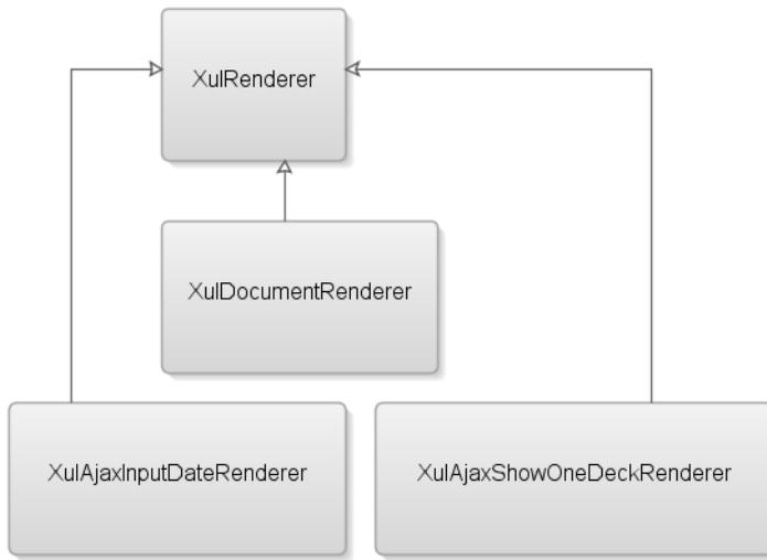
**Figure 8-7.** Class diagram showing the XUL Renderers
