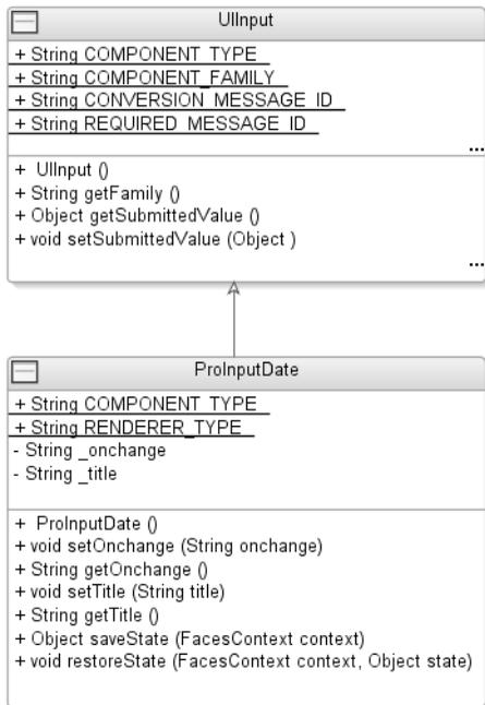
**Figure 2-10.** Class diagram over the `ProInputDate` renderer-specific subclass
