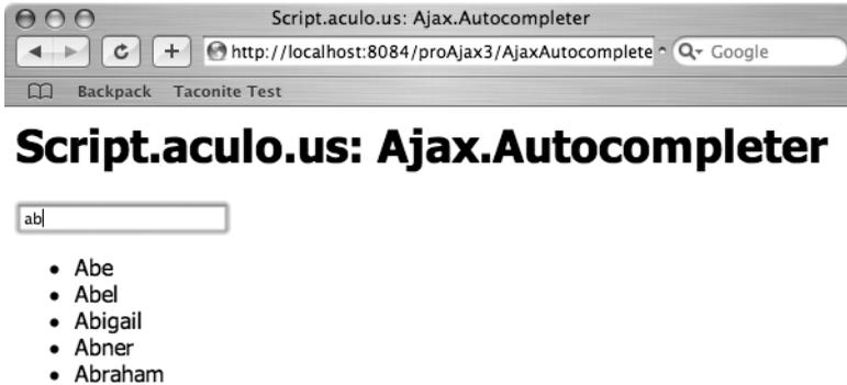
**Figure 3-14.** *The basic Ajax.Autocompleter*
