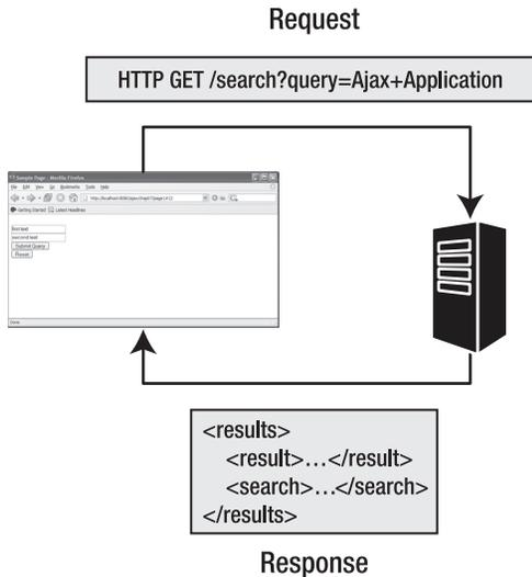
**Figure 11-5.** HTTP communication for a synchronous interface
