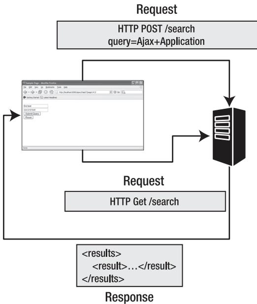
**Figure 11-6.** *HTTP communications for an asynchronous interface*
