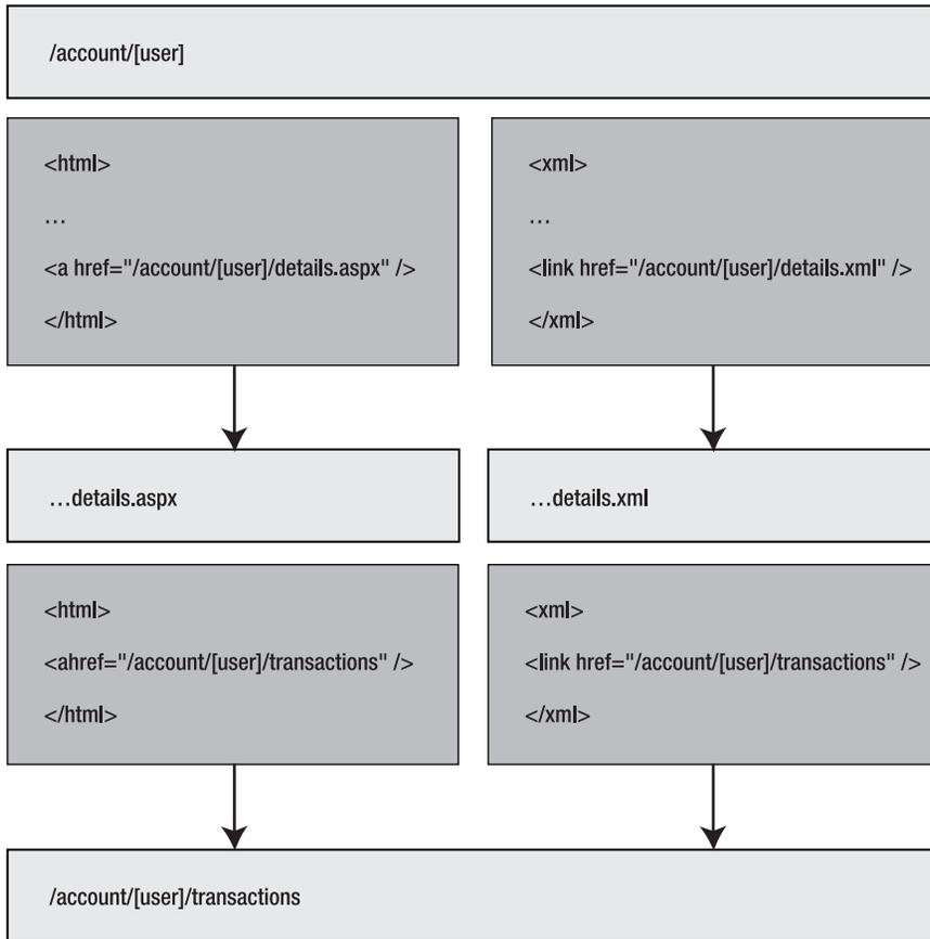
**Figure 5-7.** *Rearchitected application using the Permutations pattern*
