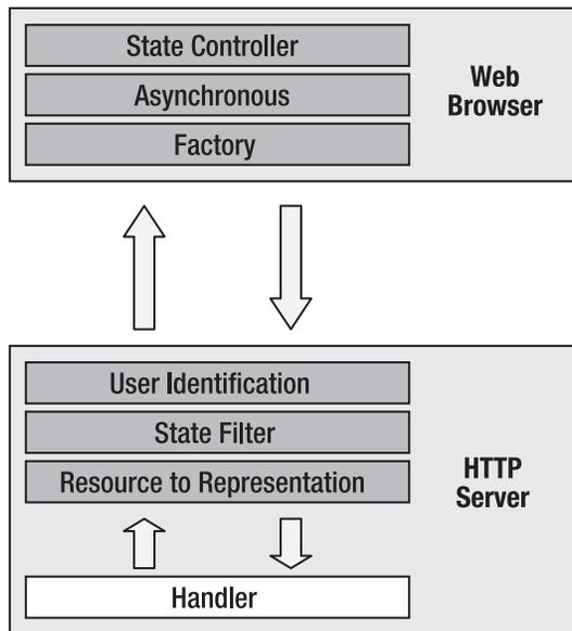
**Figure 9-12.** Layered architecture of the State Navigation pattern
