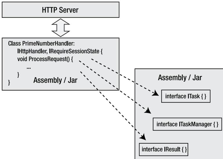
**Figure 10-3.** *Packaging structure of handler and interface implementations*
