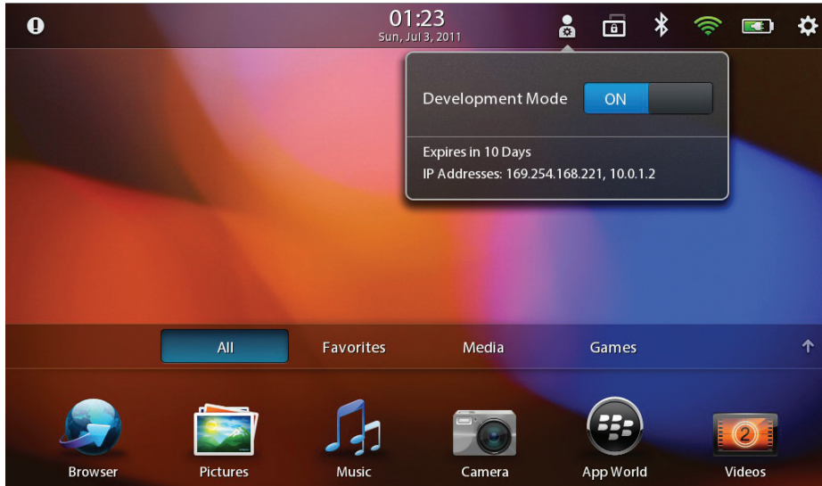
FIGURE 2-25: IP Address displayed when the Development mode is enabled and BlackBerry PlayBook is connected
