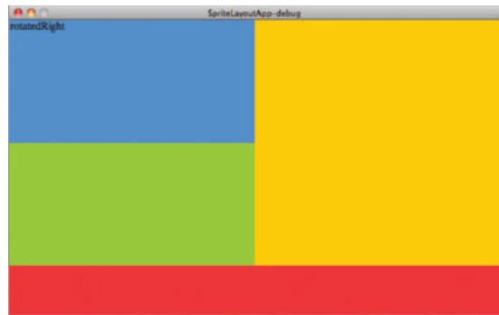
FIGURE 5-9: The deviceOrientation property being displayed in the landscape layout design for Sprite Layout App
