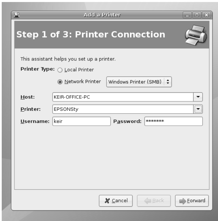
Figure 8-10. Ubuntu should be able to automatically detect any Windows or SMB shared printers on your network.
