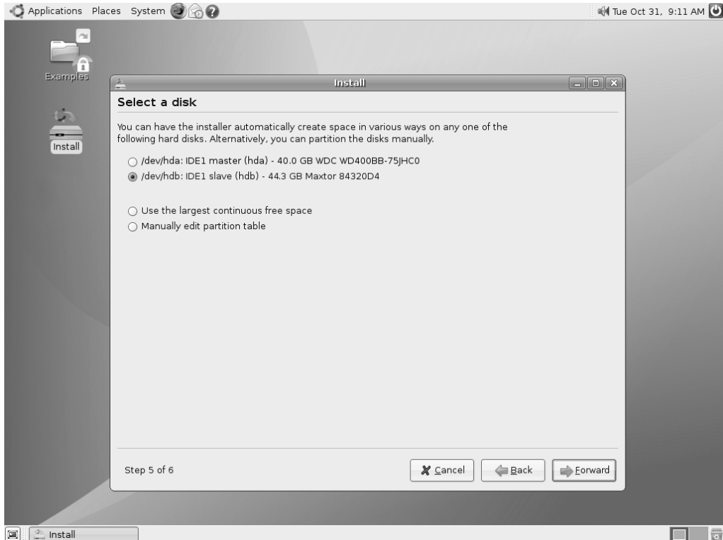
Figure 5-10. If there's more than one hard disk installed, you'll be prompted to choose between them when the partitioning tool starts.
