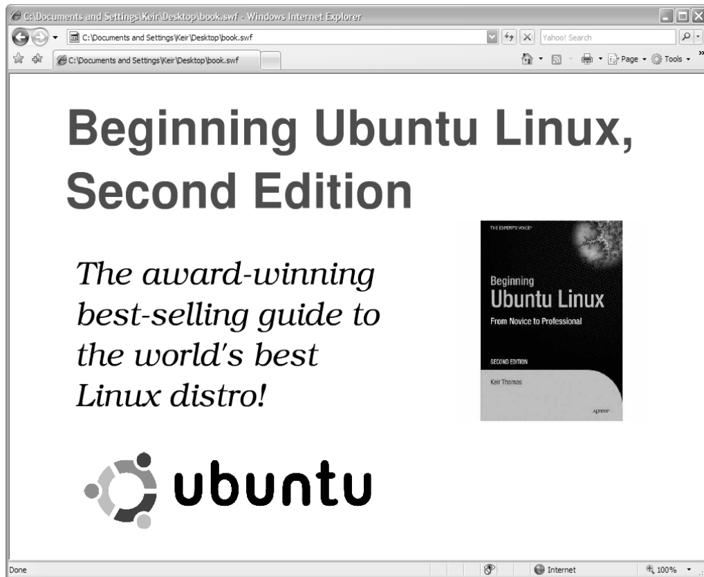
Figure 25-6. You can save any presentation as a Flash animation, which can be played back in a suitably equipped web browser.
