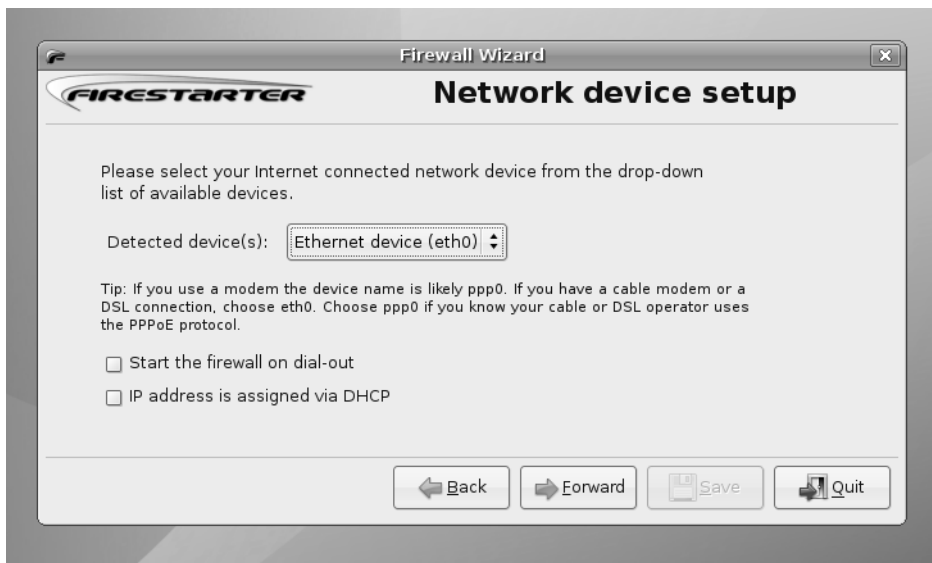
Figure 9-4. Firestarter includes a wizard to walk you through the basics of firewall configuration.
