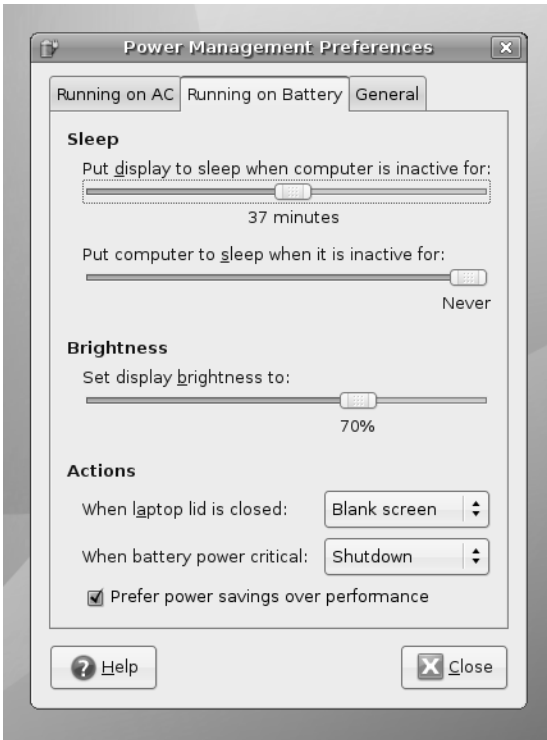
Figure 8-8. Notebook users can define an additional power profile that will kick in when the battery is in use.
