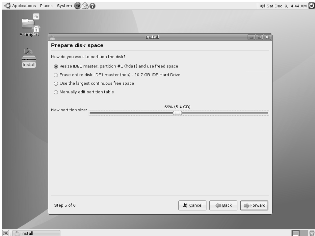
Figure 5-9. You can resize the existing partition on the hard disk by clicking and dragging the New Partition Size slider.
