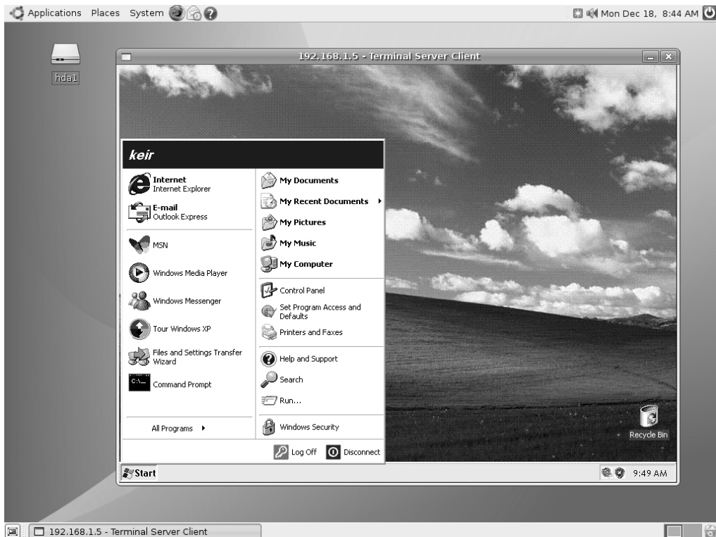
Figure 33-4. You can access remote Windows XP Professional machines using RDP and the Terminal Server Client program.
