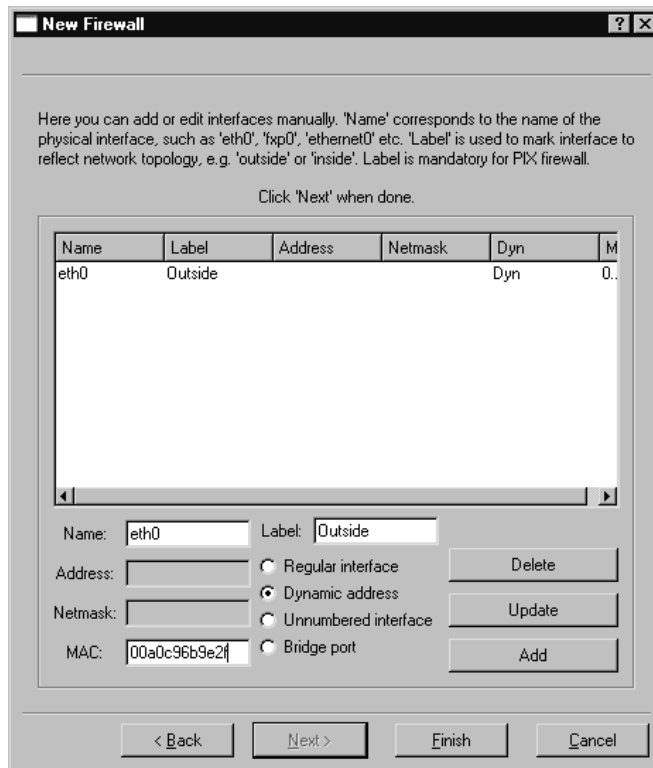
Figure 9.21 FWBuilder Manual Interface Configuration
