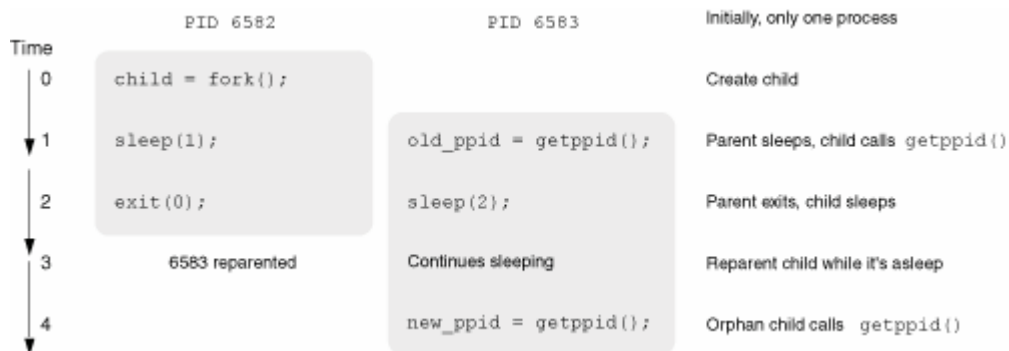
Figure 9.2. Two processes running in parallel after forking
