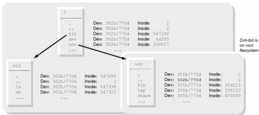
Figure 8.2. Separate filesystems, after mounting
