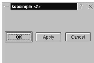
Figure 4-3: The default buttons of a KDialogBase window
