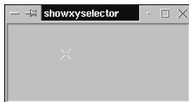
Figure 19-55: The KXYSelector widget with its cross hairs position indicator
