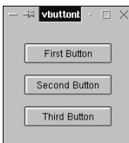
Figure 7-3: A KButtonBox with vertical orientation
