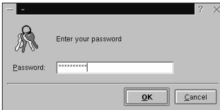
Figure 19-40: A KPasswordDialog widget with an obscured password entered
