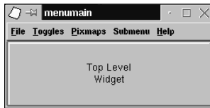
Figure 6-4: An application with a menu bar at the top
