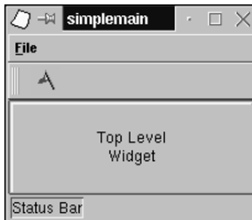
Figure 6-1: Using a KTMainWindow to create and control the main window of an application
