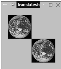
Figure 13-10: Positioning pixmaps from a new origin
