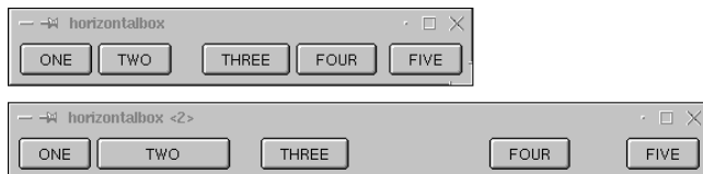
Figure 3-9: A horizontal box before and after being stretched horizontally
