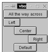
Figure 3-10: A fixed-size widget aligns left, right, or center.
