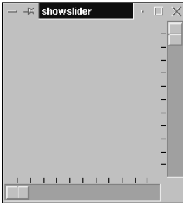
Figure 18-19: One horizontal and one vertical QSlider
