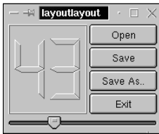
Figure 3-11: A QVBoxLayout inside a QGridLayout
