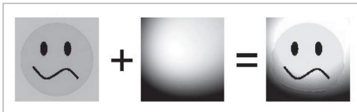
Figure 2-46: With hardware, we draw the polygon in a first pass with texture but without light map applied (left). In this first pass, the texture may be tiled. In a second pass, we apply a light map (middle) to the existing textured pixels (right). The light map is not tiled.
