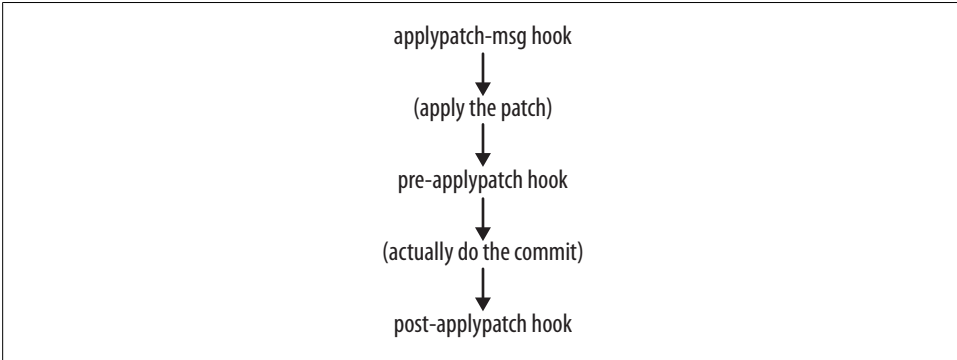
Figure 14-2. Patch hook processing
